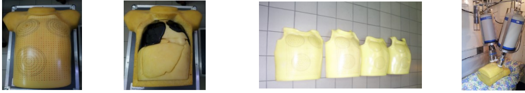
FIG. 3. LLNL realistic torso phantom, different chest plates and measurement geometry
