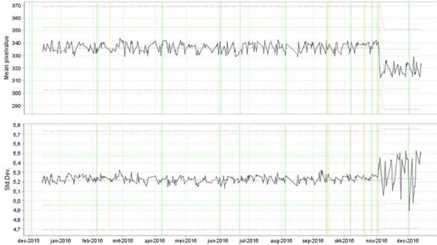
FIG. 17. Run charts of mean pixel value and standard deviation indicating an incident that needs to be further investigated (courtesy of J. Binst, UZ Leuven).
