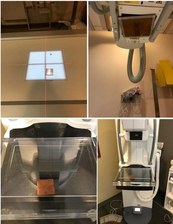
*FIG. 33. Photos of the radiography (top) and mammography (bottom) phantoms, positioned with respect to the light field. For the radiography phantom, note the use of the absorber, positioned at the collimator exit (top right).*
