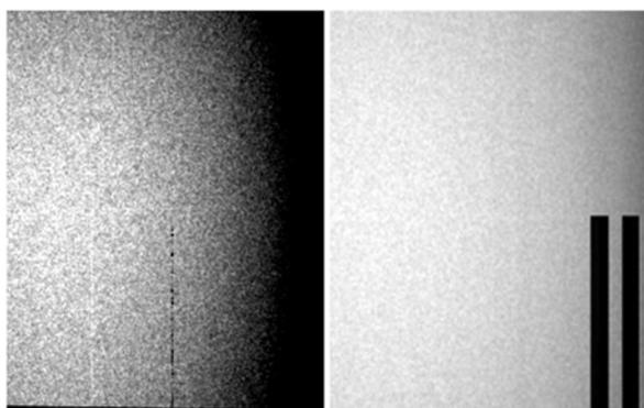
*FIG. 24. Example of the appearance of dead columns in digital detectors, single (left) and multiple (right) (courtesy of K. Lemmens, Leuven).*
