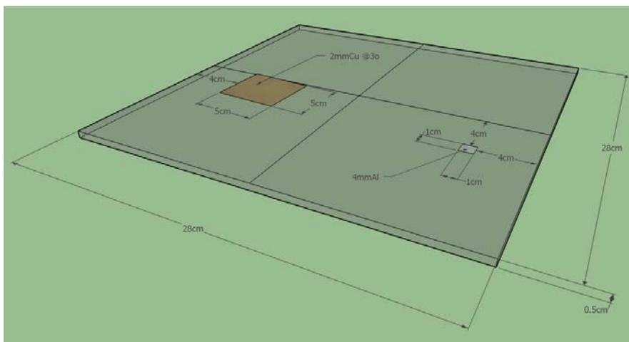
FIG. 14. Dimensions of the target plate for a radiography phantom. An additional attenuator of 2 mm Cu is required for proper use.
