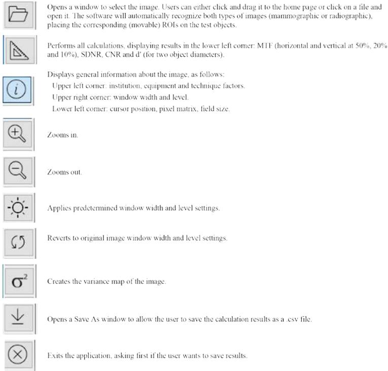
FIG. 5. Automated tool for image analysis (ATIA) application icons. CNR — contrast to noise ratio, MTF — modulation transfer function; ROI — region of interest, SDNR — signal difference to noise ratio.
