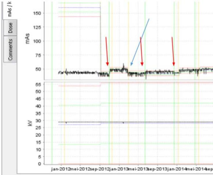
FIG. 18. Run charts of the mA-s used for standard phantom exposure, indicating several changes in the system performance (courtesy of J. Binst, UZ Leuven).
