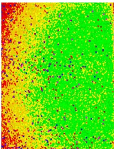
*FIG. 28. A poorly maintained computed radiography plate created this variance map, as produced by the automated tool for image analysis (ATIA).*
