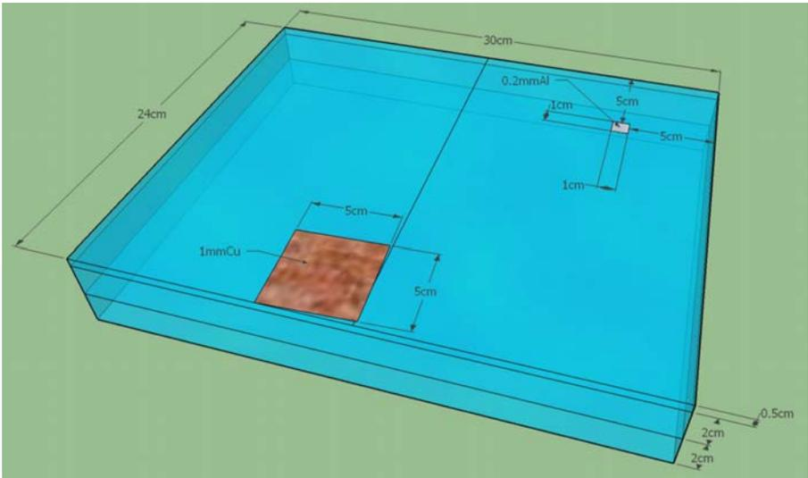
FIG. 15. Dimensions of the mammography phantom and attenuator.
