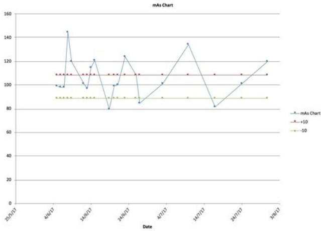
FIG. 36. Control chart of the mAs results for one mammography unit demonstrating wide fluctuations, due to inconsistent positioning of the phantom affecting the automatic exposure control.
