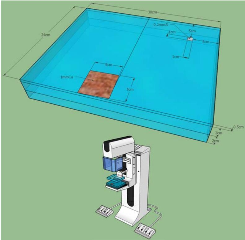
FIG. 3. Mammography phantom (top) and set-up (bottom).
