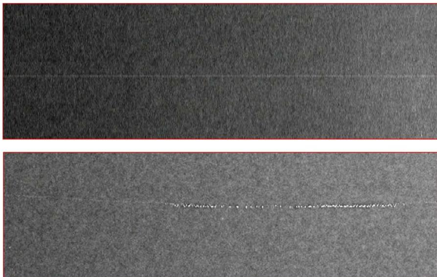
FIG. 29. Examples of computed radiography errors in the reading element (top) or due to a scratch (bottom).
