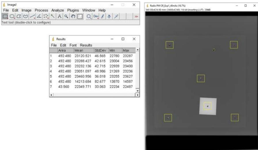
FIG. 12. Screenshot of grey level and noise measurements with ImageJ and corresponding results for region of interest (ROI) measurements.
