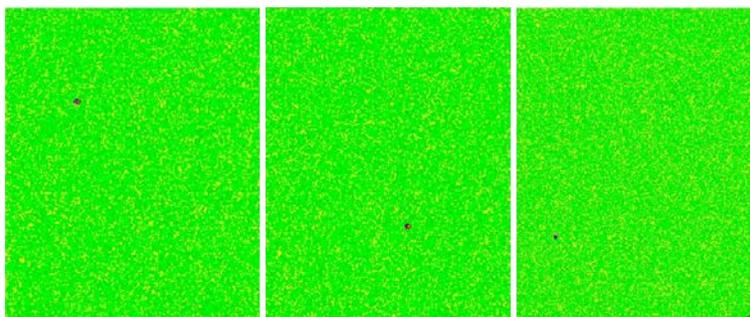
FIG. 20. Example of the appearance of dust in the bucky tray on three consecutive images of a uniformity phantom. Note that the artefact rotates together with the phantom.
