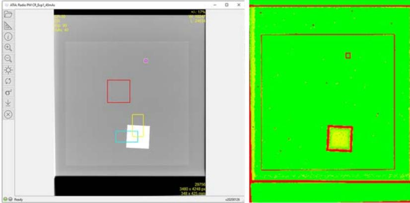
FIG. 6. A radiography phantom image loaded into the automated tool for image analysis (ATIA) (left) and the corresponding variance map (right) produced by the ATIA.
