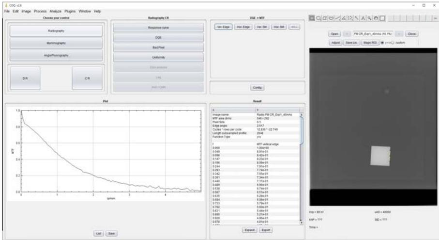
FIG. 13. Screenshot of the modulation transfer function (MTF) measurement with COQ (ImageJ plug-in) and corresponding results from COQ [33].
