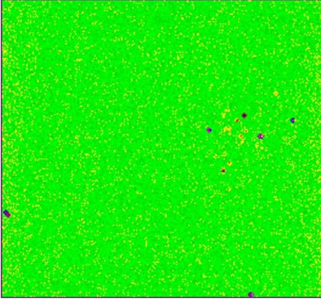
FIG. 21. Example of an image with dust or debris particles, as they appear in the variance image.
