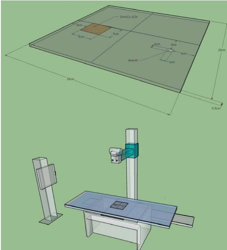
FIG. 2. Radiography phantom (top) and set-up (bottom).
