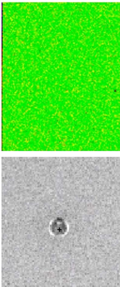
*FIG. 23. Examples of dead pixels on a digital detector. Dead pixels can show up as a signal void (top) or in the shape of a bull's eye (bottom).*
