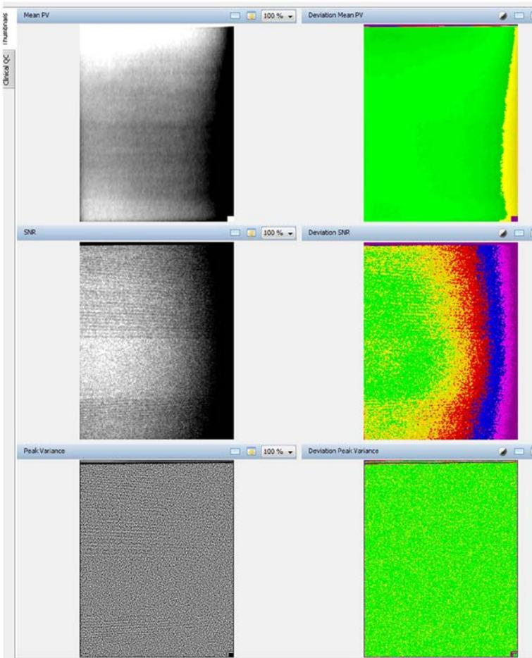
FIG. 25. These images demonstrate the effect of grid problems on mean pixel values (top row), the signal to noise ratio (SNR) (centre row) and the peak variance (bottom row).
