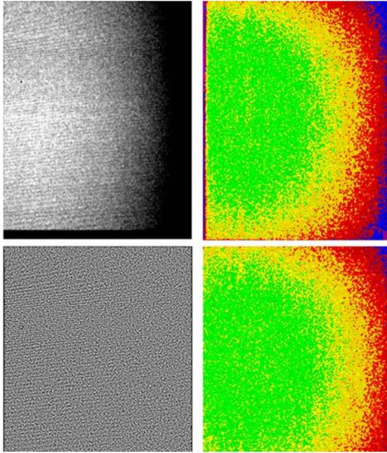
FIG. 26. Image demonstrating a grid misalignment, as shown in the image and in the variance map, before (top row) and after (bottom row) service (courtesy of K. Lemmens, Leuven).
