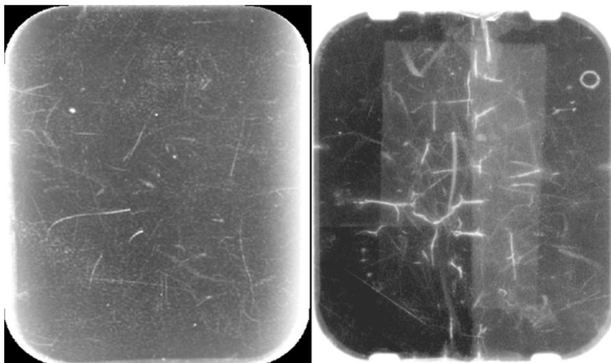
*FIG. 30. Artefacts attributed to the age and poor maintenance of computed radiography plates resulting in a permanent ghost image (right) (courtesy of A. Jacobs, Leuven).*
