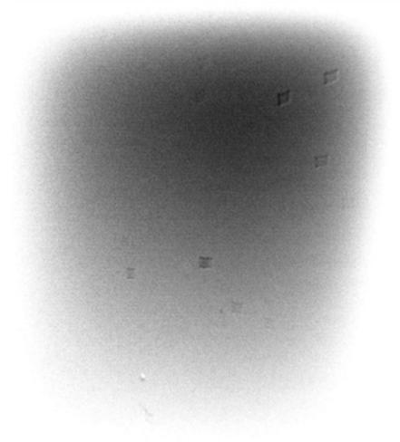
FIG. 27. The effect of small holes in the external filter (courtesy of N. Marshall, UZ Leuven).
