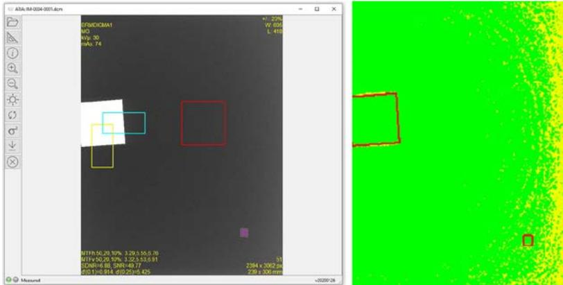
FIG. 8. A mammography phantom image loaded into the automated tool for image analysis (ATIA) (left) and the corresponding variance map (right) produced by the ATIA.
