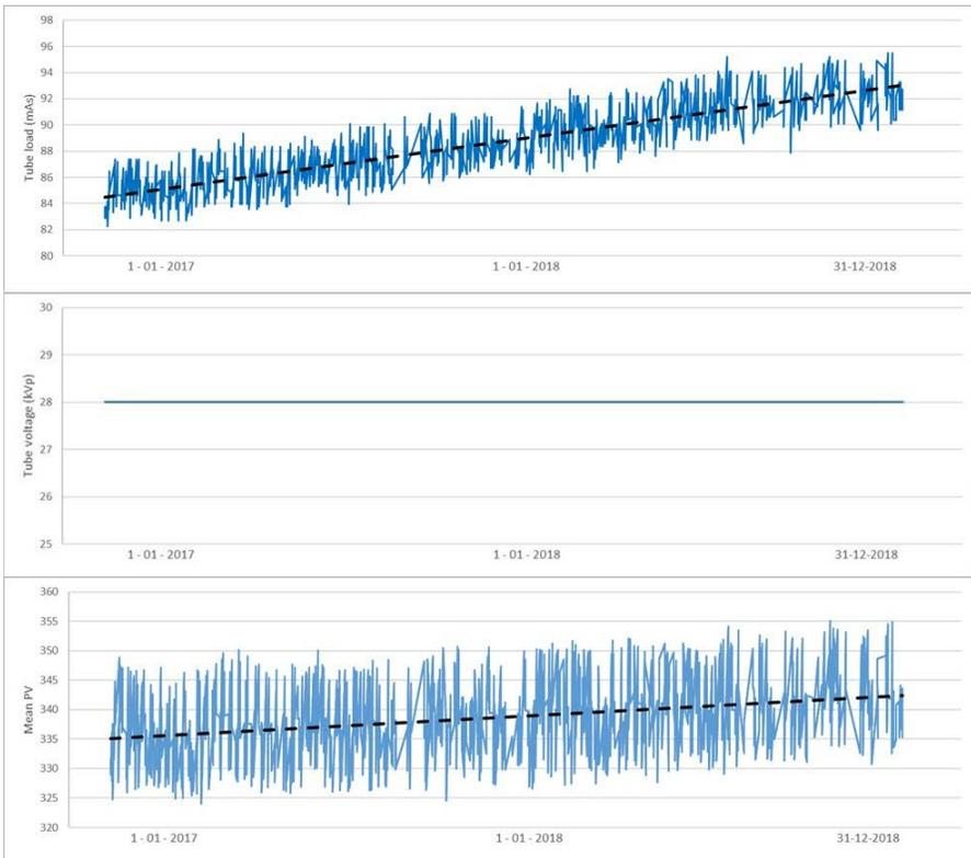
FIG. 19. Run charts of the tube load in mA·s (top), tube voltage in kVp (middle) and mean pixel value (bottom) of a system, indicating a gradual degradation of the system performance. The automatic exposure control compensates for a gradual degradation of either tube or detector by increasing the tube load. The tube load increase is larger than the mean pixel value increase (courtesy of J. Binst, UZ Leuven).
