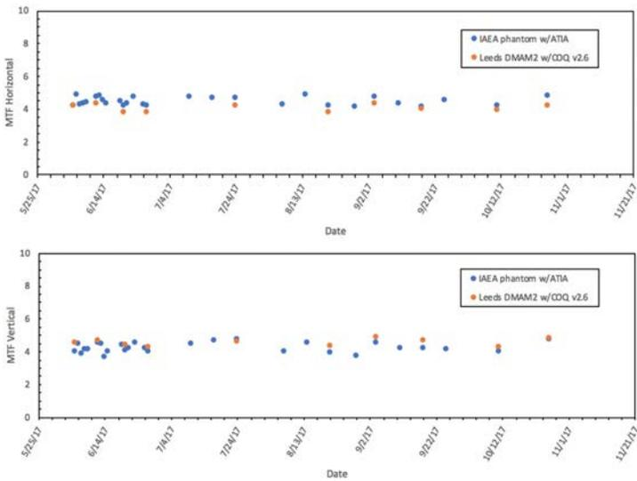
FIG. 37. Graphs demonstrating the modulation transfer function (MTF) performance over time. The blue points come from the IAEA phantom and the automated tool for image analysis (ATIA) application. The orange points are from the Leeds DMAM2 phantom analysed with an ImageJ plugin (COQ v2.6) [32]. MTF data in both the horizontal and vertical directions are presented. The two sets of data in each direction are identical with the student's t-test result  $p < 0.01$ .
