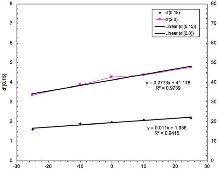
FIG. 38. Sample  $d'$  results of a digital radiography unit, confirming the expected linear response of  $d'$  with respect to the automatic exposure control setting in a digital radiography unit.
