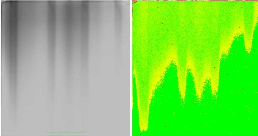
*FIG. 31. Severe streak artefacts caused by damage to the phosphor screen by the rollers in the computed radiography reader, as they appear in a uniform image (left) and in the corresponding variance map (right). Note that the variance range in the automated tool for image analysis (ATIA) was set to 10% and 110% to generate this image.*
