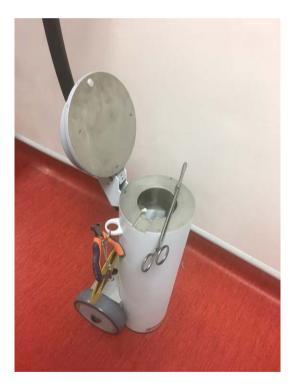
FIG. 34. When transporting low dose rate sources, a mobile shielded container needs to be used and the shortest route possible needs to be taken. A container with a long handle and/or a long-handled trolley can be used. The same container can also be used as emergency equipment for the placement of a high dose rate source if the source becomes stuck during a treatment. Note the wire cutters on the container. (Courtesy of Vetotech, Villeneuve d'Ascq.)
