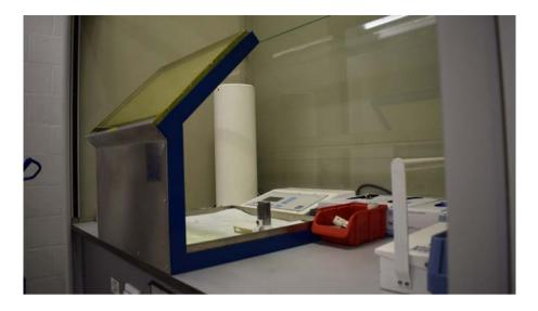
FIG. 27. Detail of the working space. The surface of the working space is covered with plastic backed absorbent paper. Note the dose calibrator to the left of the L-block shielding. A lead shielded syringe carrier is present to the right, and on the working space of the L-block shield there is a lead syringe and bottle shield.
