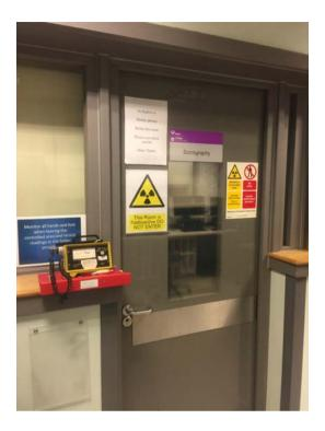
FIG. 22. The entrance to a scintigraphy room (controlled area). The door has the appropriate warning signs and is lockable. To the side of the door is a radiation monitor for monitoring for contamination on the feet and hands of personnel leaving the room. (Courtesy of Royal Veterinary College, London.)
