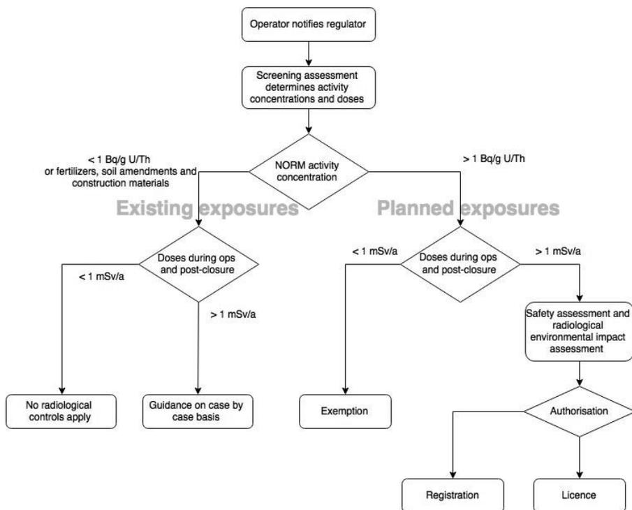
FIG. 3. Graded approach to regulation of NORM (including uranium), as laid out in GSR Part 3 [10].
