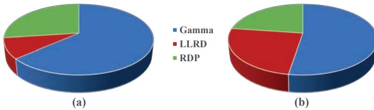
FIG. 35. Occupational exposure contribution from (a) ISL processing and (b) other mines and facilities.
