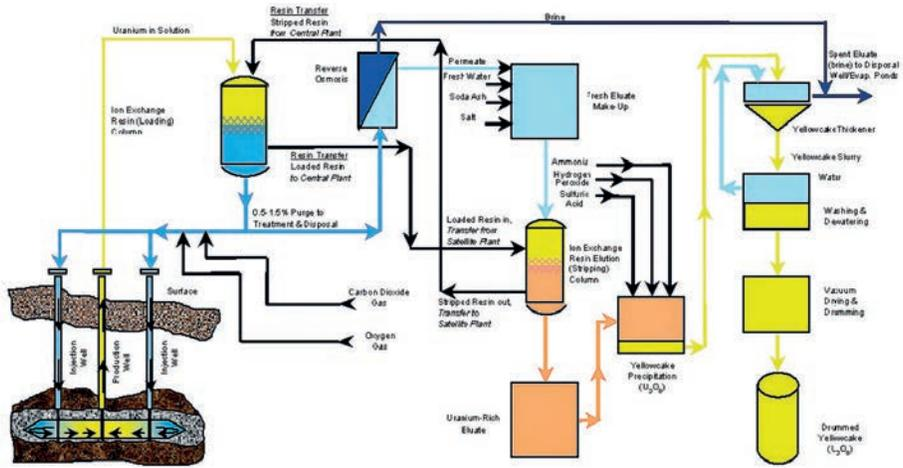
FIG. 6. Alkaline ISL process schematic (United States of America) [25] (fig. 3 of Ref. [22]).
