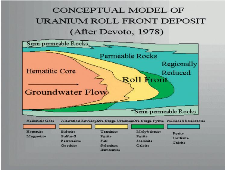
FIG. 4. Redox interface showing a roll front deposit [23] (fig. 1 of Ref. [22]).
