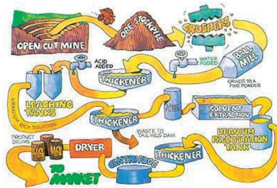
FIG. 13. A simplified uranium processing flow chart (see [www.chemcases.com/nuclear/nc-06.htm](http://www.chemcases.com/nuclear/nc-06.htm)).
