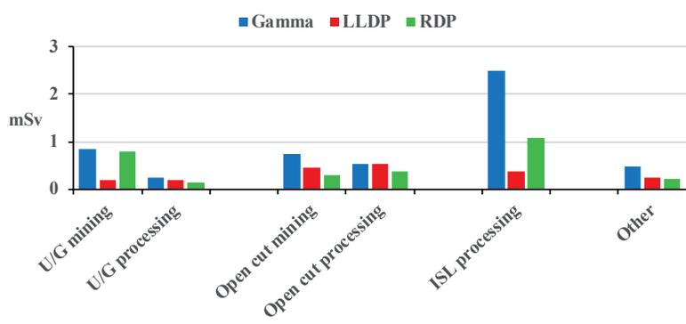
FIG. 31. Average dose with respect to different types of mining and processing.
