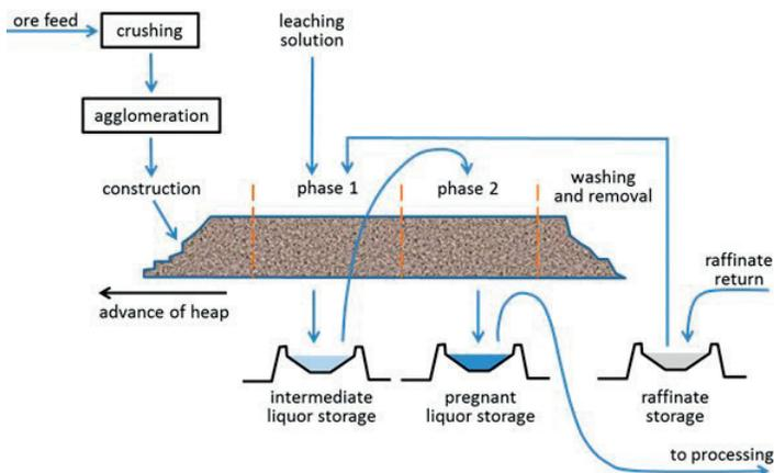
FIG. 12. Heap leaching process (simplified two stage schematic).
