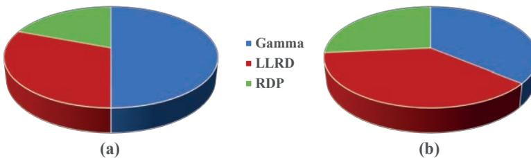
FIG. 34. Occupational exposure contribution from (a) open cut mining and (b) open cut processing.
