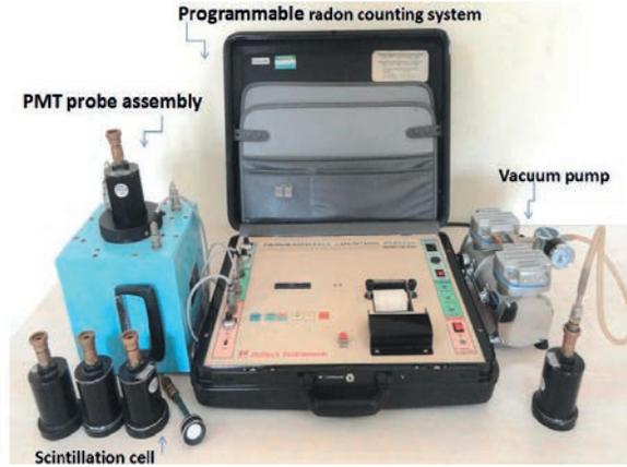
FIG. 41. Programmable radon counting system for the measurement of radon in mine air.
