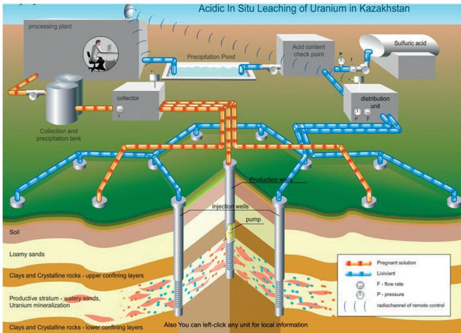
FIG. 7. Acid in situ leach process schematic (Kazatomprom, Kazakhstan).
