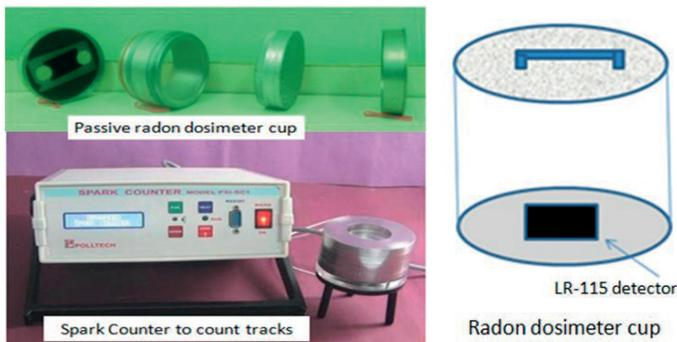
FIG. 43. SSNTD based passive radon dosimeter.
