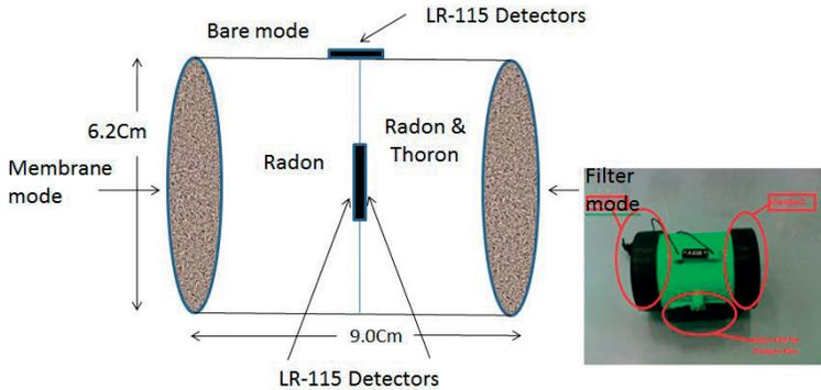
FIG. 44. Twin cup radon–thoron dosimeter.
