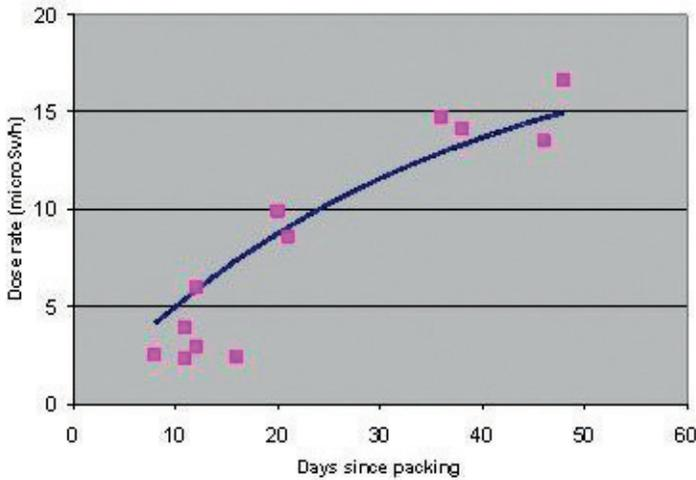
FIG. 15. The increase in gamma dose rate from uranium product due to  $^{234}\text{Th}$  ingrowth.
