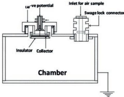
FIG. 42. Low level radon detection system (fig. 1 of Ref. [83]).
