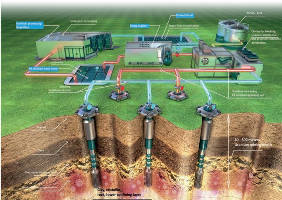
FIG. 5. Basic approach to the in situ uranium mining method (fig. 1-2 of Ref. [24]).
