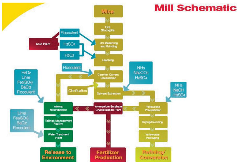
FIG. 14. Specific schematic of the processing (courtesy of D. Chambers, SENES Consultants).
