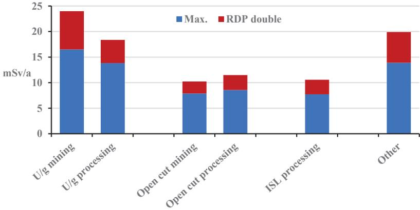
FIG. 40. Fractional contribution of radon and progeny to the total maximum dose.
