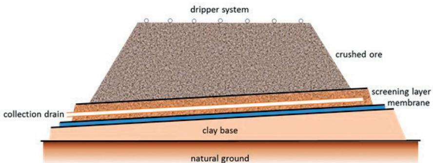
FIG. 11. Heap leaching construction (simplified schematic).
