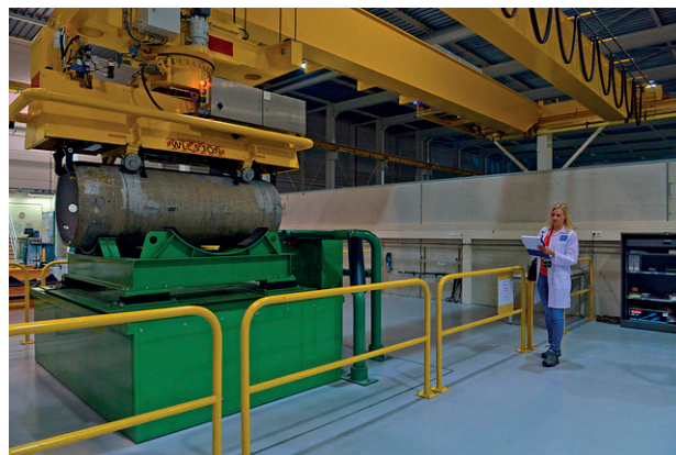
FIG. 13. An inspector weighs randomly selected cylinders on the operator's accountancy scale to verify UF 6 weight.
