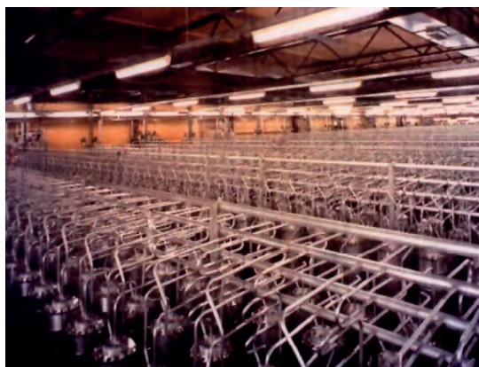
FIG. 1. Centrifuges and piping connections in a commercial uranium enrichment plant.
