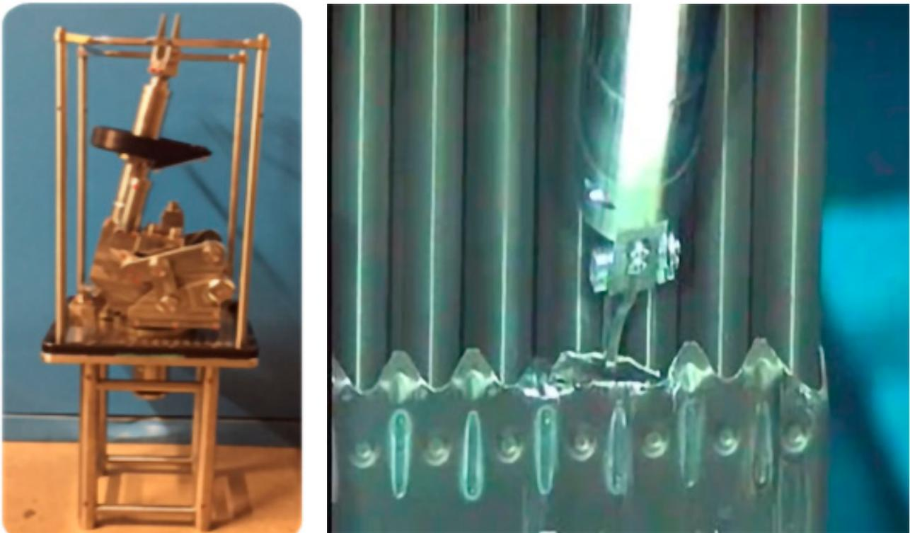
FIG. 34. Example of a gripper tool (left) used on PWRs to retrieve debris from an FA (right). Figure courtesy of *Électricité de France*.
