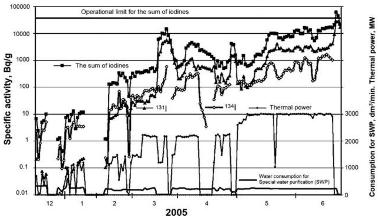
FIG. 37. The specific activity in the primary coolant during operation of Unit 3 of the Kalinin nuclear power plant with a secondary defect in the leaking FR during the first six months of 2005. Figure courtesy of the Institute for Nuclear Research and Nuclear Energy, Bulgarian Academy of Sciences [79].
