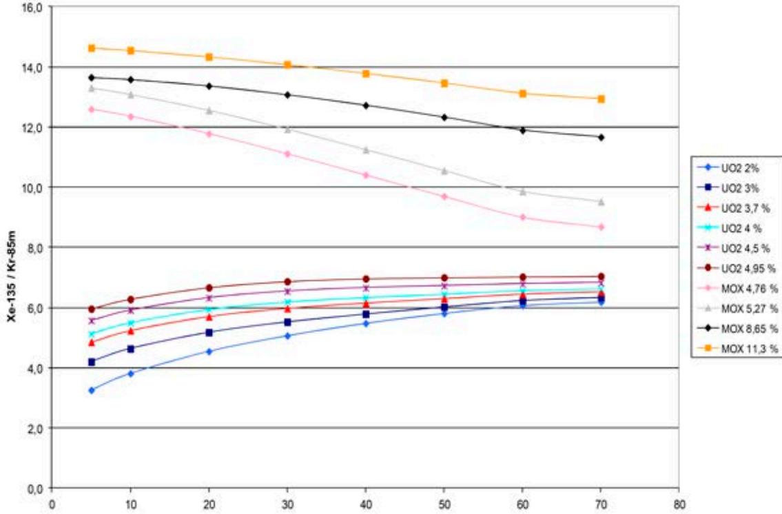
FIG. 24.  $UO_2/MOX$  fuel failure determination based on  $^{135}Xe/^{85m}Kr$  ratio. Figure courtesy of Électricité de France.
