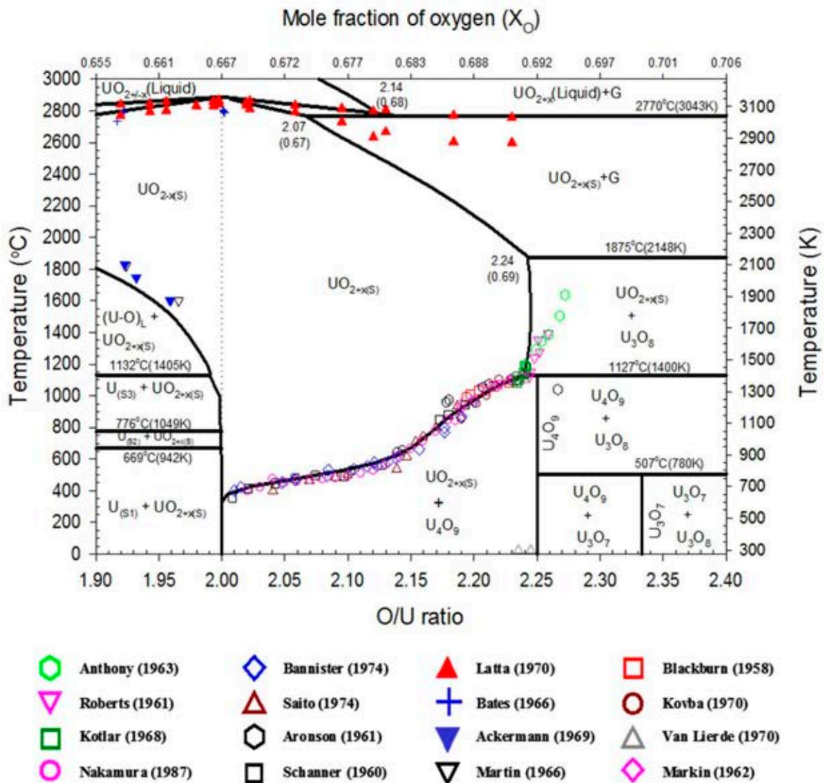
FIG. 28. Calculated phase diagram for the U-O system, highlighting the  $UO_{2+x}$  region, shown against experimental phase boundary determinations. Figure courtesy of the Royal Military College, Canada [66].
