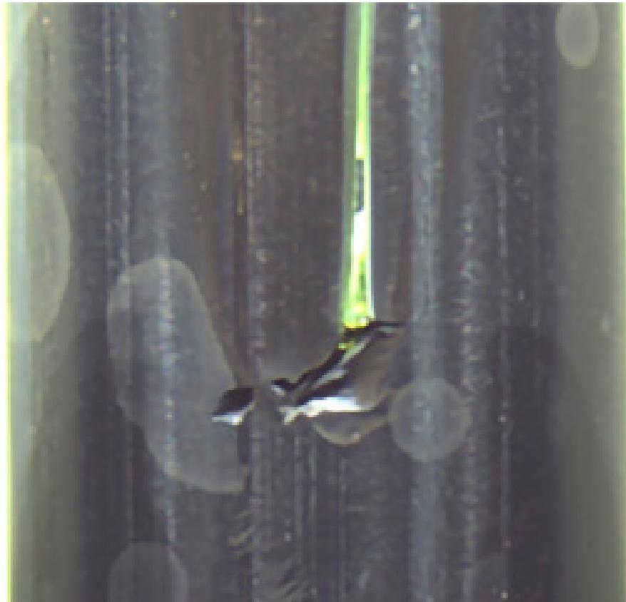
FIG. 26. Early leaker (first cycle) on a FR of an French reactor. Figure courtesy of AREVA NP.
