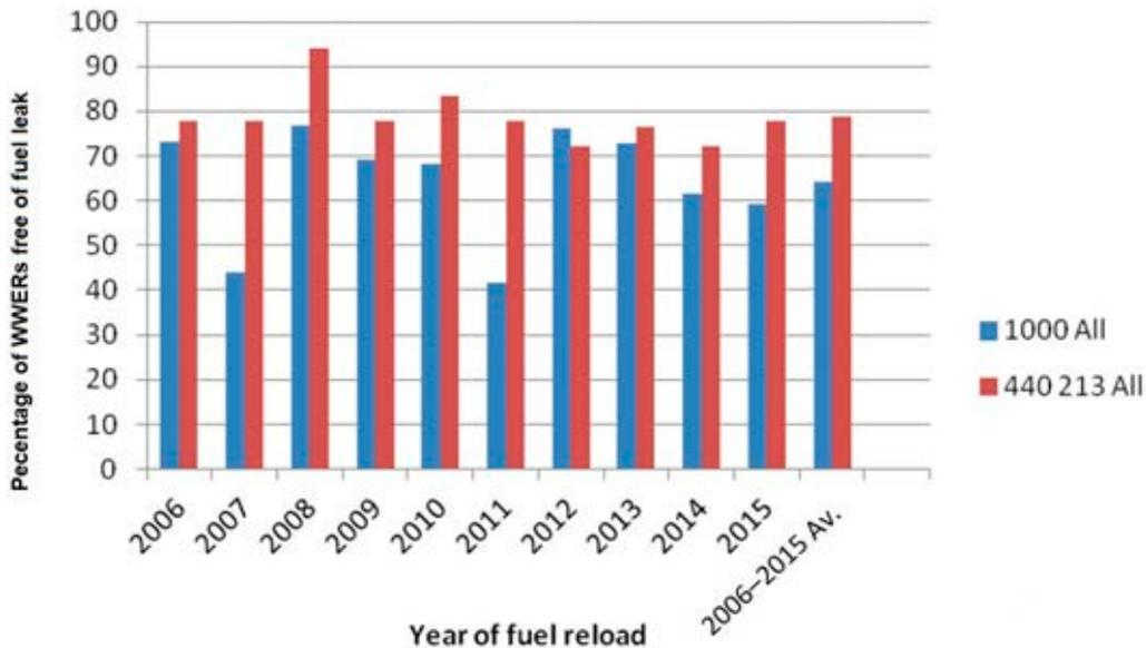
FIG. 16. Percentage of WWER units (all WWER-1000s and WWER-440/213s operated in 2006–2015) with zero fuel ‘leakers’.
