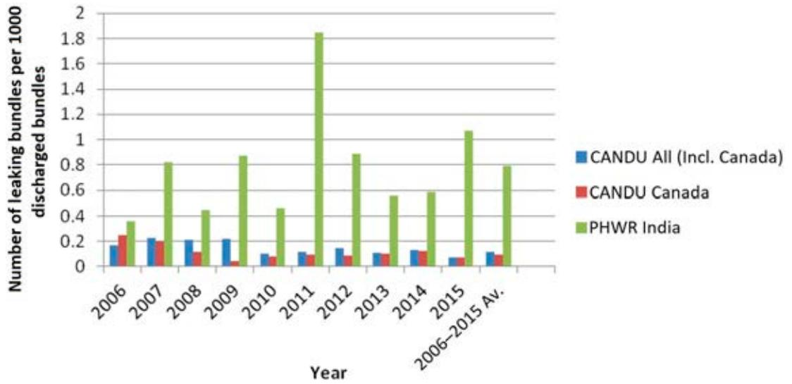
FIG. 17. CANDU and other PHWR fuel bundle failure rates.
