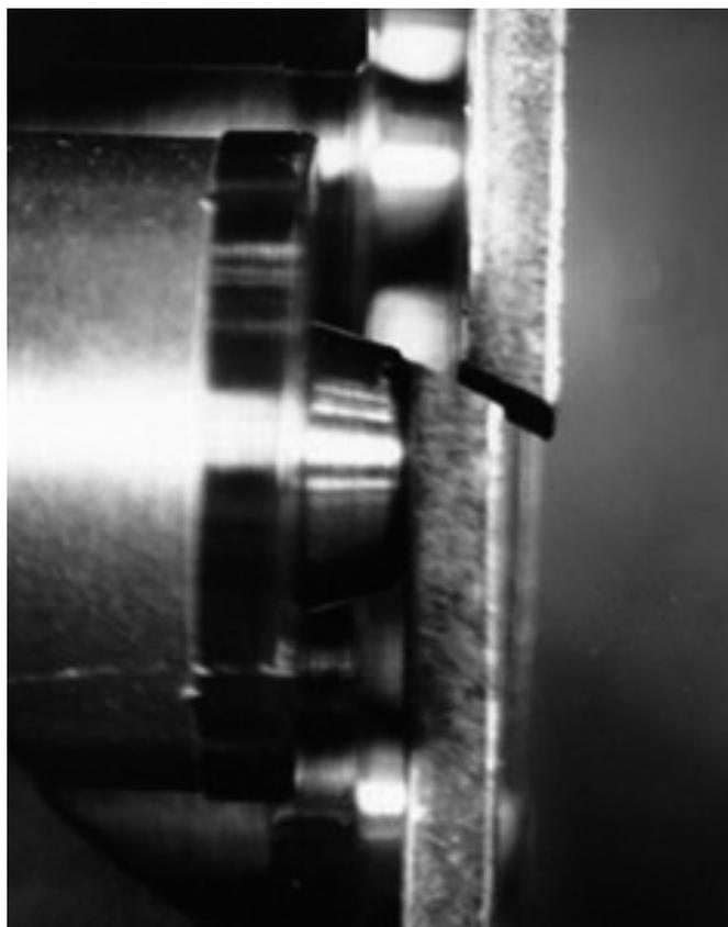
FIG. 33. Endplate fatigue crack. Figure courtesy of SNC-Lavalin, CANDU Energy.
