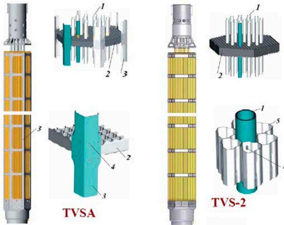
FIG. 22. WWER-1000 FAs with a rigid skeleton TVSA (left) and TVS-2 (right). Legend: 1 — guide tubes; 2 — spacer grid; 3 — angles; 4 — resistance spot welding, 5 — spacer grid cell. Figure courtesy of the Institute for Nuclear Research and Nuclear Energy, Bulgarian Academy of Sciences [29].
