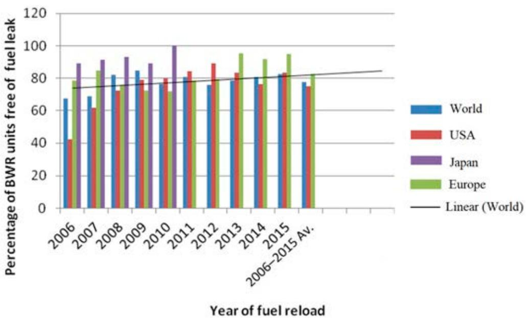
FIG. 11. Percentage of BWR units with zero fuel 'leakers'. Linear extrapolation is for world averages.
