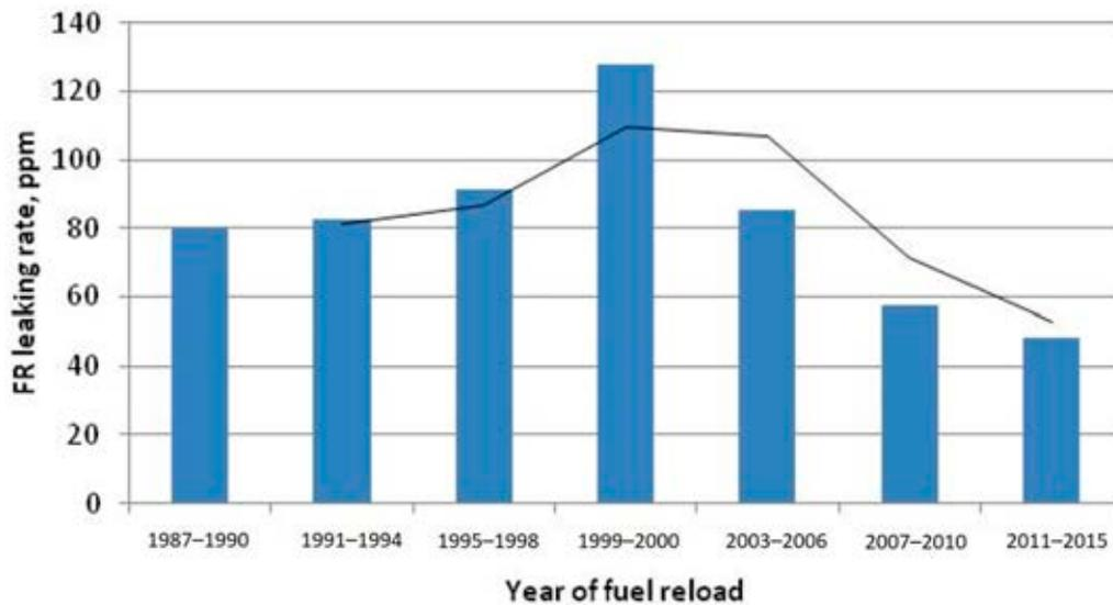
FIG. 15. FR leaking rate for all WWER-1000 and WWER-440/213 units operated in 1987–2015, averaged and grouped in 4 year time intervals.
