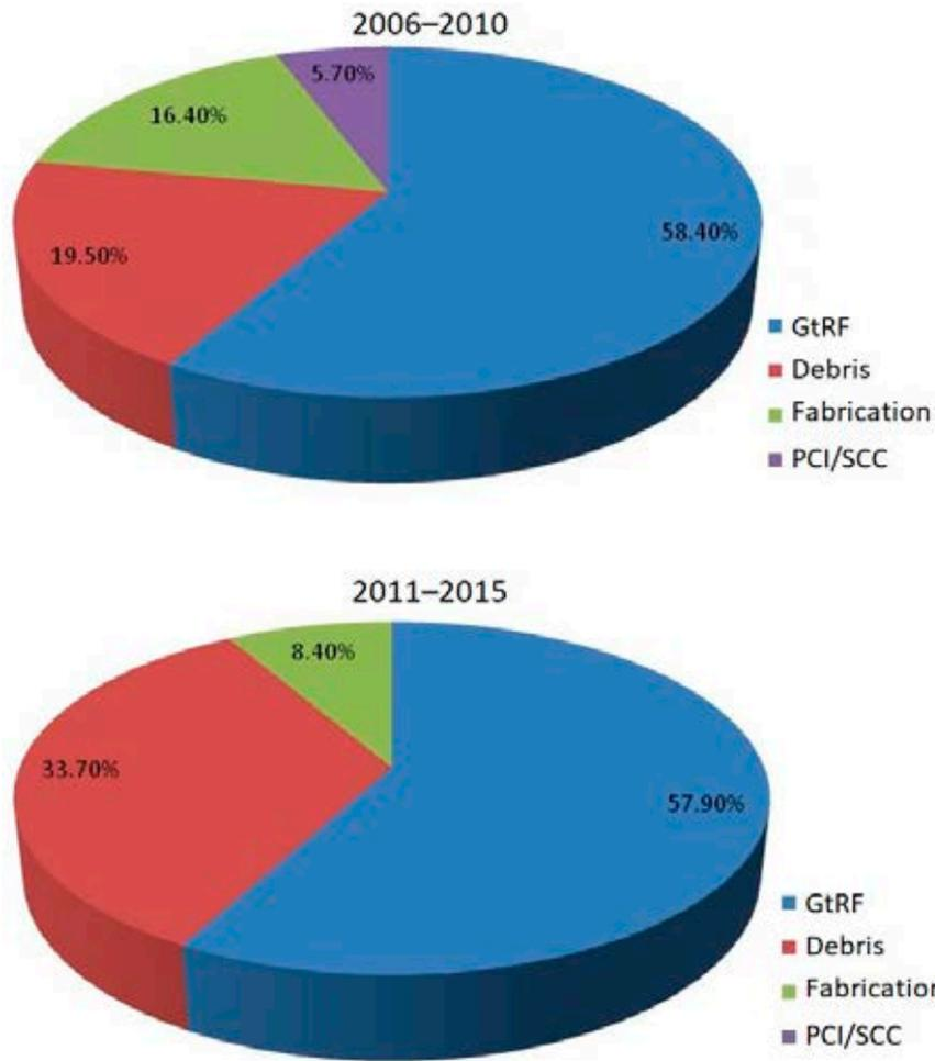
FIG. 5. PWR fuel leak causes worldwide in 2006–2010 (top) and 2011–2015 (bottom). GtRF — grid-to-rod fretting.
