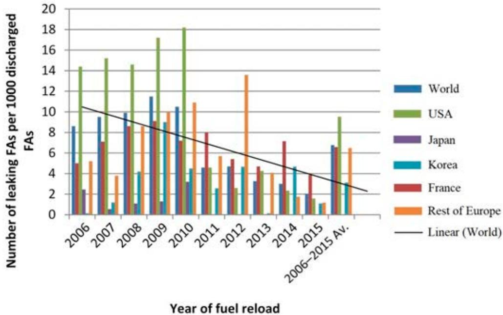
FIG. 2. PWR FA failure rates in 2006–2015. Linear extrapolation is for world averages.
