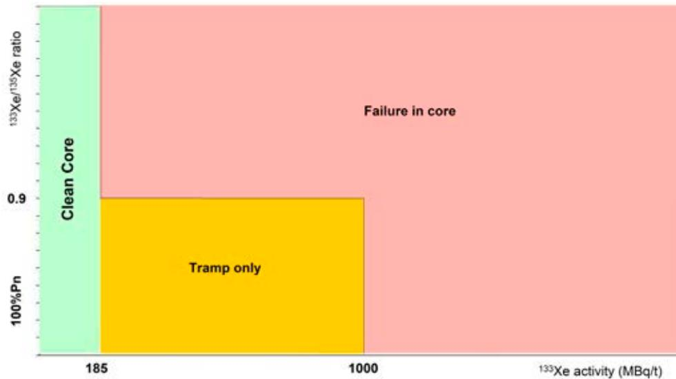
FIG. 23. Fuel failure detection diagram used in France, based on  $^{133}\text{Xe}$  and  $^{135}\text{Xe}$ . Figure courtesy of Électricité de France.
