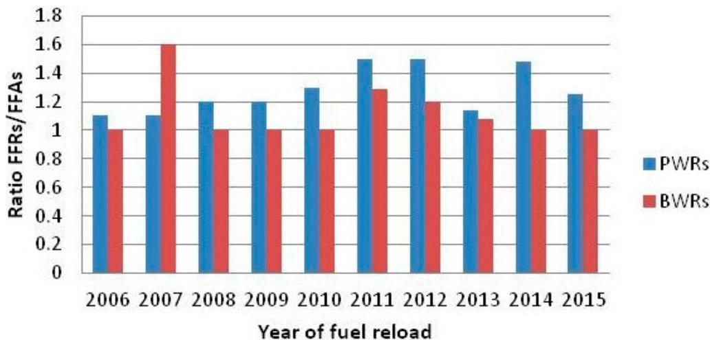
FIG. 1. Ratio of the number of failed FRs to the number of failed FAs in PWRs and BWRs (based on post-irradiation examination results).
