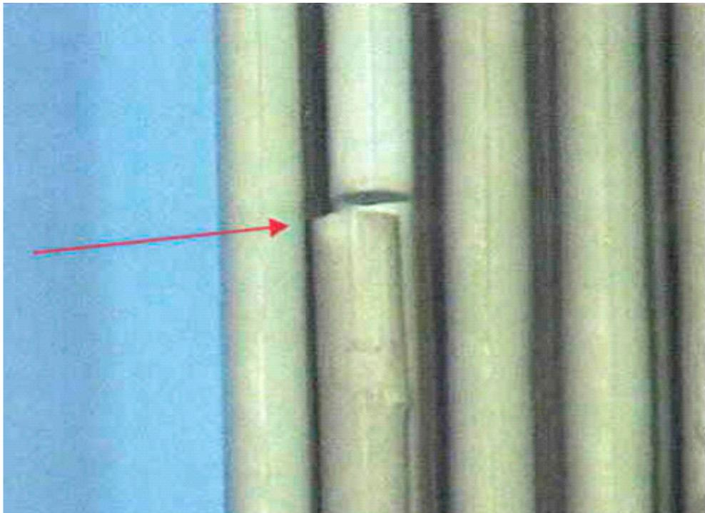
FIG. 36. Example of full circumferential rupture due to secondary hydriding. Figure courtesy of Électricité de France.
