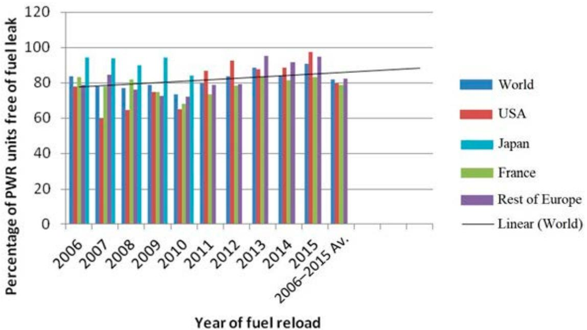
FIG. 6. Percentage of PWR units with zero fuel 'leakers'. Linear extrapolation is for world averages.
