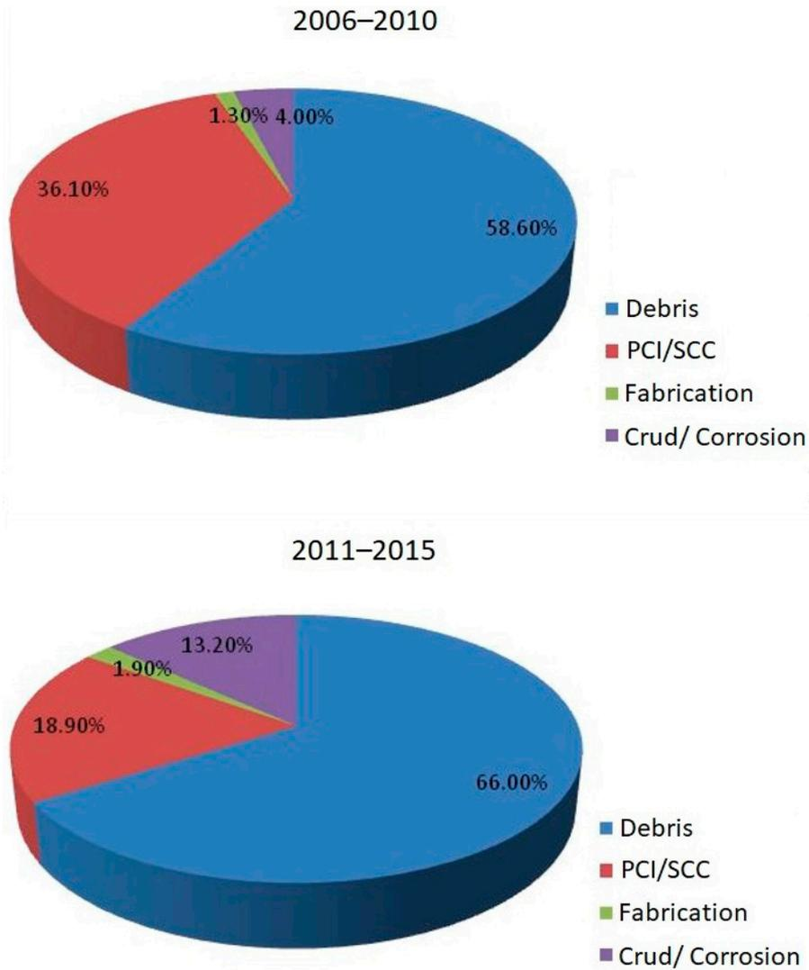
FIG. 10. BWR fuel leak causes worldwide in 2006–2010 (top) and 2011–2015 (bottom).
