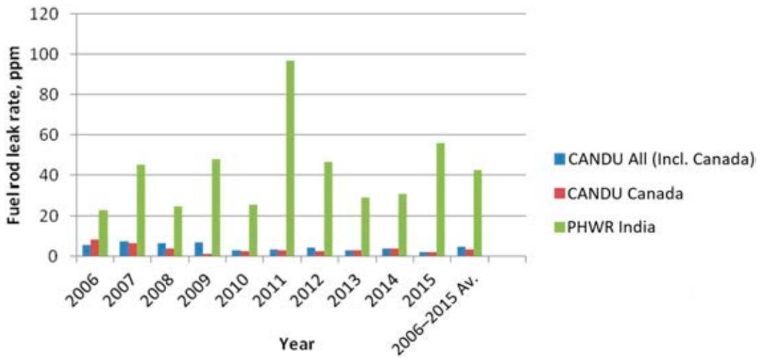
FIG. 18. CANDU and other PHWR fuel element leaking rates in 2006-2015.
