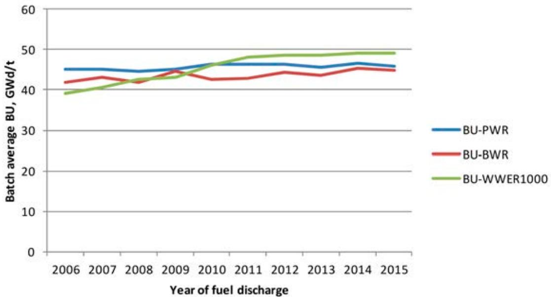
FIG. 20. Dependence of batch burnup averaged for PWRs, BWRs and WWER-1000s as reported by Members of the IAEA Technical Working Group on Fuel Performance and Technology for 2006–2015.
