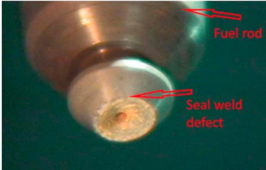
FIG. 25. Seal weld defect on a FR in an French reactor. Figure courtesy of AREVA NP.
