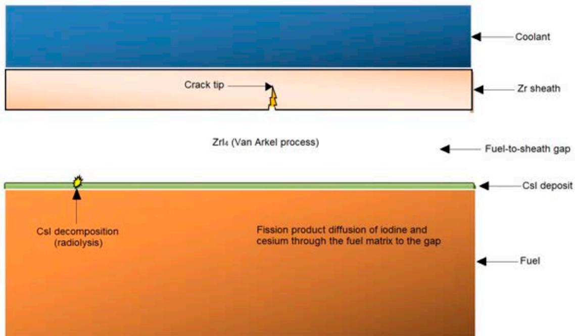
FIG. 27. Schematic of the iodine stress corrosion cracking process for crack penetration. Figure courtesy of the Royal Military College, Canada.
