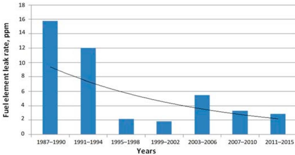
FIG. 19. CANDU fuel element leaking rate in ppm.
