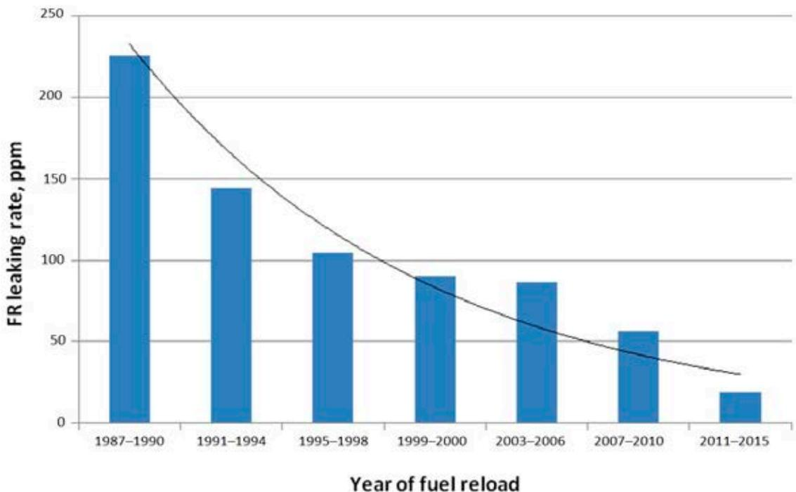
FIG. 4. World average PWR FR failure rates grouped in 4 year periods for the time frame 1987–2015 [3].
