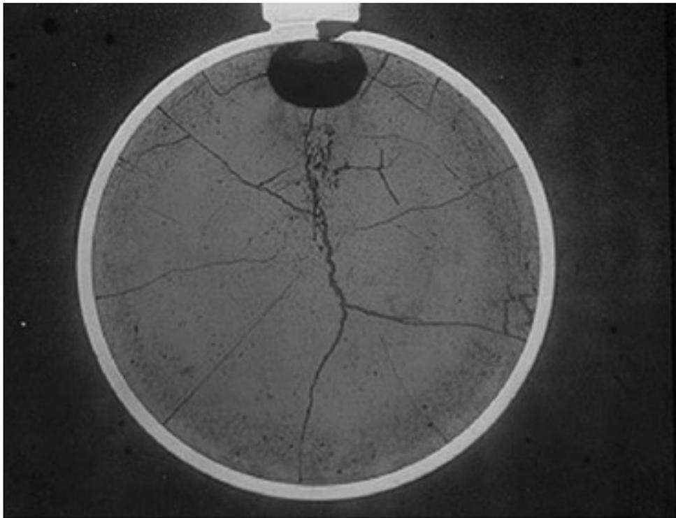
FIG. 32. Primary defect under a pad followed by  $UO_2$  erosion. Figure courtesy of SNC-Lavalin, CANDU Energy.
