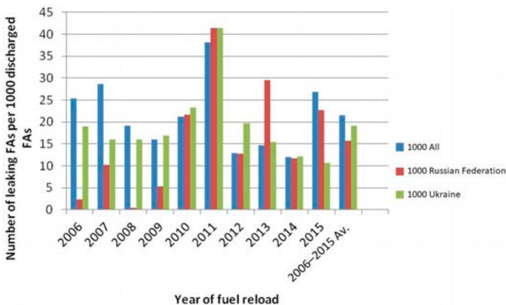
FIG. 13. WWER-1000 FA leak rates in 2006–2015.
