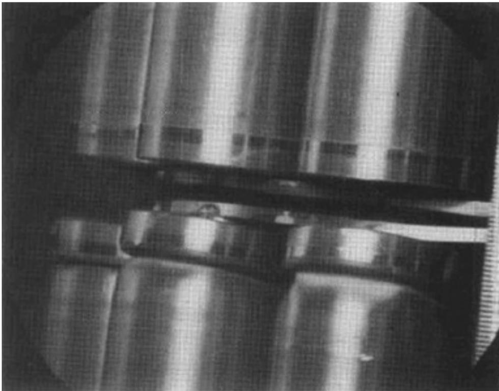
FIG. 31. Sheath axial collapse into axial gaps in a CANDU reactor. Figure courtesy of CANDU Energy.
