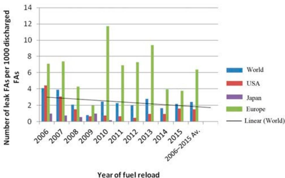
FIG. 7. BWR FA failure rates in 2006–2015. Linear extrapolation is for world averages.
