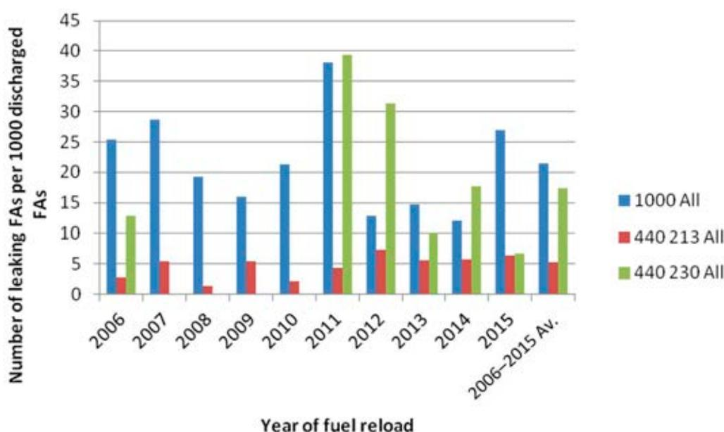
FIG. 12. WWER FA leak rate in 2006–2015.
