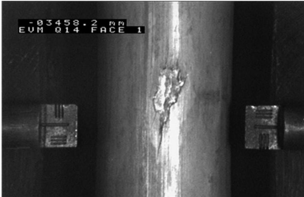
FIG. 35. Example of sunburst due to secondary hydriding. Figure courtesy of AREVA NP.
