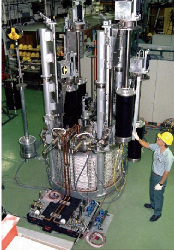
FIG. 52. Electro refining equipment. (Courtesy of USDOE, USA.)
