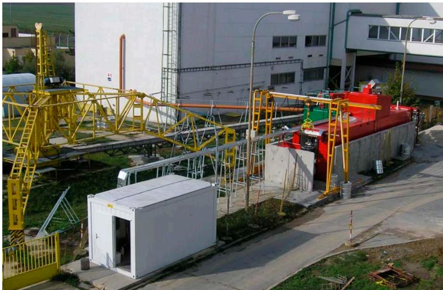
FIG. 20. Long-reach manipulator DENAR-41 and MCF at the A1 NPP. (Courtesy of VÚJE, Slovakia.)
