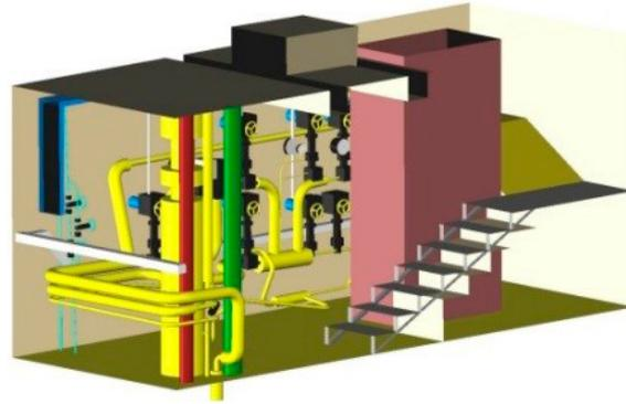
FIG. 12. 3-D laser scanning-panoramic photo, cloud of points and 3-D model. (Courtesy of Nuclear Power Plant Research Institute (VÚJE) Trnava, Slovakia.)
