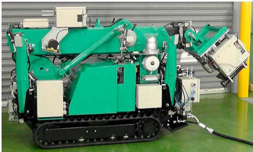
FIG. 13. Remote-controlled robot crawler crane. (Courtesy of International Research Institute for Nuclear Decommissioning (IRID), Japan.)
