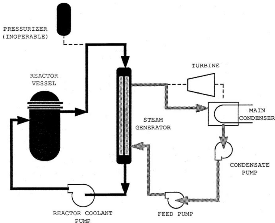
FIG. 10. TMI-2 decay heat removal pathway. (Courtesy of EPRI, USA.)
