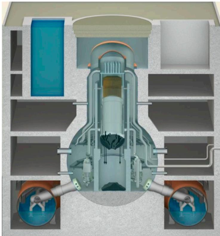
FIG. 43. Illustration of approximate location of fuel debris inside damaged Fukushima Daiichi NPP reactor. (Courtesy of IRID, IAEA and TEPCO.)
