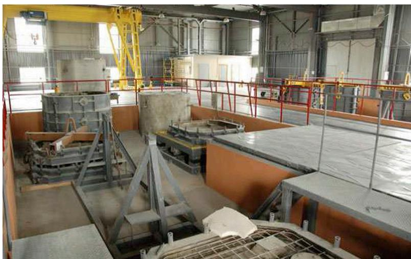
FIG. 30. Production of metal barrels and reinforced concrete containers. (Courtesy of Chernobyl NPP, Ukraine.)
