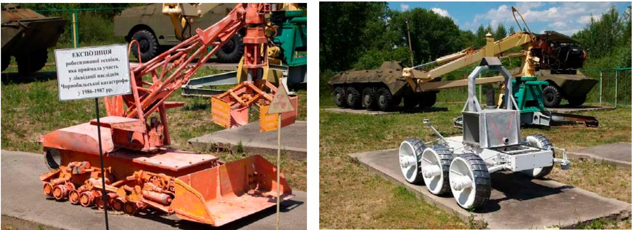
FIG. 16. Remote-controlled decontamination machines used at the Chernobyl NPP. (Courtesy of Chernobyl NPP, Ukraine.)
