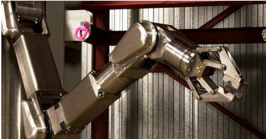
FIG. 46. Remote manipulator system Maestro. (Courtesy of Cybernétix, France.)
