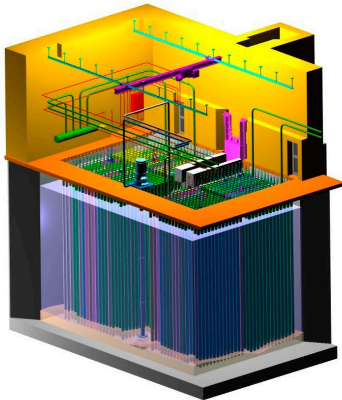
FIG. 33. A 3-D model of the A1 NPP long term storage pool. (Courtesy of AllDeco, s.r.o., Slovakia.)
