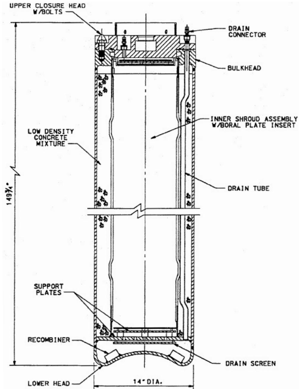
FIG. 45. TMI-2 fuel debris canister. (Courtesy of EPRI, USA.)
