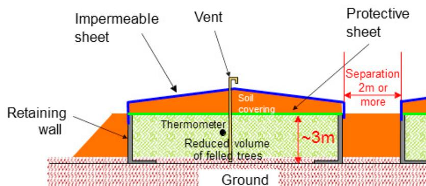
FIG. 21. Schematic of a soil covered storage facility for branches, leaves and roots. (Courtesy of TEPCO, Japan.)
