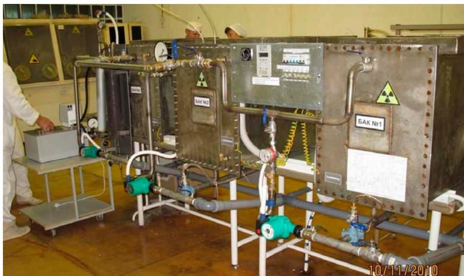
FIG. 18. Pilot facility for shelter object water treatment. (Courtesy of Chernobyl NPP, Ukraine.)
