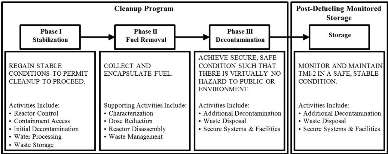
FIG. 1. TMI Roadmap. (Adapted from Electric Power Research Institute (EPRI), with permission).
