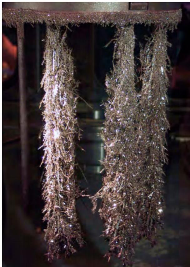
FIG. 53. Uranium product collected during advanced refiner testing. (Courtesy of USDOE, USA.)
