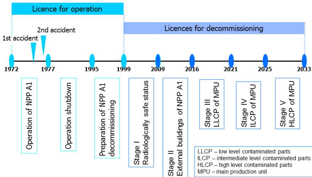
FIG. 2. Stages of A1 NPP decommissioning. (Courtesy of JAVYS, a.s., Slovakia.)
