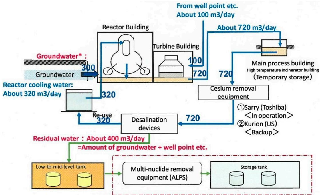
FIG. 19. Overview of contaminated water management showing water volumes as of March 2015, Fukushima Daiichi, Japan. (Adapted from Ref. [41].)
