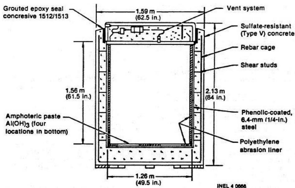
FIG. 25. Reinforced concrete high integrity container. (Courtesy of EPRI, USA.)
