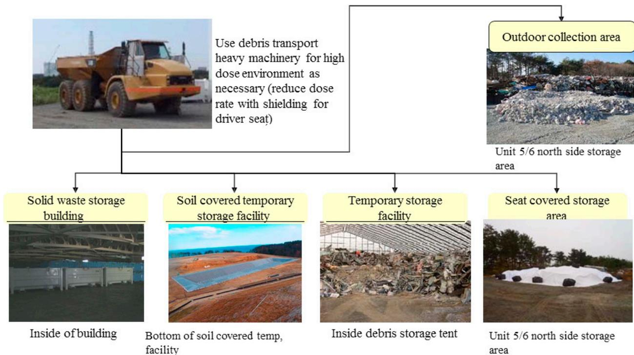
FIG. 23. Examples of facilities constructed for the management and storage of debris. (Courtesy of TEPCO, Japan.)
