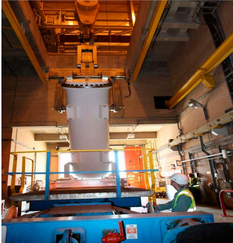
FIG. 50. First fuel being lowered into the THORP receipt and storage building from the rail bay in 1994. (Courtesy of Sellafield Ltd, United Kingdom.)
