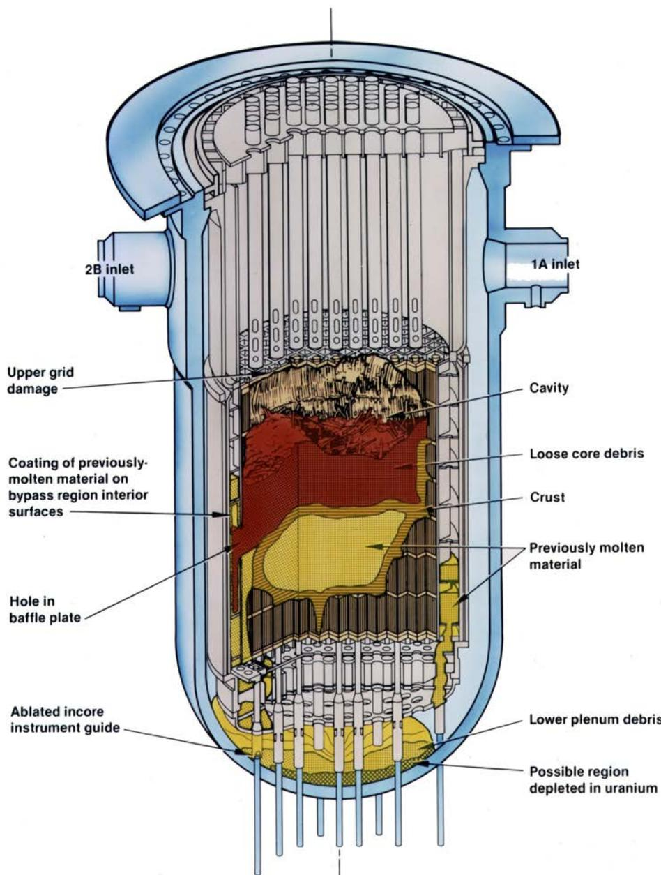
FIG. 34. TMI-2 core damage. (Adapted from Ref. [7].)
