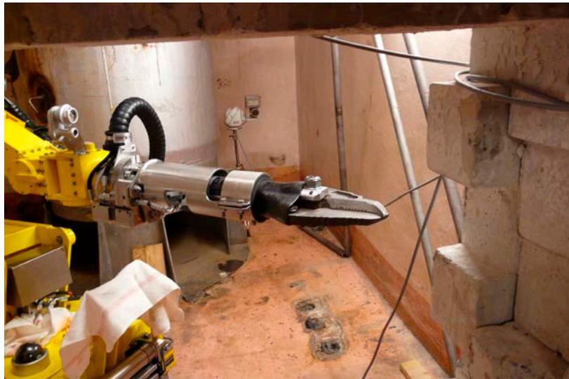
FIG. 15. Remotely operated robotic arm MT-80A. (Courtesy of VÚJE, Slovakia.)
