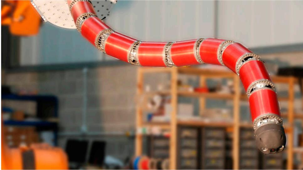
FIG. 39. Snake arm. (Courtesy of Oliver Crispin Robotics limited, United Kingdom.)
