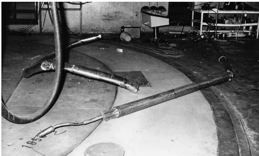
FIG. 31. Damaged fuel assembly on the floor of reactor hall. (Courtesy of JAVYS, a.s., Slovakia.)
