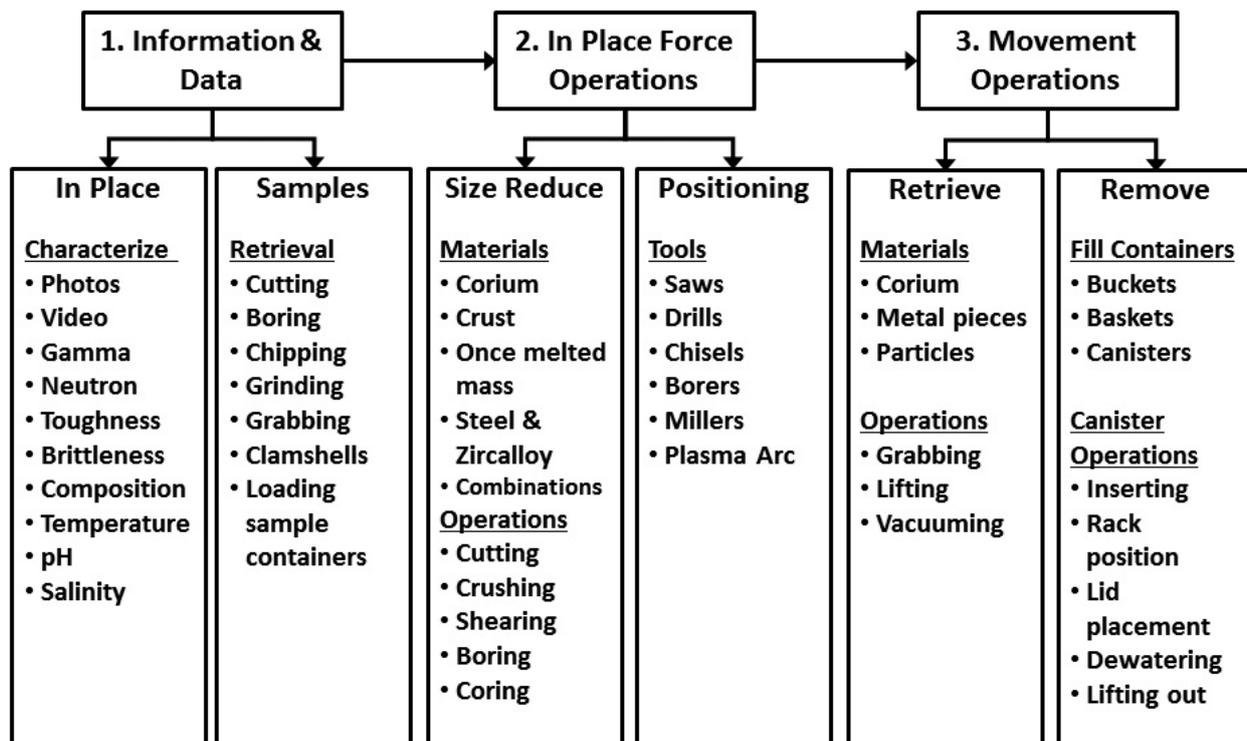
FIG. 44. Functions required for fuel debris removal.
