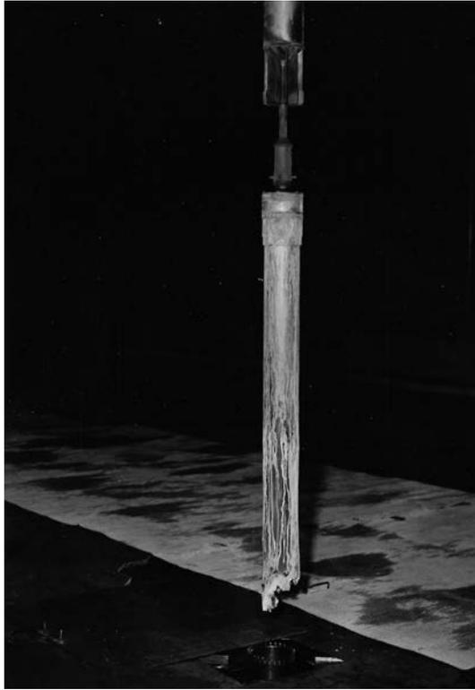
FIG. 32. Part of the overheated fuel assembly after its removal from the reactor. (Courtesy of JAVYS, a.s., Slovakia.)
