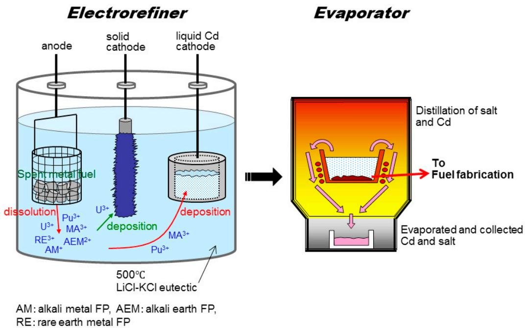
FIG. 51. Principle of separation by electrorefining. (Courtesy of Central Research Institute of Electrical Power, Japan.)
