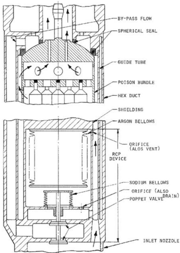
FIG. 43. Rate of change pressure switch trip actuator concept [34].
