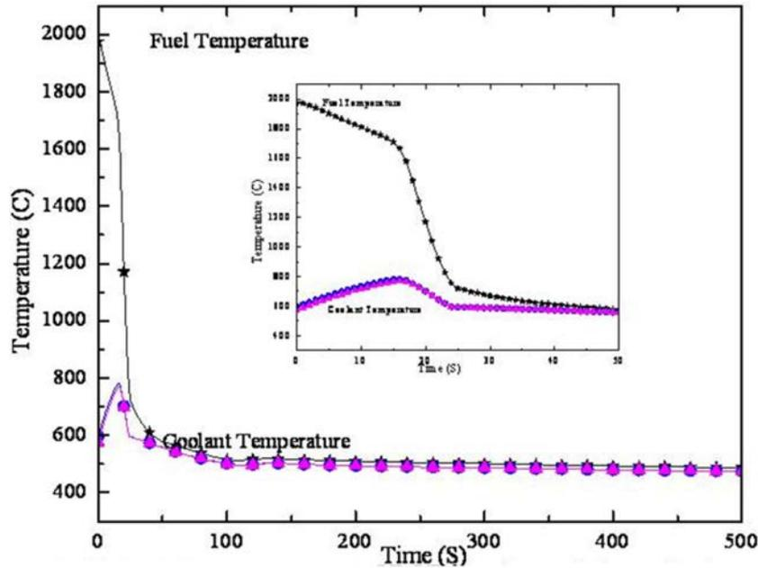
FIG. 60. Evolution of temperature with poison insertion during an unprotected loss of flow event (courtesy of V. Raju Indira Gandhi Centre for Atomic Research).
