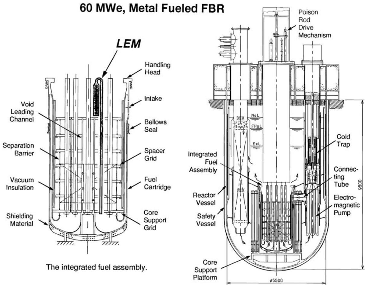
FIG. 48. Reactor structure of a RAPID fast reactor.
