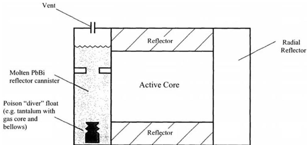
FIG. 11. Alternate Cartesian diver design for use in reflector (reproduced from Ref. [20]).
