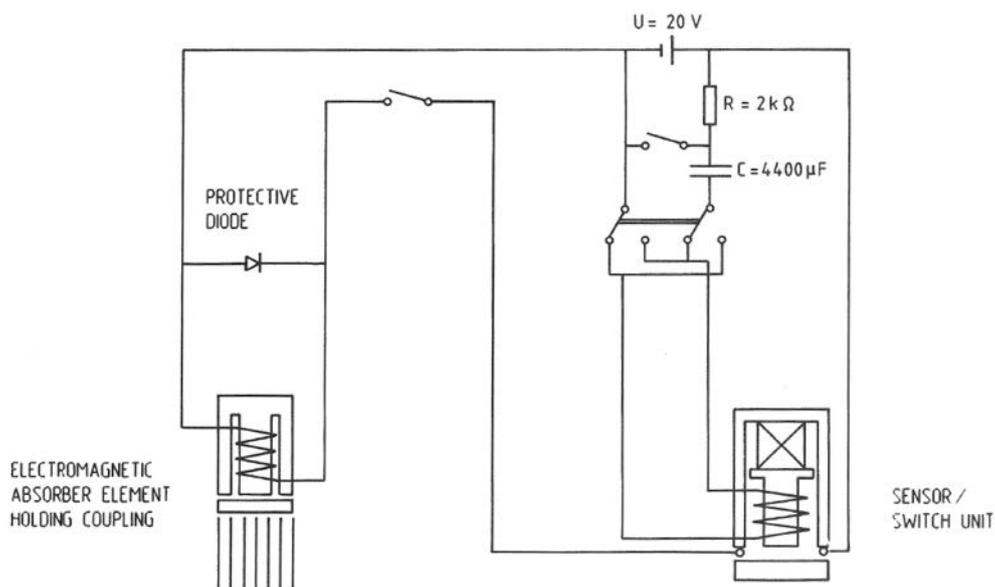
FIG. 39. Electric circuit of the shutdown system [30].
