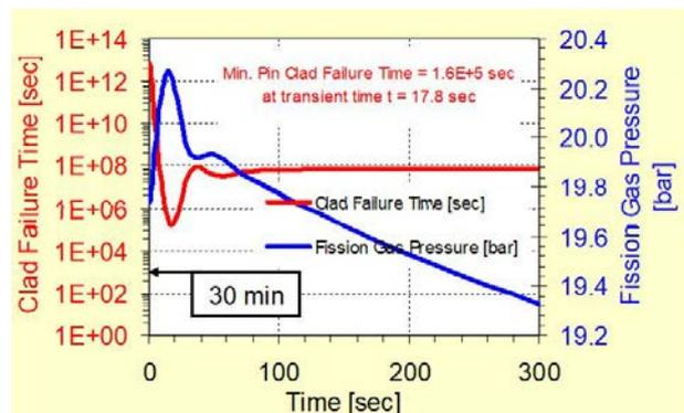
FIG. 86. Cladding failure time and peak pin fission gas pressure.
