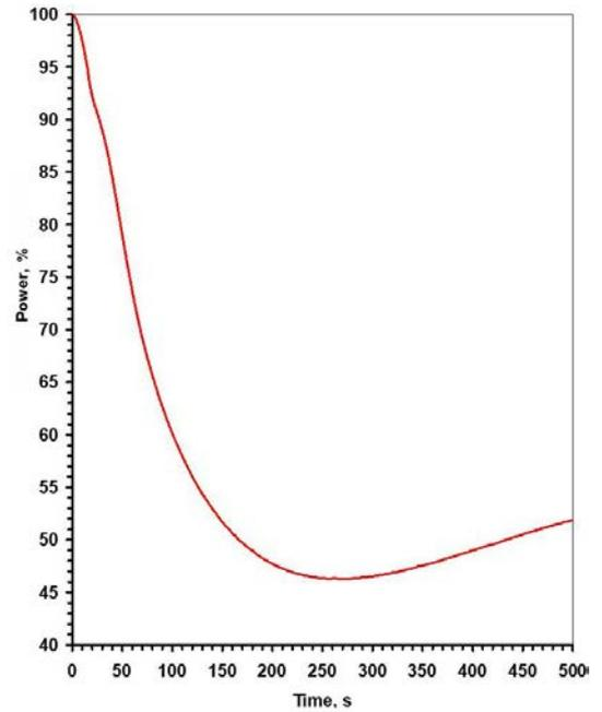
FIG. 68. Reactor power during one primary sodium pump trip event without safety action.
