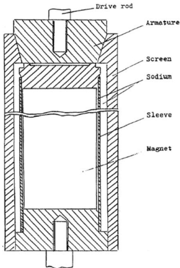
FIG. 34. Mock-up of magnetic actuating device (reproduced from Ref. [18]).
