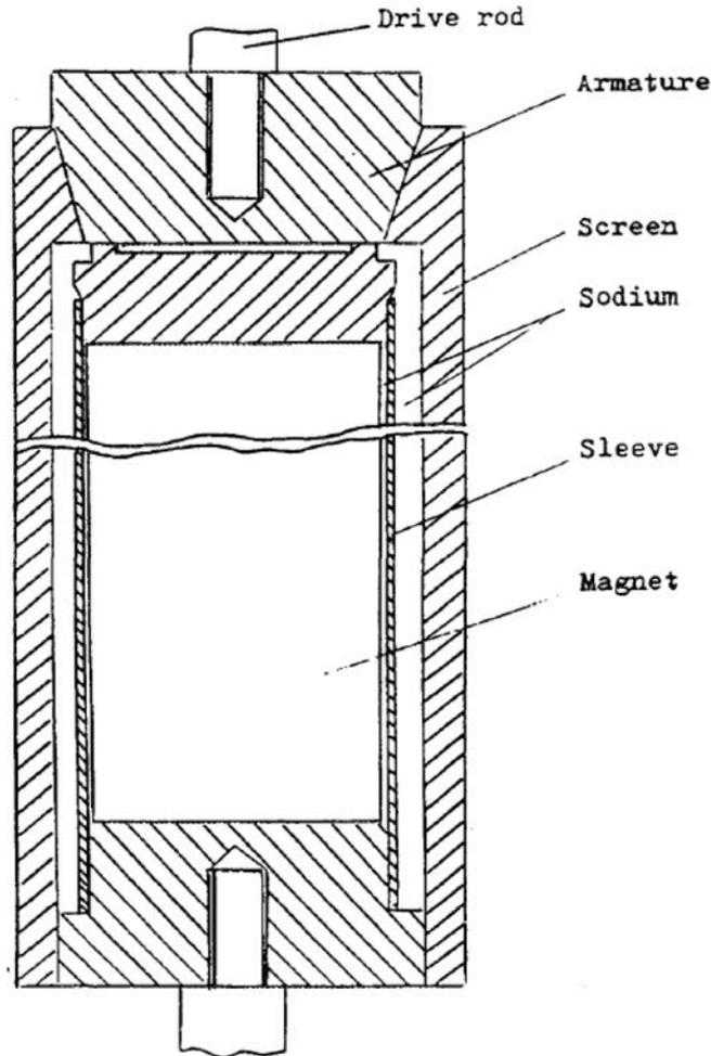
FIG. 63. Mock-up of magnetic actuating device [18].
