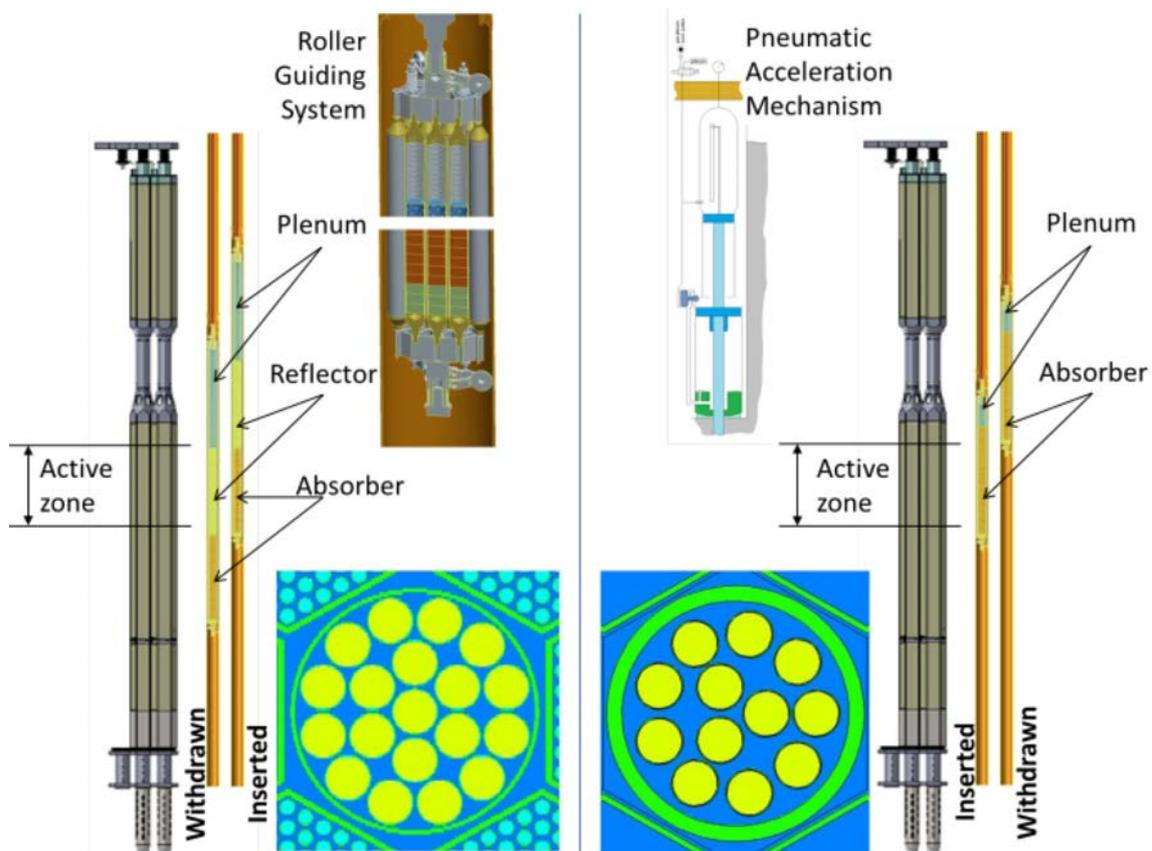
FIG. 78. Schemes and cross-sections of the ALFRED control rods (left) and safety rods (right) (courtesy of L. Burgazzi, Italian National Agency for New Technologies, Energy and Sustainable Economic Development).
