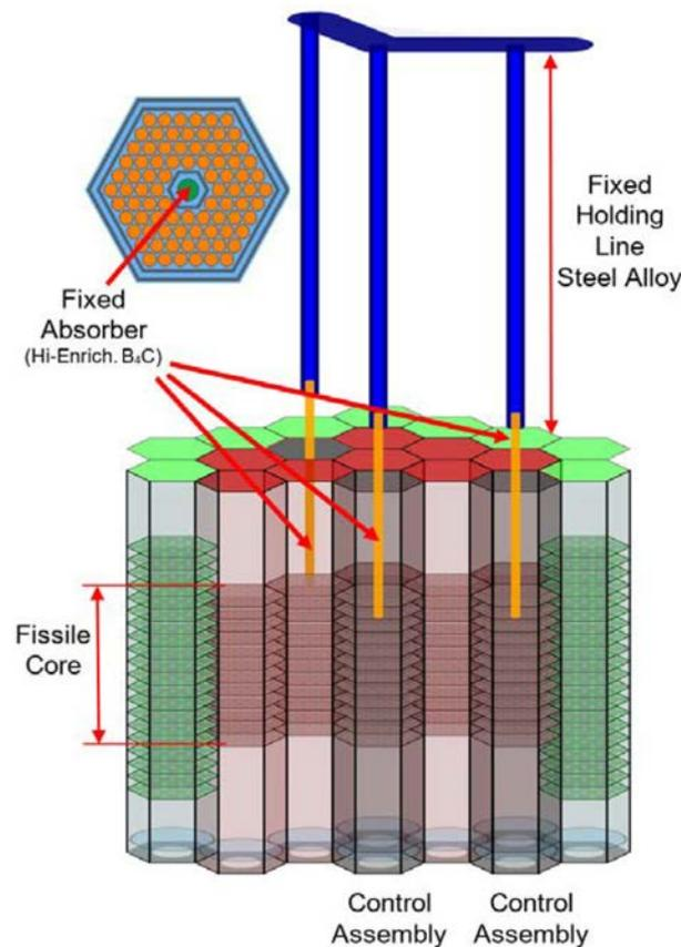
FIG. 22. Static absorber feedback equipment (adapted from Ref. [23]).
