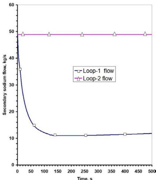
FIG. 71. Secondary sodium flows during one secondary sodium pump trip event without safety action.
