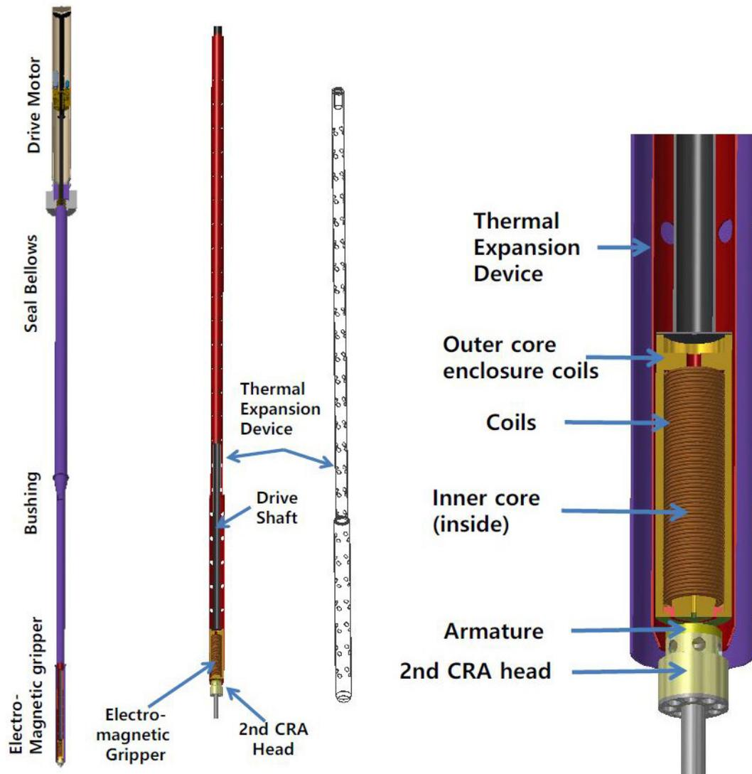
FIG. 52. Passive shutdown concept using a bimetallic thermal expansion device with an electromagnet (courtesy of J. Lee, KAERI).
