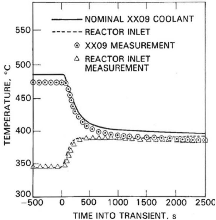
FIG. 66. Unprotected loss of heat sink from 100% power — pretest predictions and measurements of reactor temperatures (courtesy of Argonne National Laboratory).
