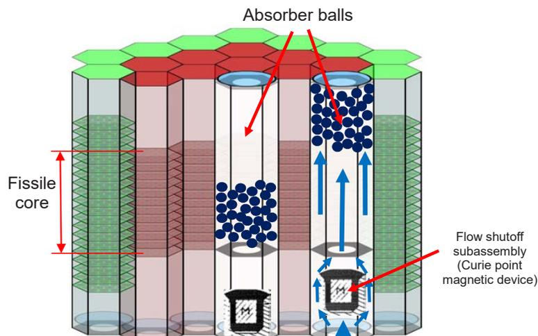
FIG. 12. A levitated absorber system for self-actuated shutdown system (adapted from Ref. [18]).
