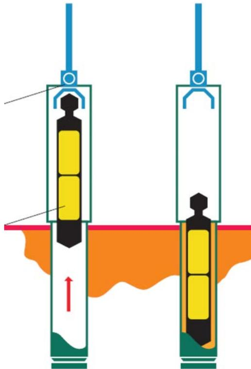
FIG. 33. Passive shutdown rods: pumps in operation (left); pumps out of operation (right) (reproduced from Ref. [15]).
