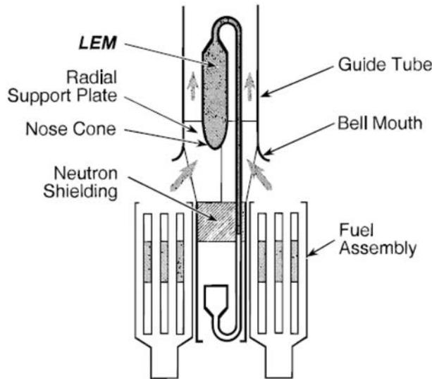
FIG. 49. Lithium expansion module installed in a guide tube to accommodate a conventional core.
