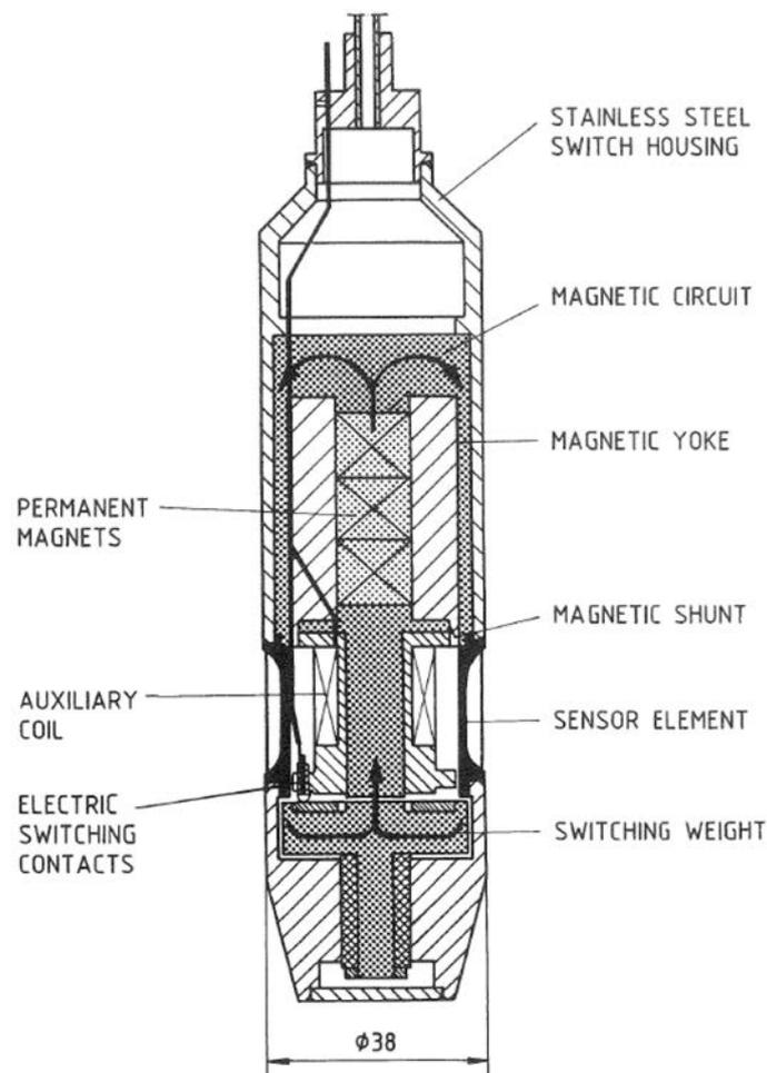
FIG. 38. Curie point controlled sensor/switch unit [30].
