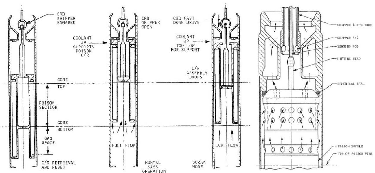
FIG. 41. Basic orifice concept for a levitated absorber assembly design [34].
