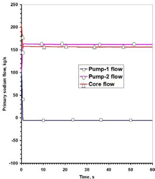
FIG. 69. Primary sodium flows during one primary sodium pump seizure event without safety action.
