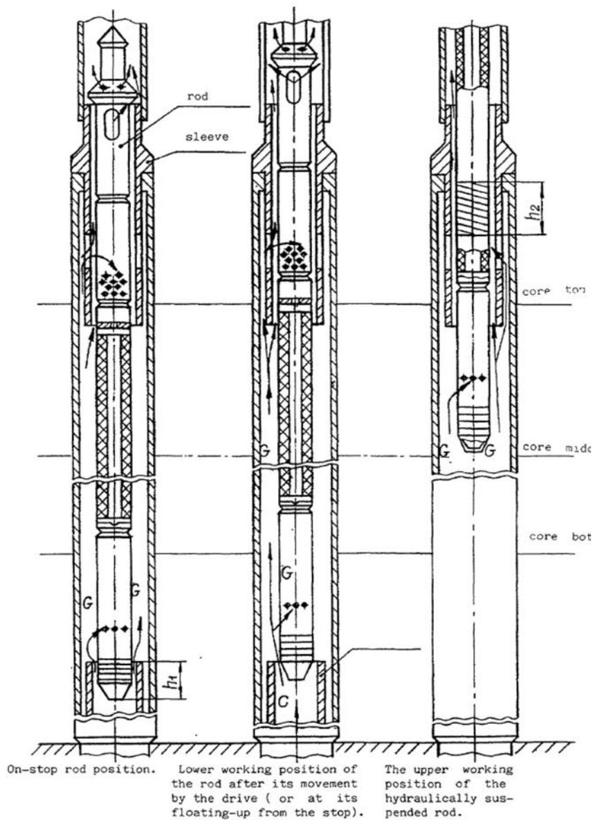
FIG. 29. Passive shutdown system subassembly with hydraulically suspended rod for the BN-600 reactor (reproduced from Ref. [29]).
