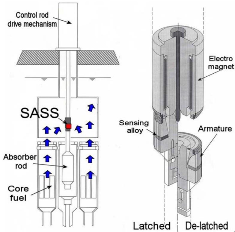
FIG. 91. Curie point concept in self-actuated shutdown systems (reproduced from Ref. [12]).
