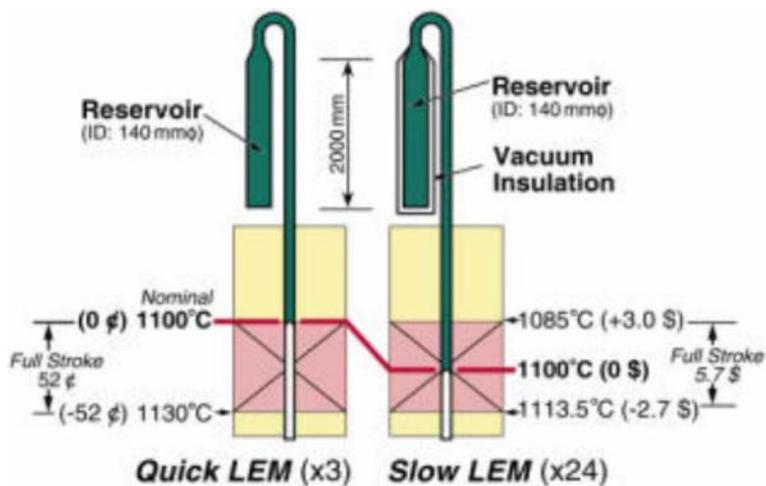
FIG. 2. Elevation of the lithium expansion module gas-liquid interface.
