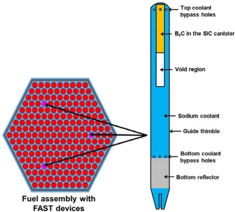
FIG. 61. Floating absorber for safety at transient passive safety device.
