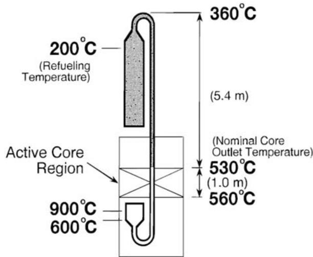
FIG. 47. Elevation of the gas-liquid interface in the liquid expansion module envelope.
