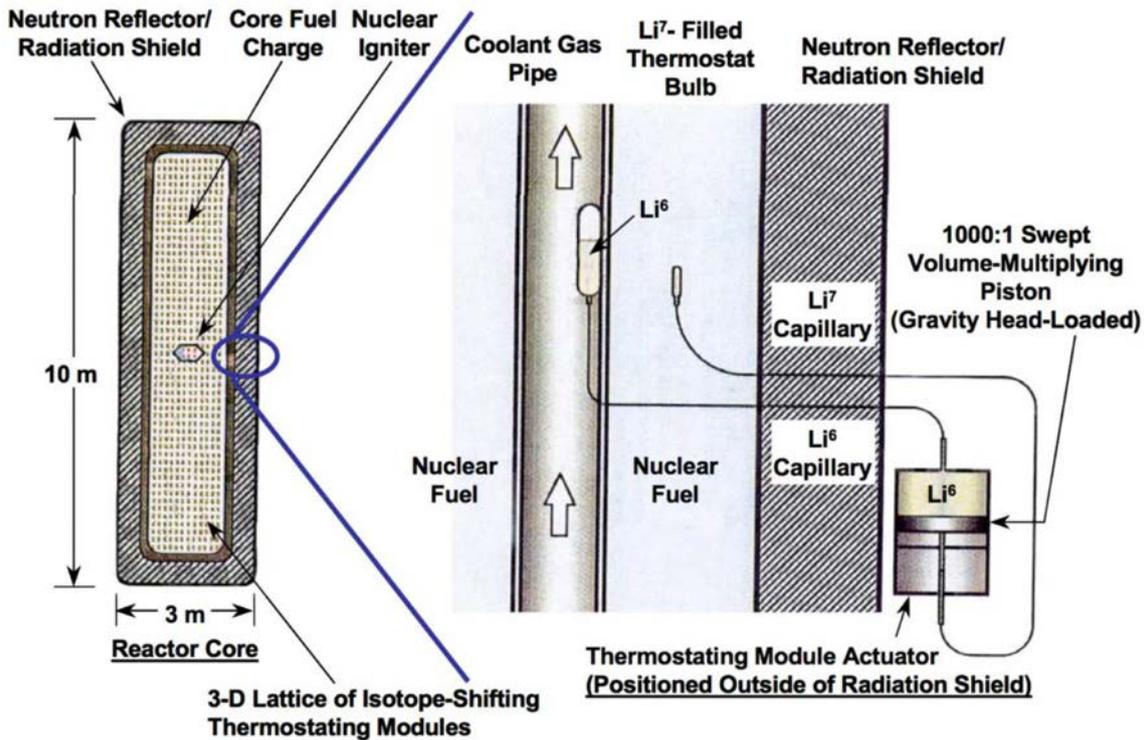
FIG. 20. The travelling wave reactor  ${}^6\text{Li}$  thermostating control system.
