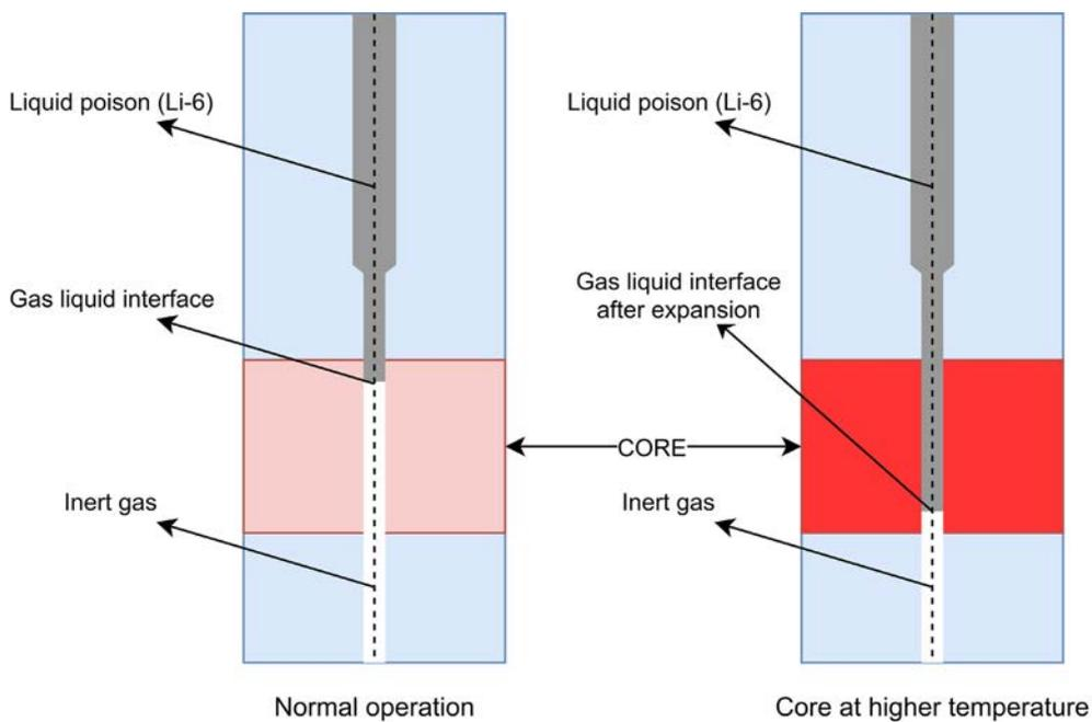
FIG. 1. Lithium expansion module concept.
