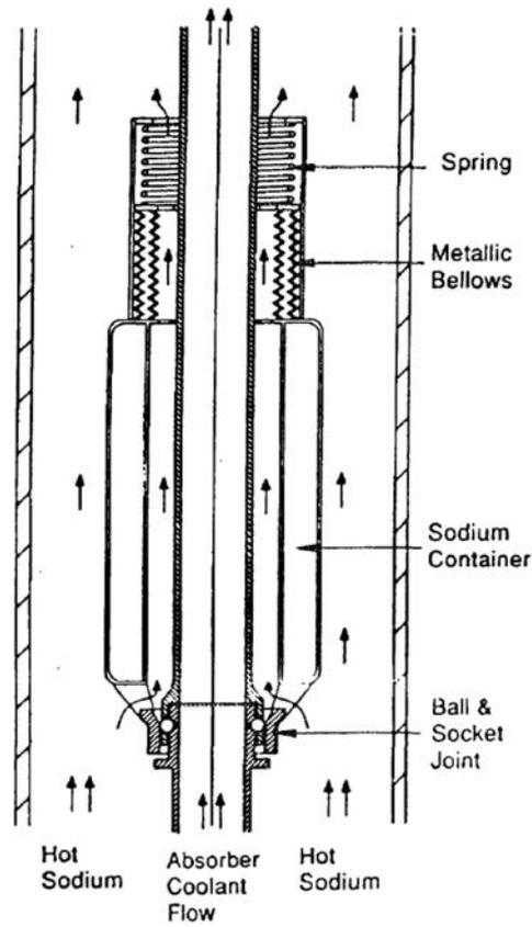
FIG. 14. Enhanced thermal expansion hydraulic concept (reproduced from Ref. [18]).
