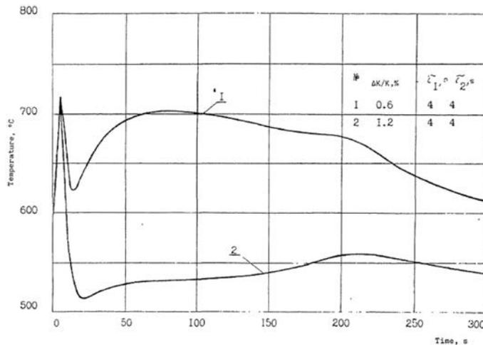
FIG. 31. Sodium temperature at the core outlet as a function of time since the onset of an accident (reproduced from Ref. [29]).
