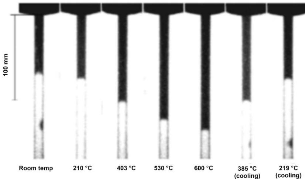
FIG. 46. Neutron radiograph of lithium expansion module [10].
