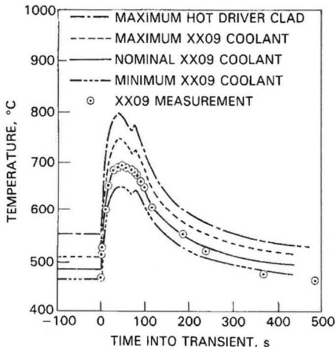
FIG. 65. Unprotected loss of flow from 100% power with 95 second pump coastdown time — predictions and measurements of in-core temperatures (courtesy of Argonne National Laboratory).
