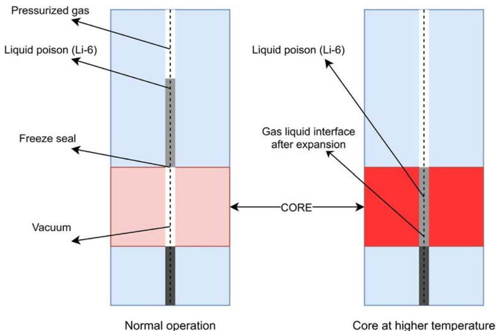
FIG. 3. Lithium injection module concept.
