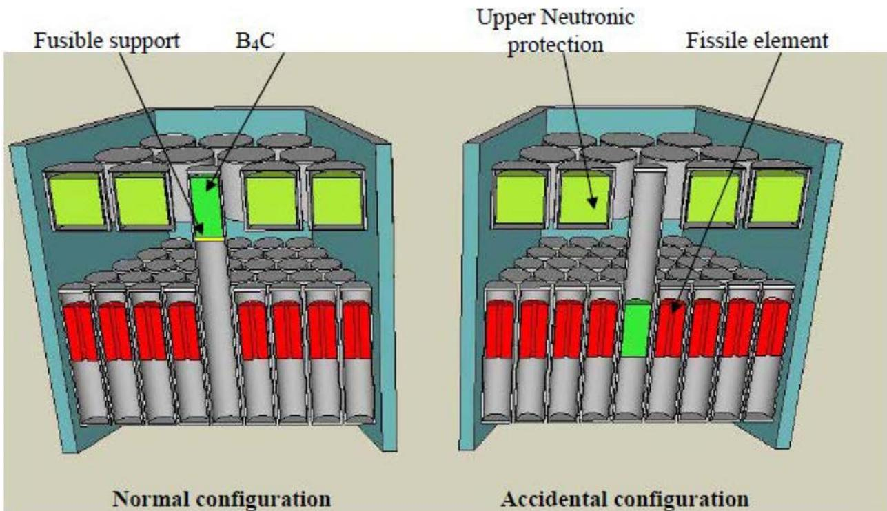
FIG. 64. Self-protected additional shutdown device schematics [53].
