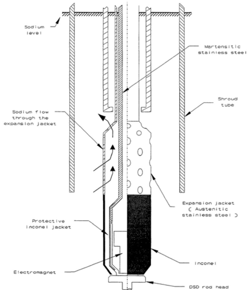
FIG. 16. Thermal expansion device for passive insertion of backup rods in European fast reactor (reproduced from Ref. [18]).
