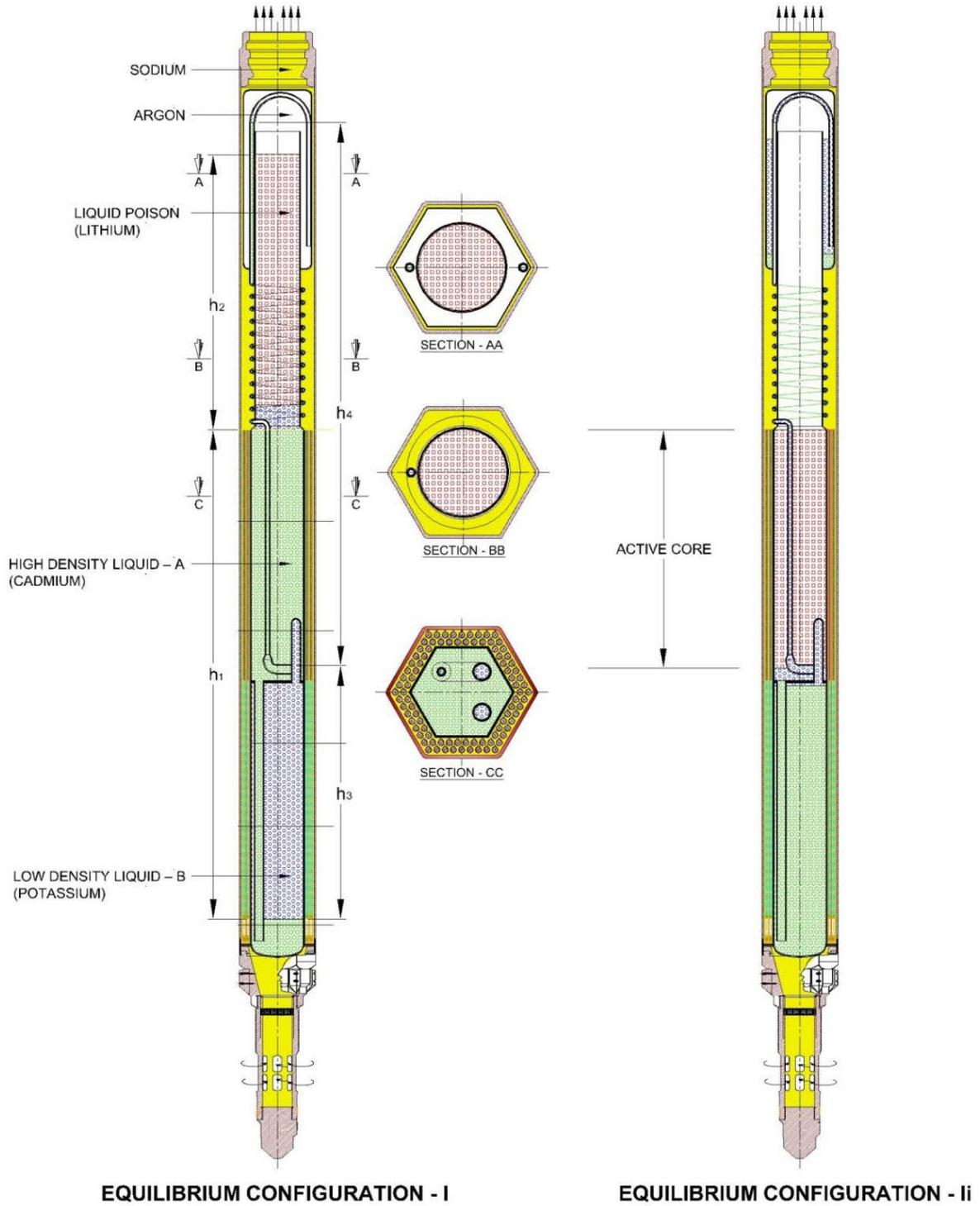
FIG. 56. A thermo siphon passive shutdown subassembly.
