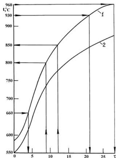
FIG. 8. Change of coolant temperature under beyond design basis accident conditions in the BN-800 reactor: (1) a subassembly with maximal power; (2) the reactor.
