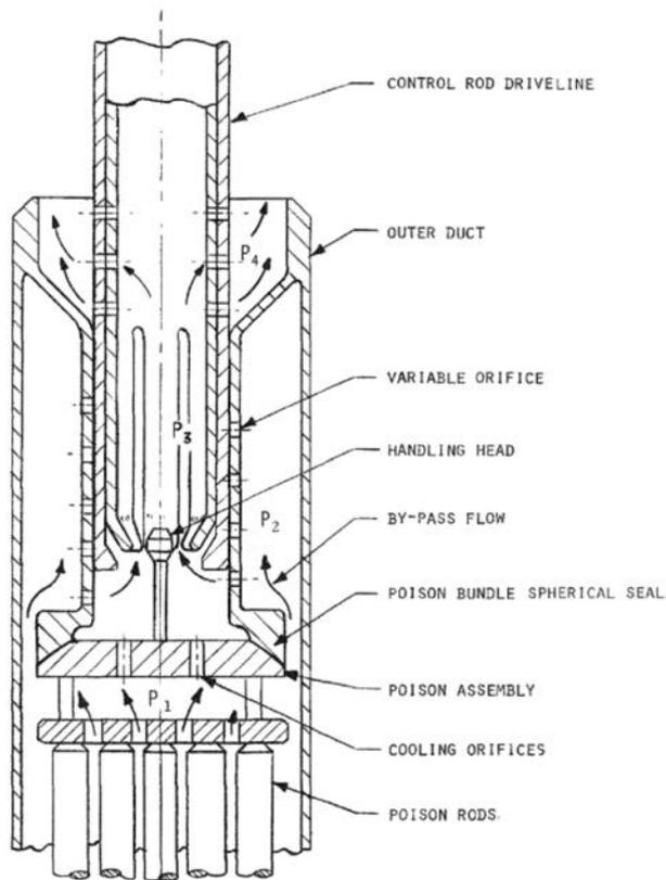
FIG. 42. Variable orifice concept allowing operation at various power levels [34].
