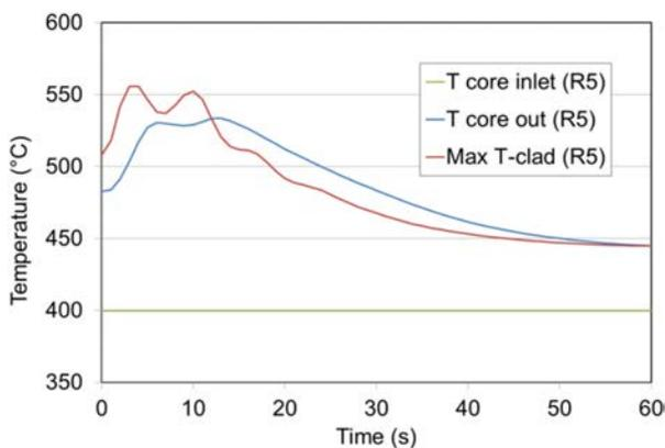
FIG. 80. Core inlet/outlet and maximum cladding temperatures (short term).
