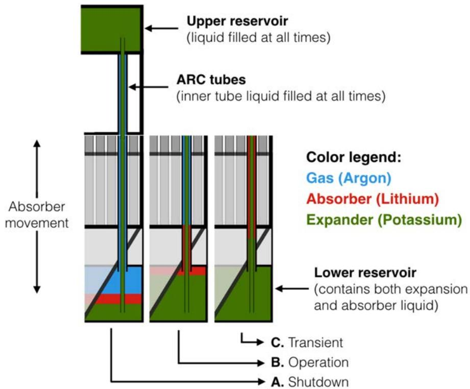
FIG. 18. Schematic view of the autonomous reactivity control system at different states/temperature (courtesy of S. Qvist, University of California, Berkeley).
