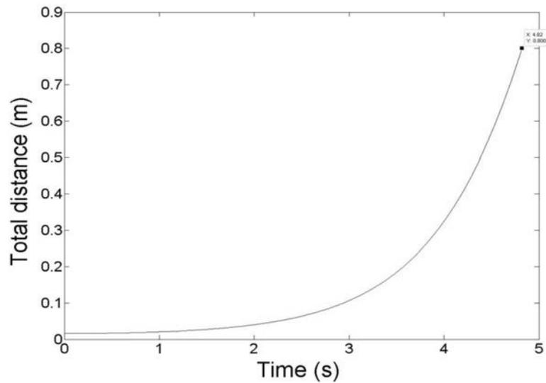
FIG. 58. Transient flow of liquid until it covers the siphon pipe length.
