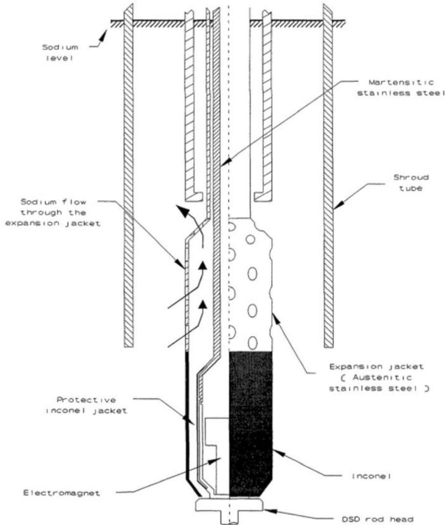
FIG. 51. The European fast reactor third shutdown concept (reproduced from Ref. [42]).
