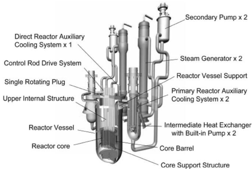
FIG. 90. Japan Sodium Cooled Fast Reactor [12].
