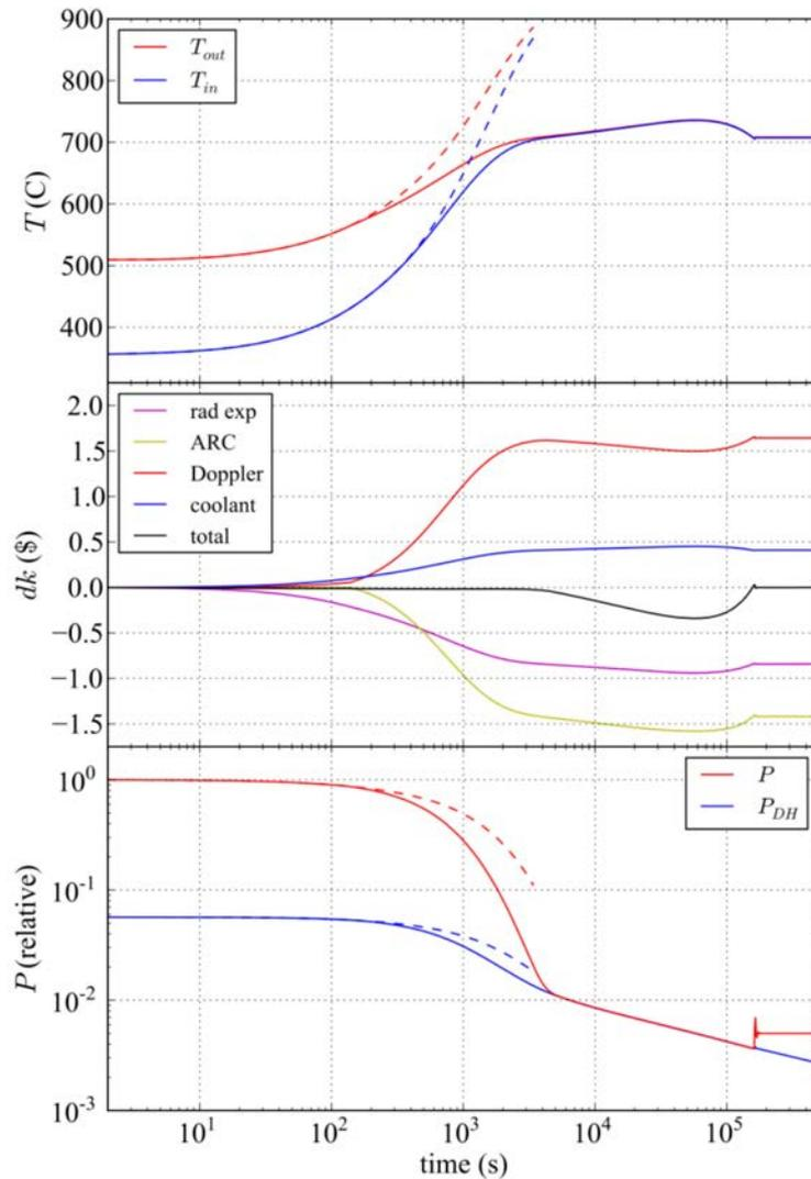
FIG. 76. Unprotected loss of heat sink simulation results. Upper panel: coolant temperatures (dotted lines are without autonomous reactivity control systems installed); middle panel: reactivity components; lower panel: power (total and decay) and flow rate.
