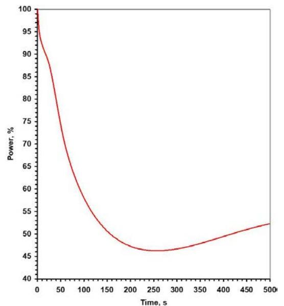
FIG. 70. Reactor power during one primary sodium pump seizure event without safety action.
