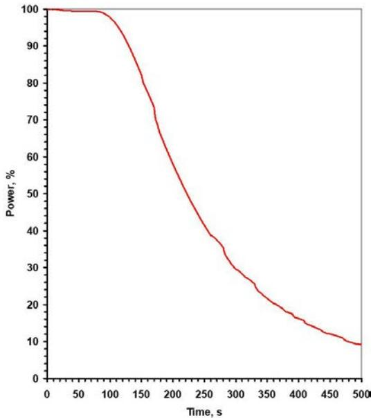
FIG. 73. Reactor power during loss of feedwater without safety action.
