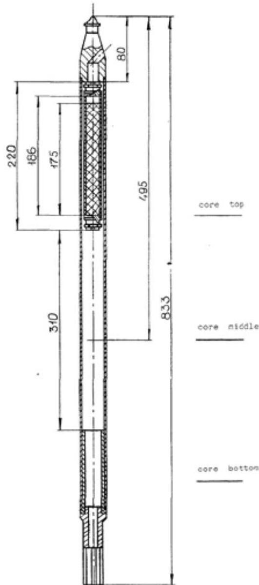
FIG. 28. Passive shutdown system subassembly with hydraulically suspended rod for the BR-10 reactor (reproduced from Ref. [29]).
