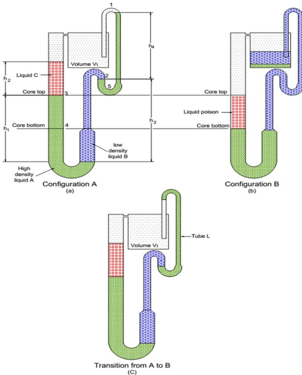
FIG. 21. Stages of the thermo siphon concept: (a) initial configuration, (b) final configuration, and (c) transition from initial to final configuration (courtesy of V. Raju, Indira Gandhi Centre for Atomic Research).
