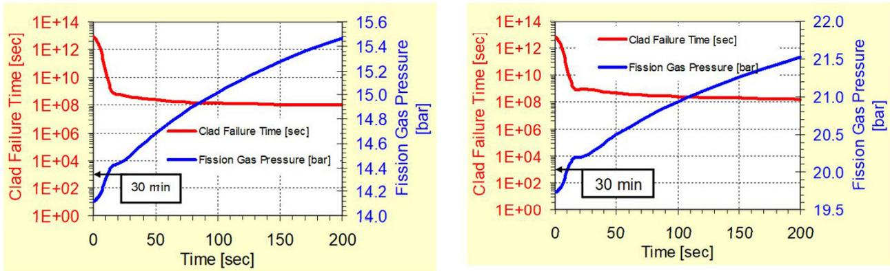
FIG. 89. Cladding failure time and peak pin fission gas pressure at beginning of cycle (left) and end of cycle (right) core conditions.
