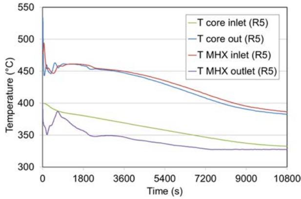
FIG. 82. Core inlet/outlet and main heat exchanger (MHX) inlet/outlet temperatures (long term).
