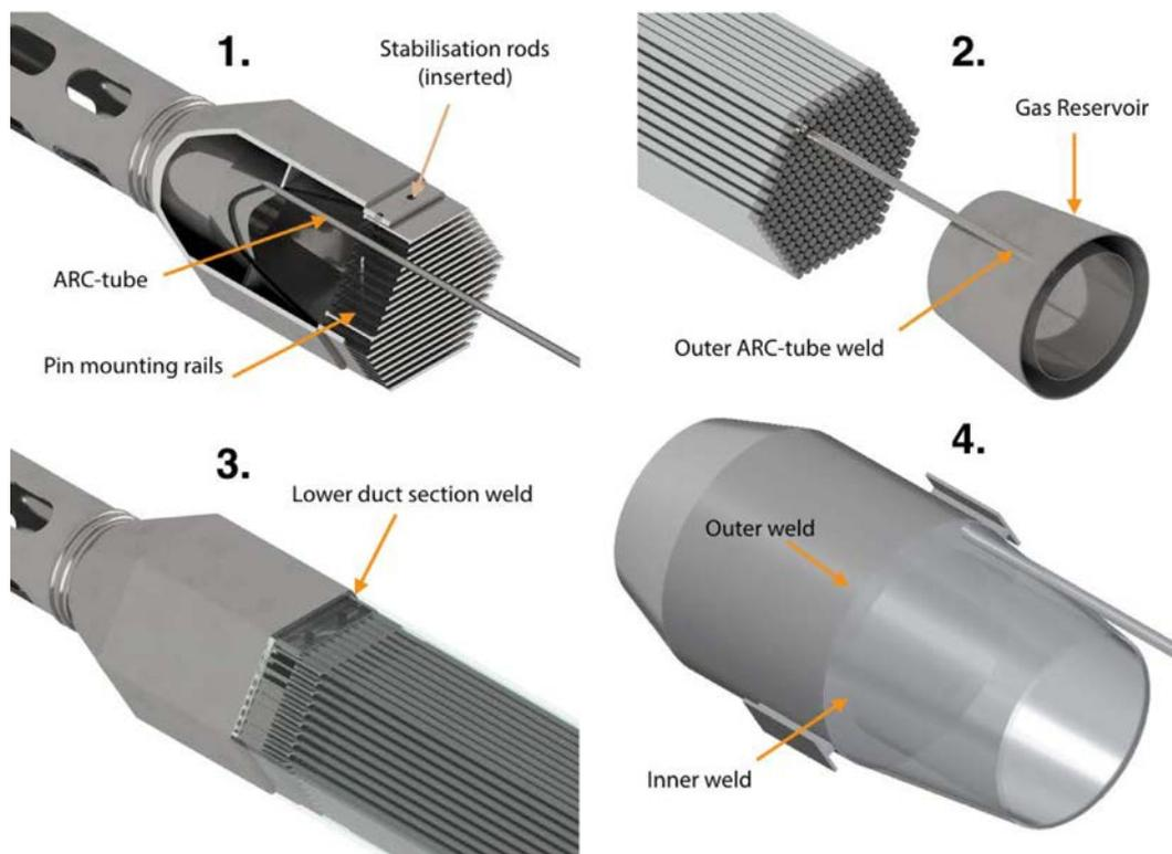
FIG. 55. Main assembling steps of a fuel assembly equipped with autonomous reactivity control (courtesy of S. Qvist, University of California, Berkeley).
