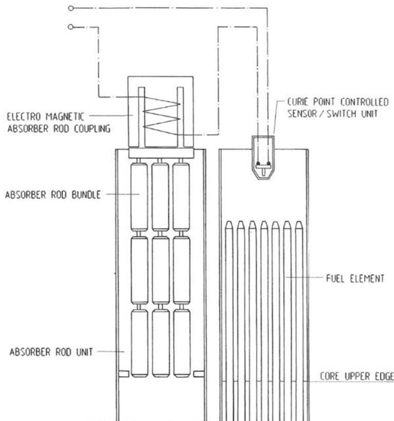
FIG. 37. Temperature sensitive inherent reactor shutdown system [30].
