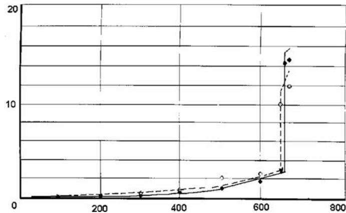
FIG. 7. Lengthening of passive shutdown system aluminium and magnesium as temperature rises: O — aluminium (experiment, calculation); ● — magnesium (experiment, calculation) (reproduced from Ref. [15]).
