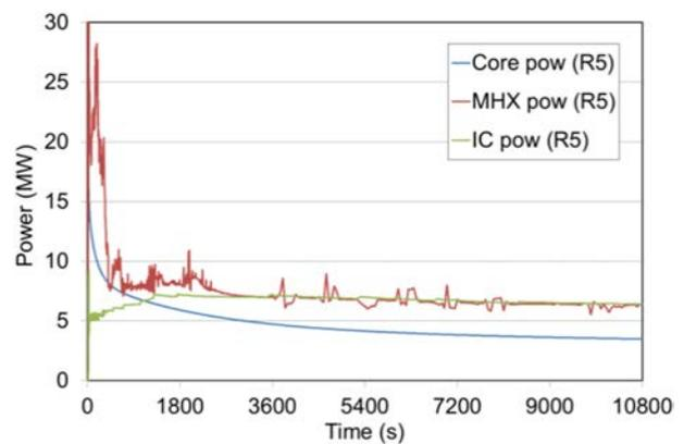
FIG. 81. Core, main heat exchanger (MHX) and isolation condenser (IC) powers (long term).
