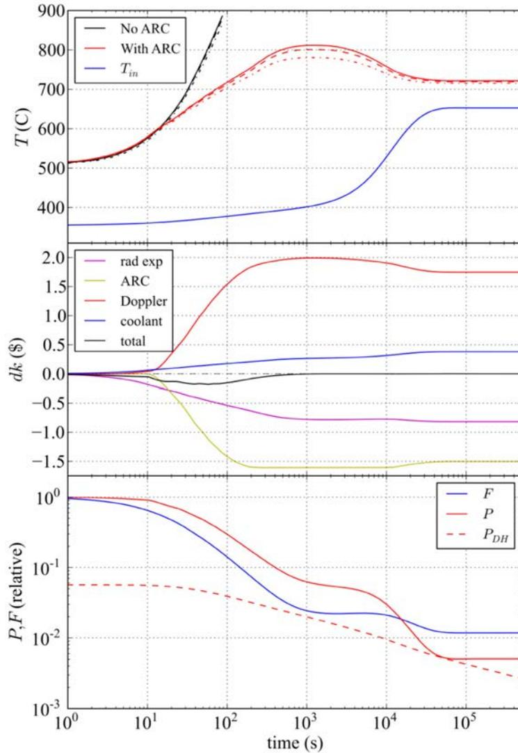
FIG. 77. Station blackout simulation results. Upper panel: coolant temperatures (the three red lines correspond to the three separate channels); middle panel: reactivity components; lower panel: power and flow rate.
