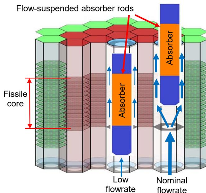
FIG. 9. Passive shutdown system with flow levitated rods for BN-800 (adapted from Ref. [18]).
