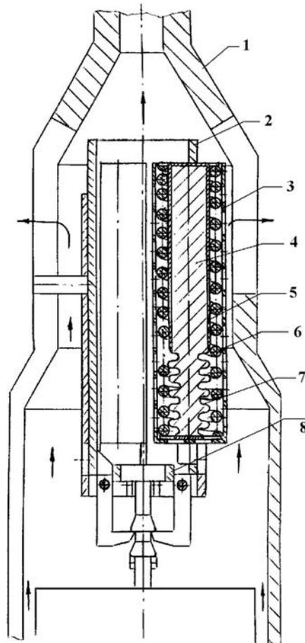
FIG. 6. The passive shutdown system with three sylphon working elements (reproduced from Ref. [15]): (1) head of a core assembly of passive type; (2) movable bush; (3) movable cylinder; (4) working medium; (5) container; (6) high temperature spring; (7) sylphon; (8) stop ring.
