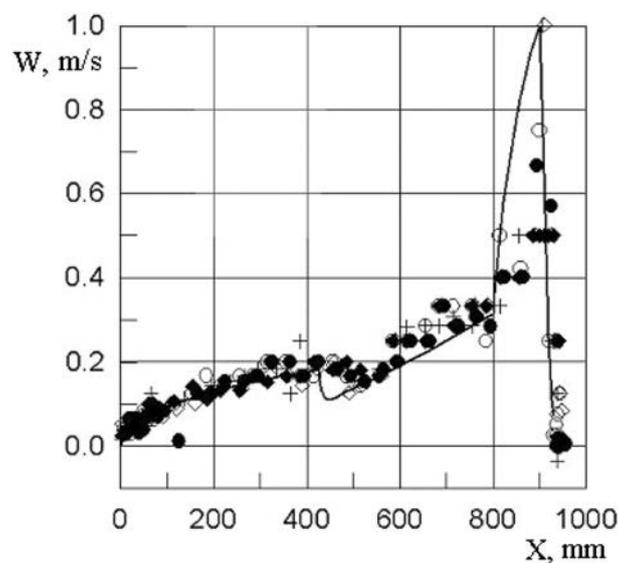
FIG. 27. Fall velocity variation of a rod in passive accident protection assembly as a function of distance (from its actuation point) in a regime cloning a rundown of main circulation pump 1 of the BN-600 reactor (reproduced from Ref. [15]).
