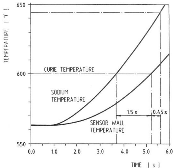
FIG. 40. Sensor wall temperature in the SNR-2 reactor during a loss of flow accident [30].
