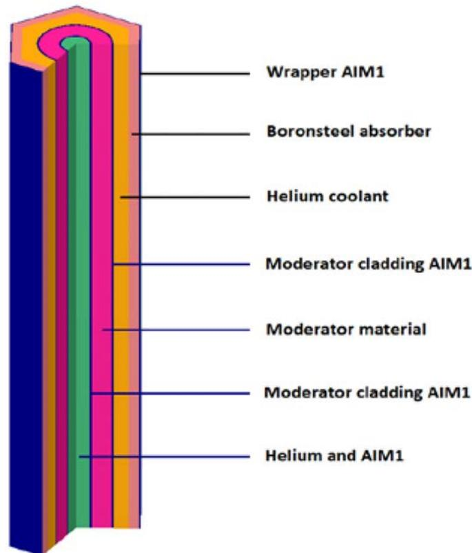
FIG. 45. Schematic for the neutron trap for application in gas cooled fast reactors [38].
