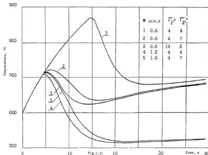
FIG. 30. Sodium temperature at the core outlet as a function of time since the onset of an accident (reproduced from Ref. [29]).
