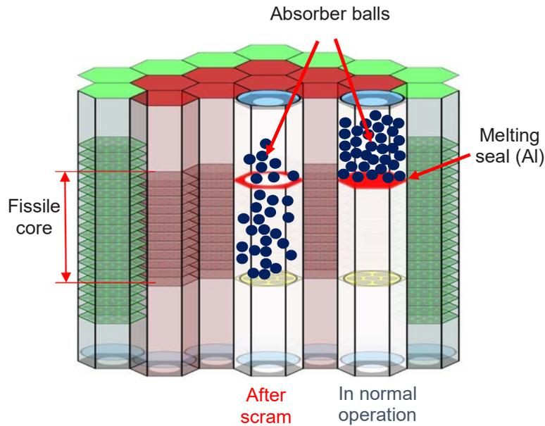
FIG. 13. Concept for a secondary scram system using absorber balls and an aluminium melt seal.
