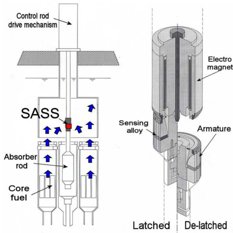
FIG. 4. Self-actuated shutdown systems concept (reproduced from Ref. [12]).
