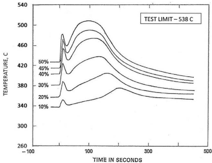
FIG. 25. Temperatures measured at the outlet of assembly row 2 during an unprotected loss of flow sequence initiated at different initial core power levels with nine gas expansion modules located at the core periphery of the fast flux test facility (courtesy of D. Wootan, Pacific Northwest National Laboratory).
