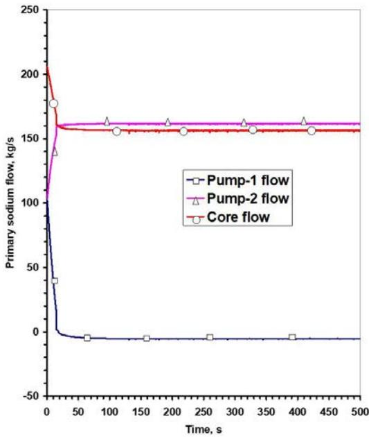
FIG. 67. Primary sodium flows during one primary sodium pump trip event without safety action.
