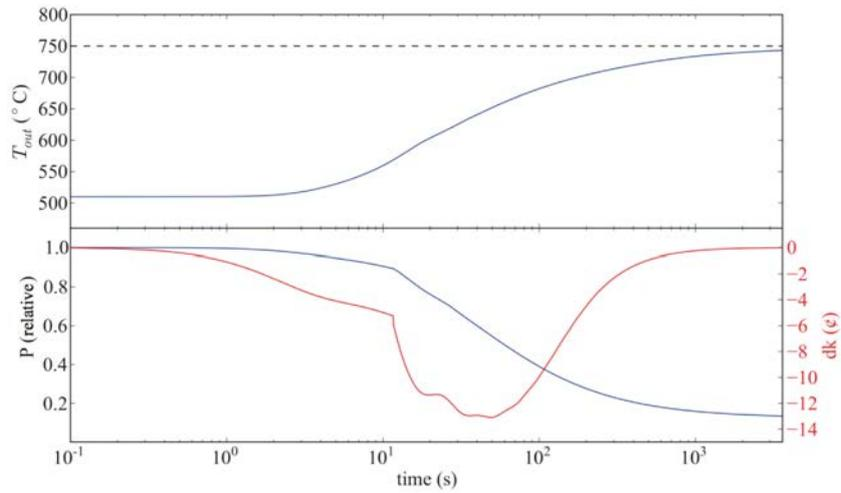
FIG. 75. Advanced Burner Reactor unprotected loss of flow quasi-static temperature prediction and transient simulation results. Upper panel: mean coolant outlet temperature (dotted black line: quasi-static prediction); lower panel: power and net reactivity. Note the discontinuity in the reactivity after about  $10^1$  s, which is due to the ARC system being engaged.
