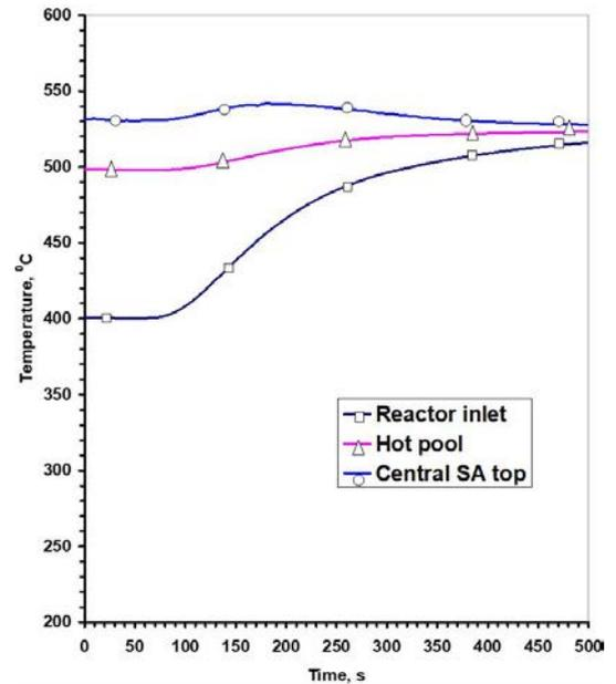
FIG. 74. Primary circuit temperatures during loss of feedwater flow event without safety action.
