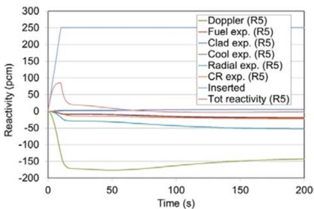
FIG. 87. Total reactivity and feedbacks.
