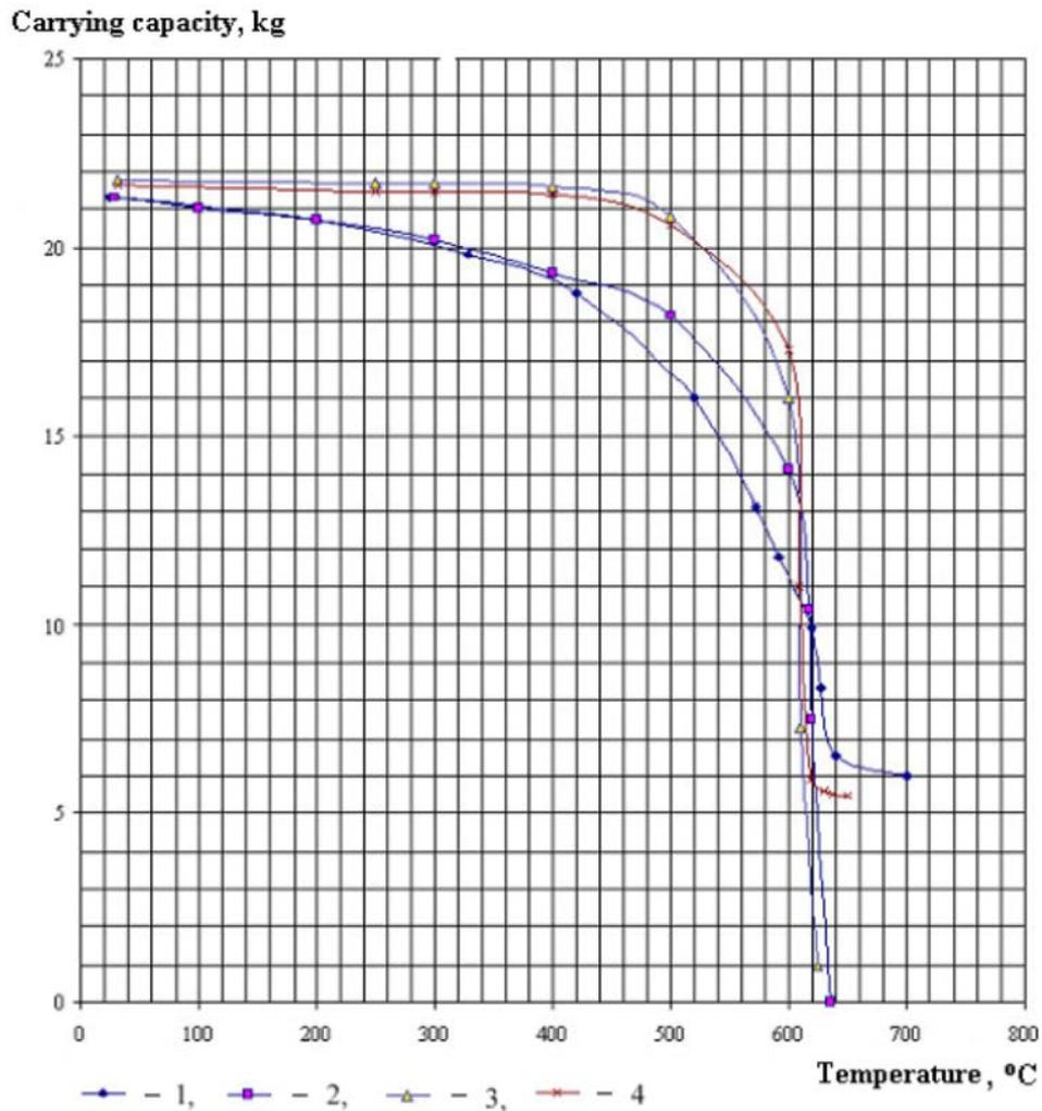
FIG. 35. Carrying capacity as a function of temperature for various samples (reproduced from Ref. [15]): (1) screen material — Fe–65Ni, armature material — St.3; (2) screen material — Fe–65Ni, armature material — Fe–65Ni; (3) screen material — Fe–67Ni–Co, armature material — Fe–67Ni–Co; (4) screen material — Fe–67Ni–Co, armature material — St.3.
