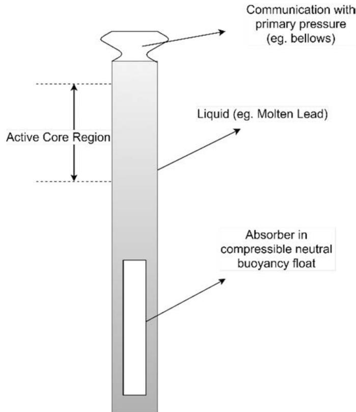
FIG. 10. Cartesian diver reactivity feedback device (adapted from Ref. [20]).
