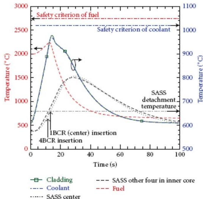
FIG. 93. Loss of flow without scram with passive shutdown [73].
