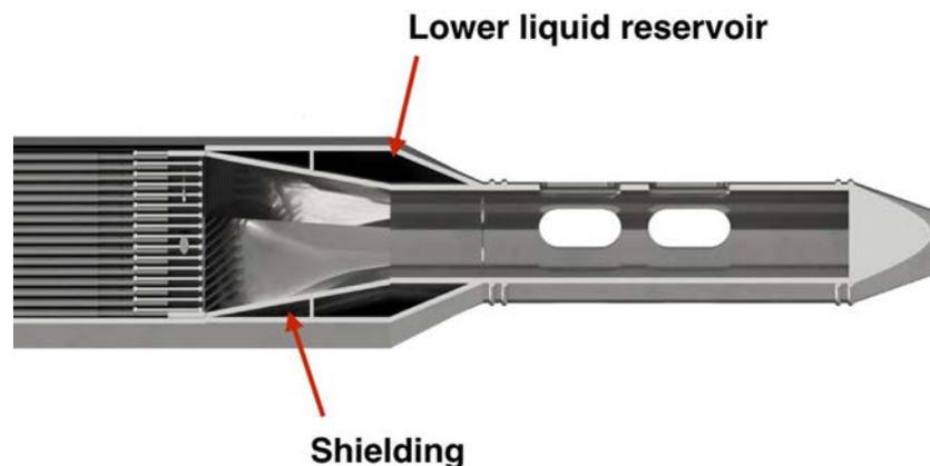
FIG. 53. Foot of a fast reactor fuel assembly with a lower autonomous reactivity control reservoir (courtesy of S. Qvist, University of California, Berkeley).
