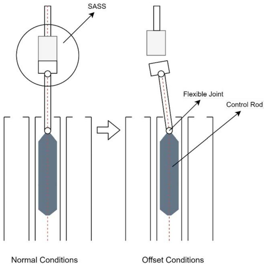
FIG. 92. A self-actuated shutdown system with a flexible joint (adapted from Ref. [73]).
