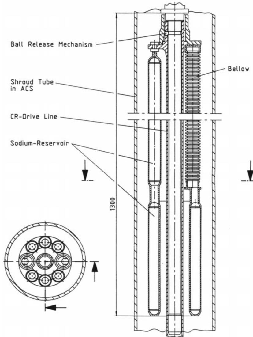
FIG. 50. The ATHENA technical design (reproduced from Ref. [41]).
