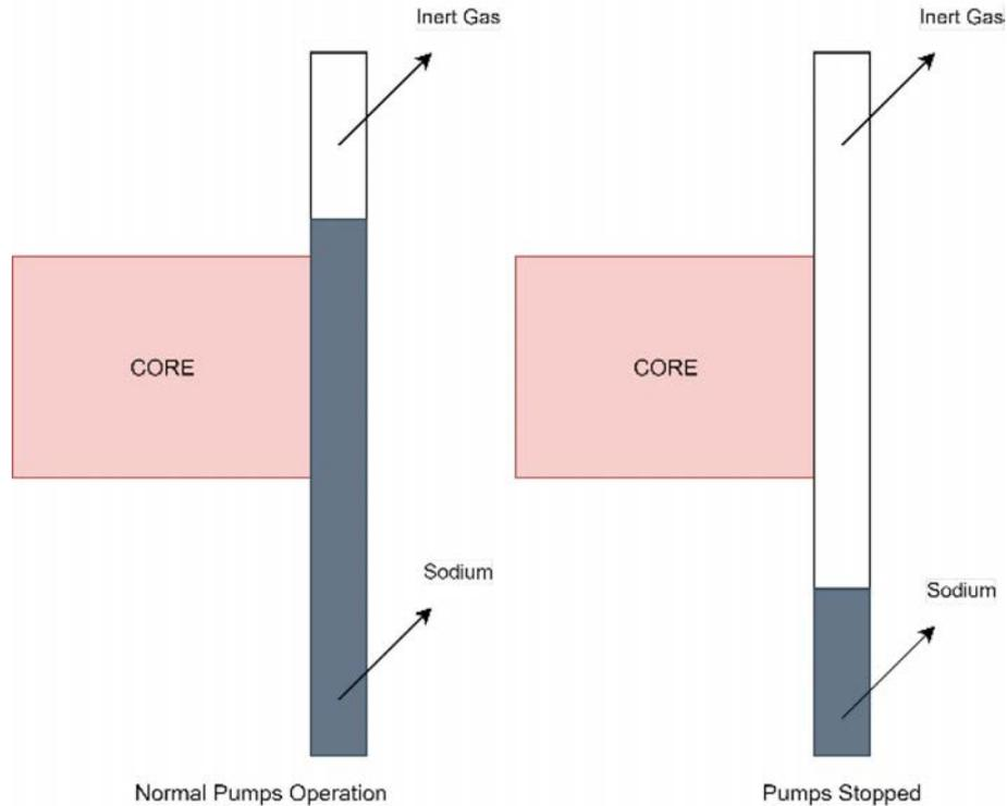
FIG. 17. Gas expansion module design concept.
