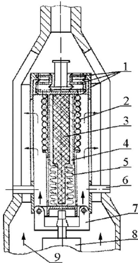
FIG. 36. Passive shutdown system operating on the basis of magnetic memory shape and on other physical effects (reproduced from Ref. [15]): (1) springs with magnetic memory shape; (2) high temperature spring; (3) capillary porous material; (4) temperature sensitive substance; (5) syphon; (6) support; (7) trigger mechanism; (8) absorber of neutrons; (9) coolant.
