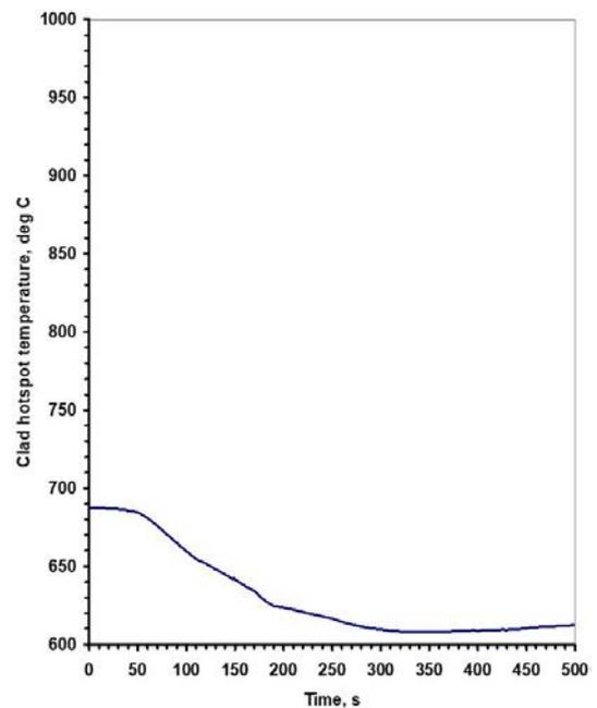
FIG. 72. Cladding hotspot temperature during one secondary sodium pump trip event without safety action.
