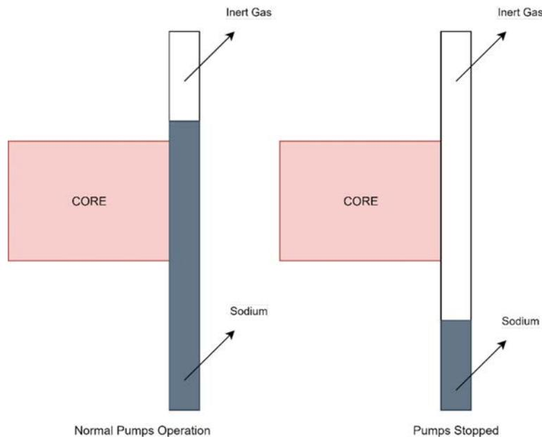
FIG. 44. Design concept of a gas expansion module [35].
