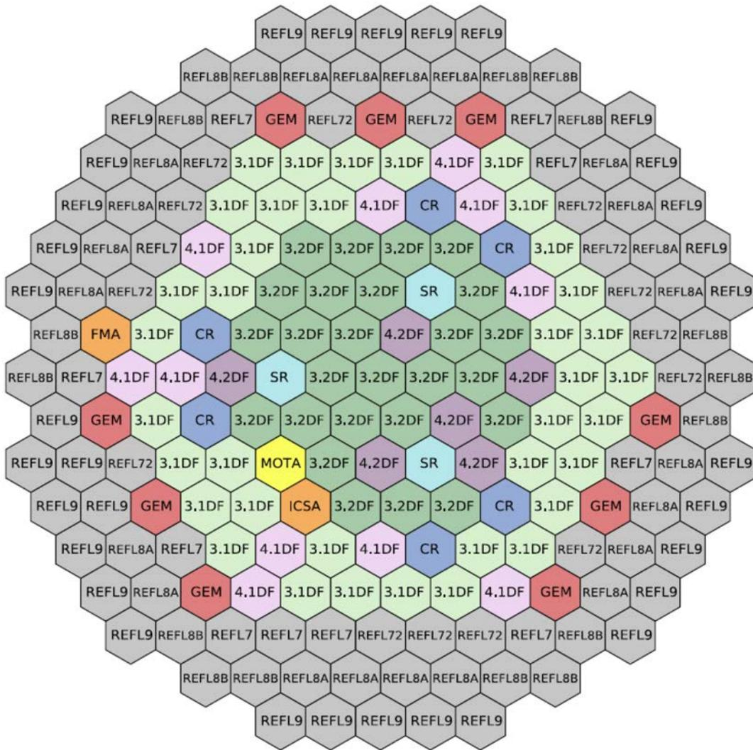
FIG. 24. Locations of gas expansion modules in the core of a fast flux test facility (courtesy of D. Wootan, Pacific Northwest National Laboratory).
