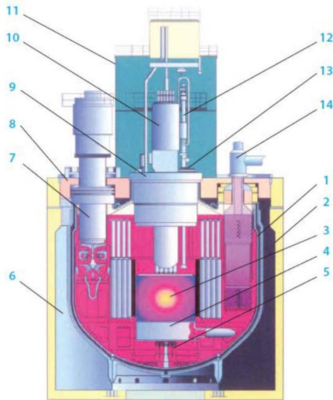
FIG. 32. BN-800 reactor components (courtesy of ROSATOM): (1) reactor pressure vessel; (2) guard tank; (3) reactor core; (4) pressure chamber; (5) corium catcher; (6) reactor cavity; (7) reactor coolant pump; (8) fixed upper shield; (9) large rotating cover; (10) central rotating cover; (11) protected hood; (12) reloading device; (13) small rotating cover; (14) intermediate heat exchanger.
