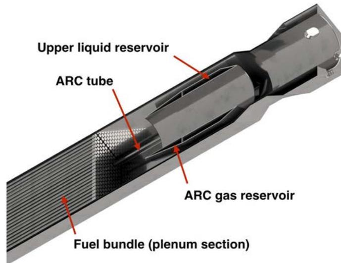
FIG. 54. Top of fast reactor fuel assembly with upper autonomous reactivity control reservoir (courtesy of S. Qvist, University of California, Berkeley).
