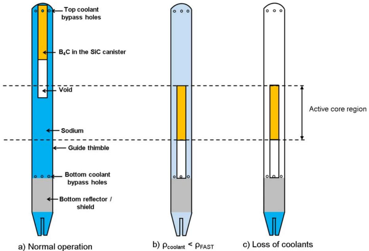
FIG. 62. Positions of a floating absorber for safety at transient device in several reactor conditions.
