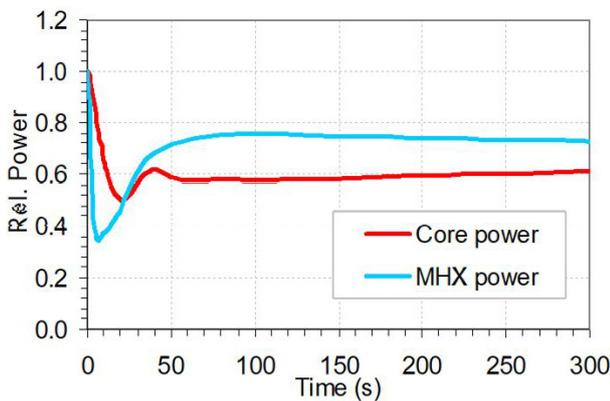
FIG. 85. Core and main heat exchanger (MHX) powers.
