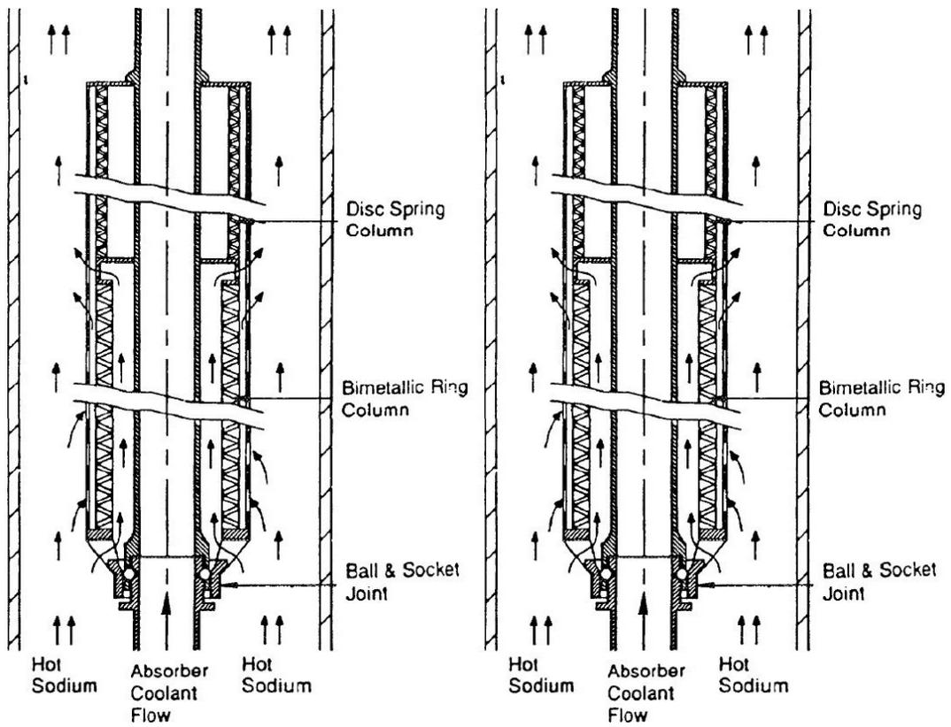
FIG. 15. Enhanced thermal expansion bimetallic ring concept (reproduced from Ref. [18]).
