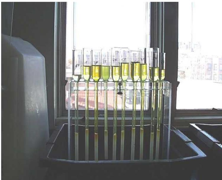
*FIG. 14. Chromatography columns for purification of zinc from other minerals in digested samples.*
