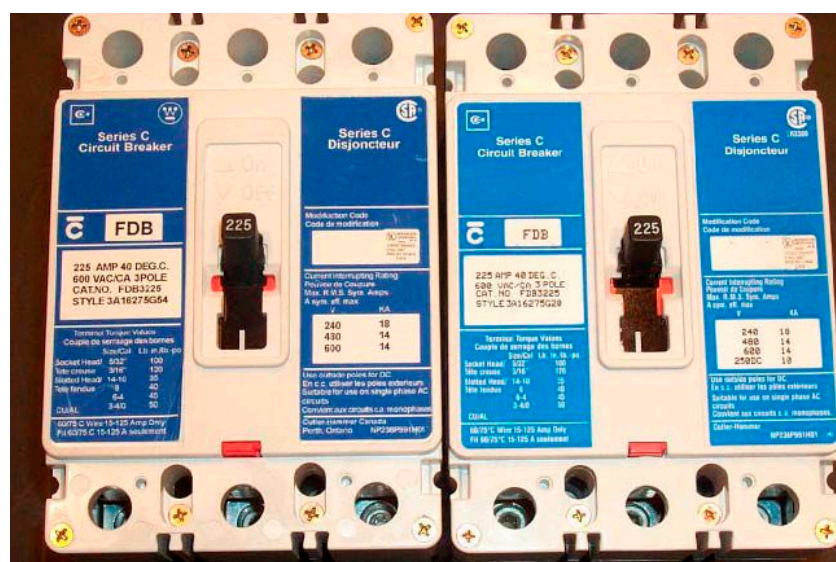
FIG. 3. Counterfeit (left) and legitimate breaker (right) supplied to a hospital in Montreal, Canada. (Reproduced from Ref. [11] with permission courtesy of Canadian Standards Association Group Inc.)
