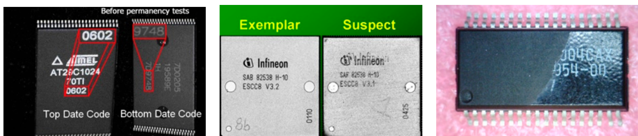
FIG. 9. Electronic counterfeit examples (left: date code changes; centre: tampering detected via acoustic microscope; right: blacktopping detected by heated solvent test). (Courtesy of SMT Corp.)
