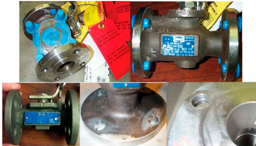
FIG. 4. Flanges received as 'new' at Savannah River, South Carolina. Note clamp marks and different rivet sizes. (Reproduced from Ref. [10] with permission courtesy of US Department of Energy.)
