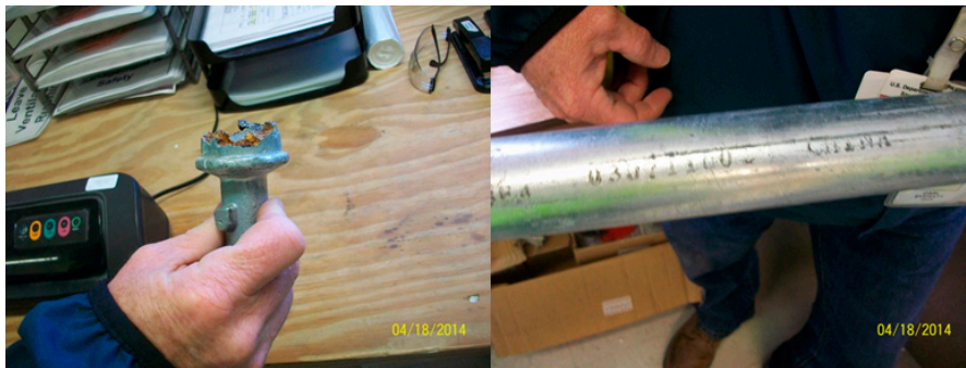
FIG. 24. Suspected fraudulent scaffolding. (Courtesy of US Department of Energy.)
