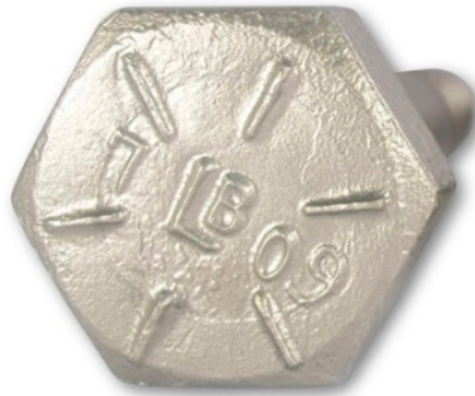
FIG. 2. Typical bolt-head marking indicating capability (the six lines indicate a Society of Automotive Engineers grade 8 bolt) and the manufacturer (manufacturer code for the Lewis Bolt & Nut Company). (Courtesy of Lewis Bolt & Nut Company.)
