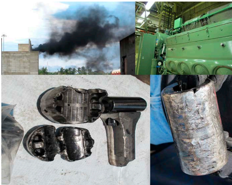
FIG. 25. Laguna Verde emergency diesel generator 3 failure. (Reproduced from Ref. [75] with permission courtesy of Comisión Federal de Electricidad.)
