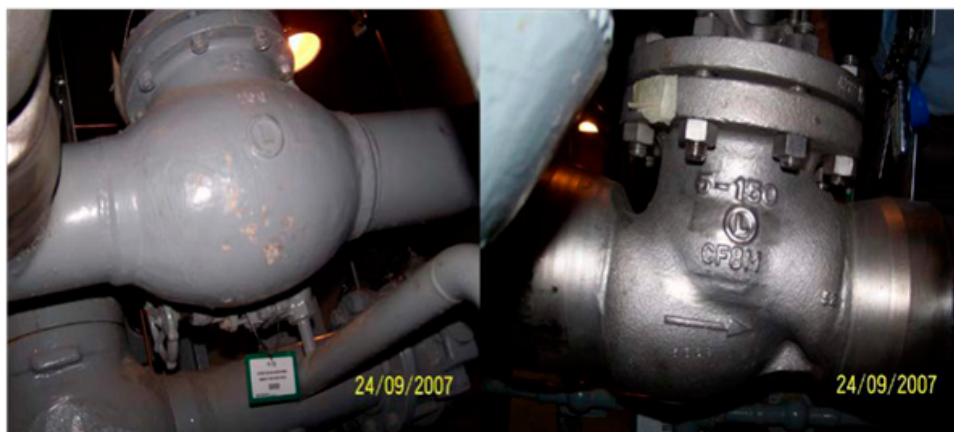
FIG. 22. Genuine (left) and counterfeit (right) Ladish check valves. (Reproduced from Ref. [6] with permission courtesy of EPRI.)
