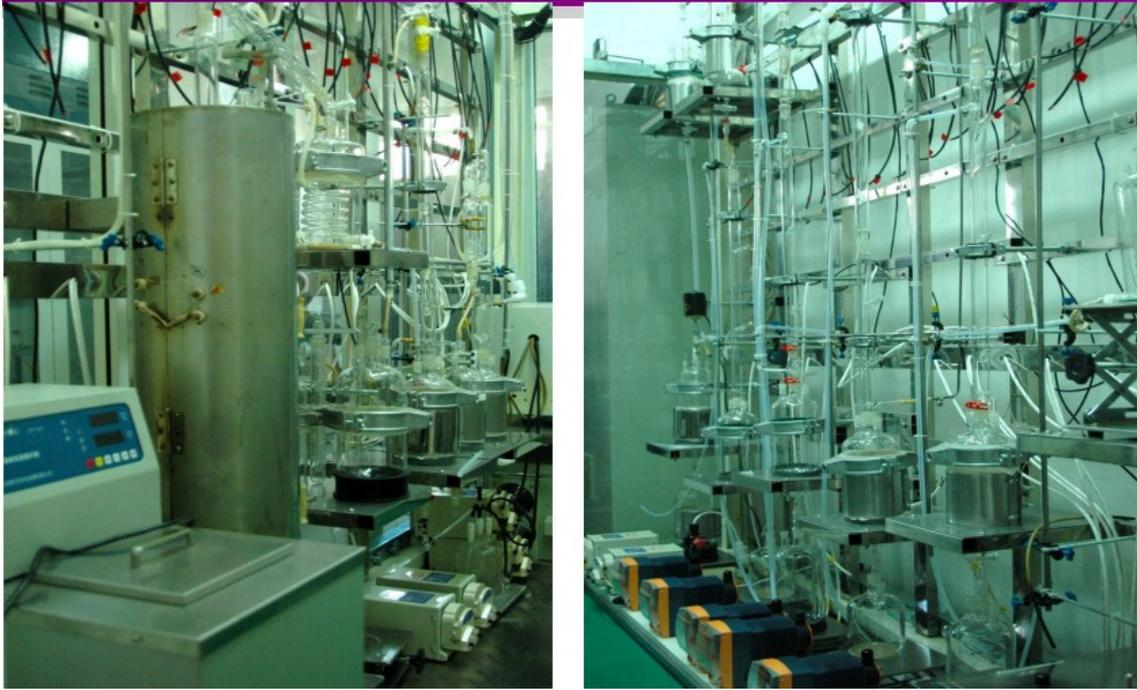
FIG. 18. Proof of concept experimental facility of the sulphur–iodine process at INET.
