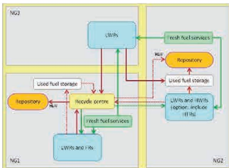
FIG. 15. Heterogeneous model with synergistic groups and specific reactor types and fuel services identified [3]. HTR — high temperature reactor; HWR — heavy water reactor; LWR — light water reactor; MNA — multilateral nuclear approach.
