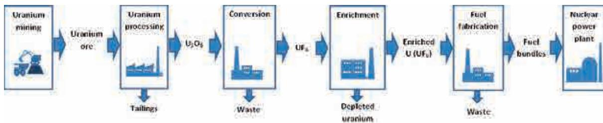
FIG. 25. Fuel production chain for a light water reactor using uranium fuel in an open fuel cycle.
