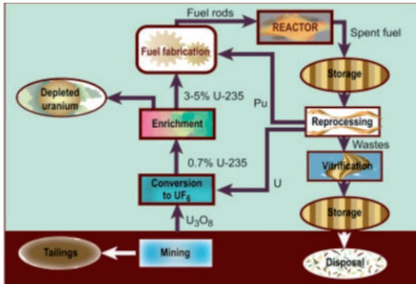
FIG. 7. Nuclear fuel cycle of a thermal reactor with recycling of uranium and plutonium [27].
