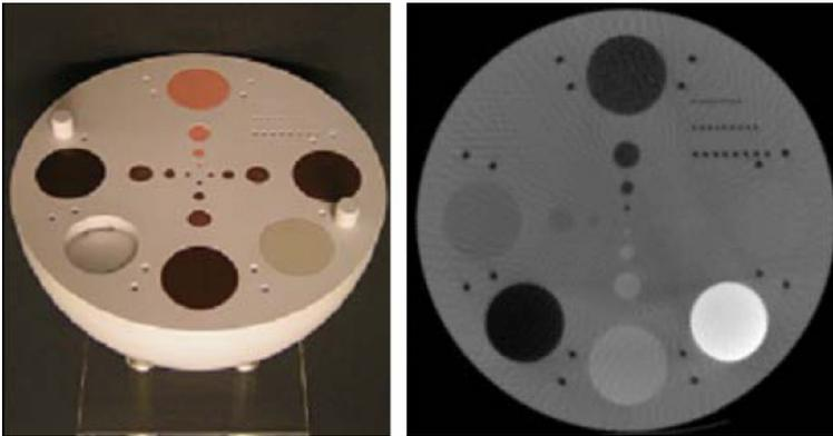
FIG. 29. Picture of a phantom used for image quality optimization (left) and an axial CT image of the phantom (right). (Images courtesy of Siemens.)
