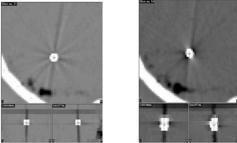
FIG. 28. (Left) An axial reconstruction of a 0.2 cm lead bead based on CT data from an anthropomorphic phantom using a sequential scanning mode with a slice thickness and feed of 0.2 cm. (Right) A similar axial reconstruction of the same lead bead using a helical scanning mode (slice and feed of 0.2 cm) illustrating the enlarged streaking artefact. (Images courtesy of D. Verellen.)
