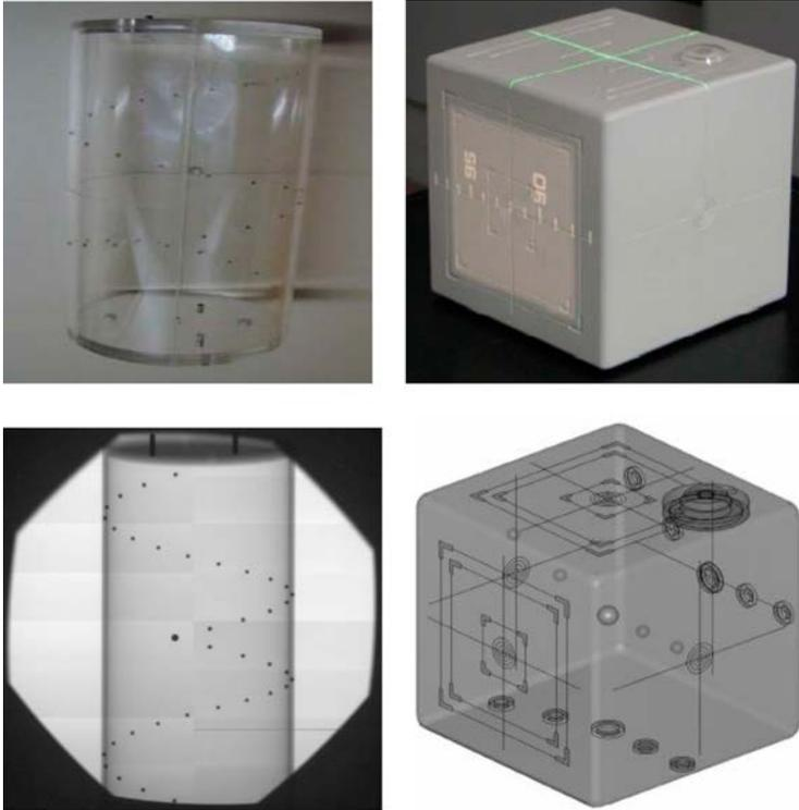
FIG. 27. Phantoms for 3-D geometrical calibration using known external features and interior structures. (Courtesy of U. Oelfke and J. P. Bissonnette.)
