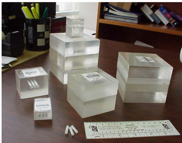
FIG. 43. IROC Houston irradiation phantoms for QA audit.
