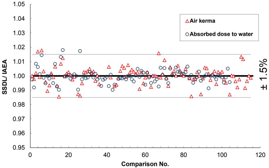
FIG. 20. Ratios of ionization chamber calibration coefficients supplied by the SSDLs to those measured by the IAEA in 1991–2012. Triangles correspond to air kerma for  $^{60}\text{Co}$  and circles correspond to absorbed dose to water coefficients.
