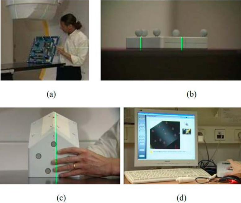
FIG. 33. An example of the calibration procedure for a target localization system: (a) Referencing video and IR system; (b) Calibrating IR system with respect to treatment isocentre using room lasers; (c) Phantom with IR reflective markers and radio-opaque imbedded markers; (d) Software tool to calibrate the X ray system with respect to the IR system referencing the IR markers and radio-opaque markers from the previous phantom. (Courtesy of D. Verellen.)
