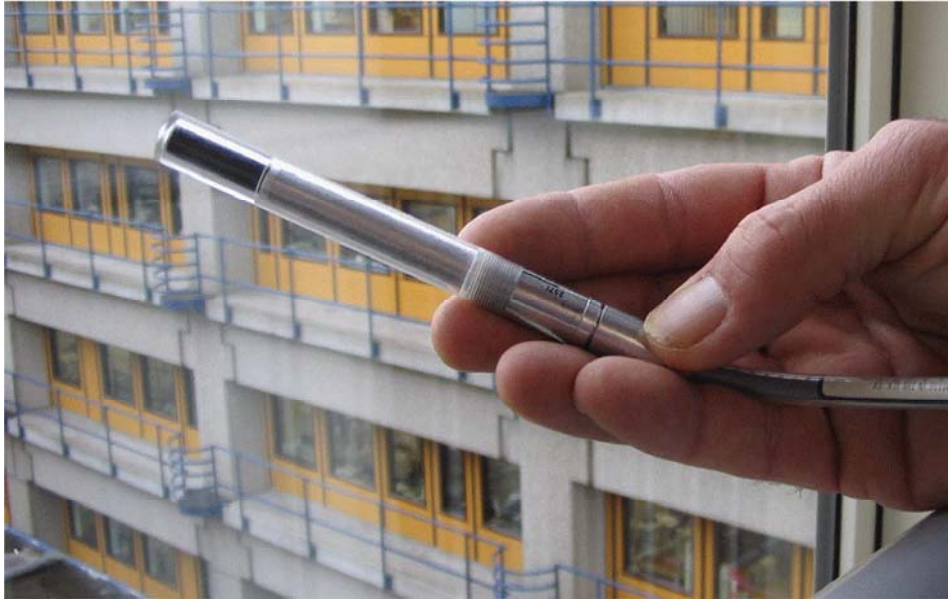
FIG. 14. Farmer chamber, as an example of a smaller ion chamber.
