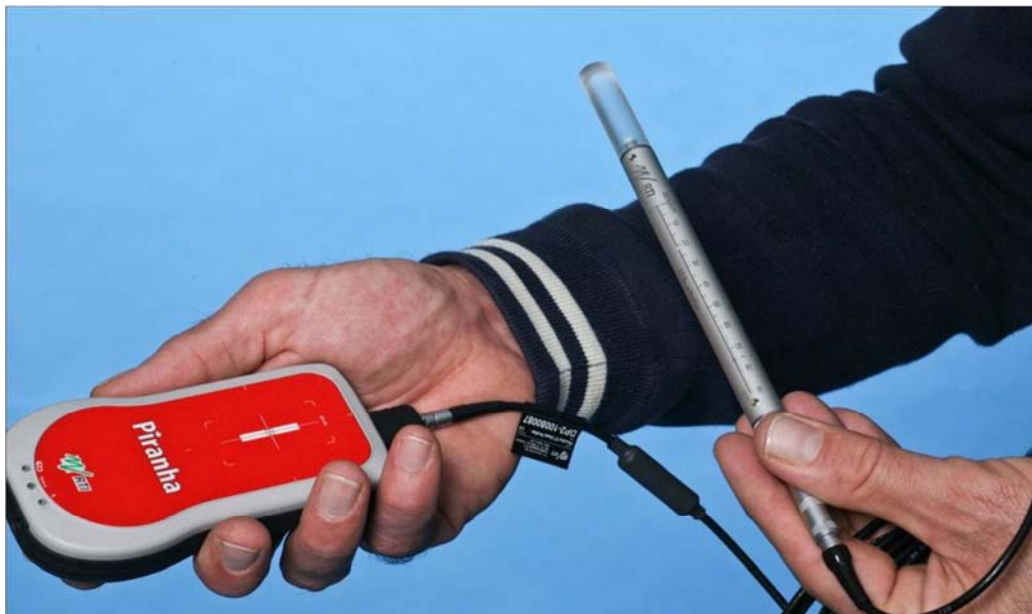
FIG.15. Small solid state detector with read unit.
