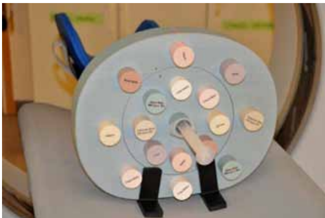
FIG. 1. The density phantom positioned on the CT scanner couch ready to be scanned.
