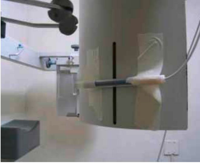
FIG. 3. Set up of CT pencil chamber.
