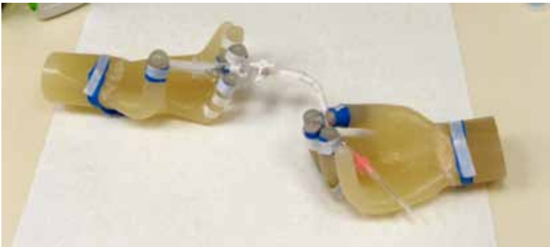
FIG. 4. Measurement of skin dose by pairs of TLDs MCP-7 and MCP-Ns on hands with an unshielded syringe (left) and with an infusion tube (right), both filled by ^{18}\text{F} -FDG.
