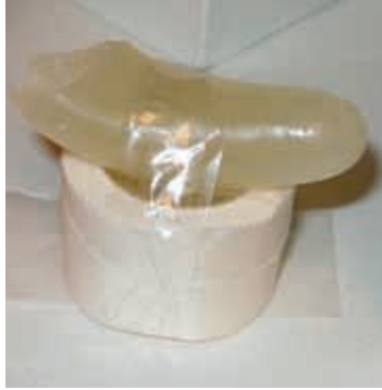
FIG. 1. Measurement of skin dose by pairs of TLDs MCP-7 and MCP-Ns placed on the finger phantom. The plane source of positron ^{18}\text{F} -FDG is at a distance of 2 cm under the finger.
