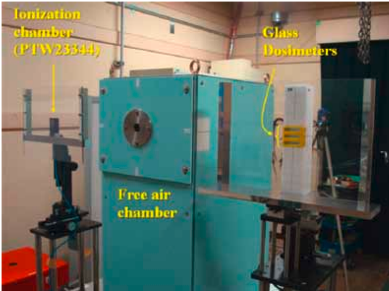
FIG. 4. Evaluation of glass dosimeters at the National Institute of Advanced Industrial Science and Technology (AIST).
