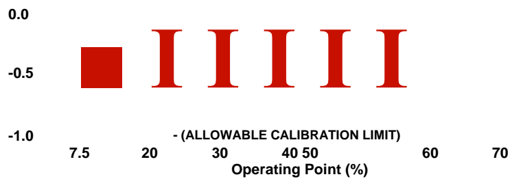
FIG. 7. On-Line Monitoring Results for Assessment of Calibration of a Pressure Transmitter as a Function of Pressure Range
