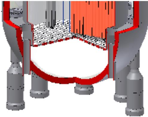
*Fig. 4. Bottom of the reactor vessel*
