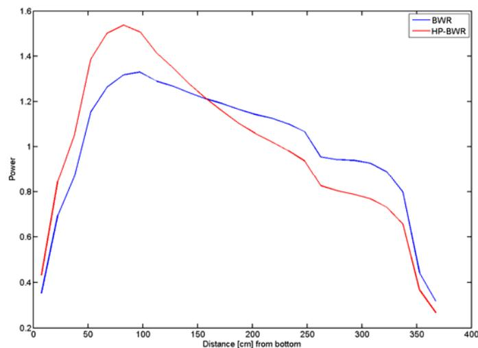
Fig. 5. Axial power distribution in HP-BWR and BWR, calculated with the RELAP5 (Mod3.3 Patch02) and PARCS codes
