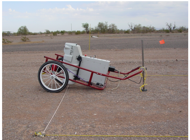
FIG. 4: PELAN on a cart used for the blind tests at Yuma Proving Ground.
