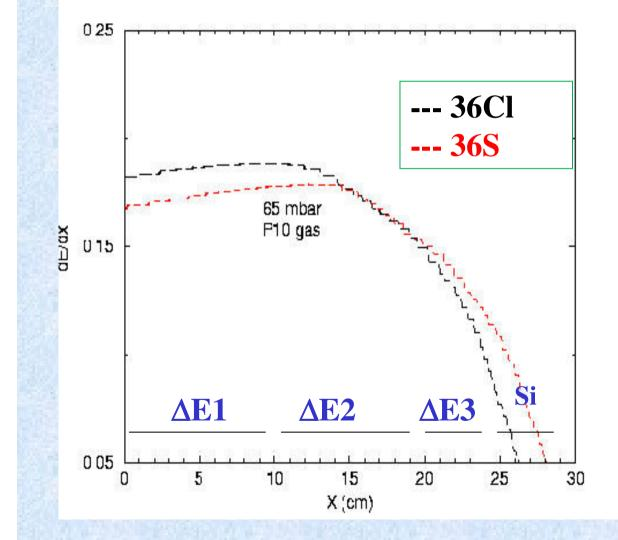
In  $\Delta E1$  &  $\Delta E2$ , signal height of  ${}^{36}Cl > {}^{36}S$ In  $\Delta E3$ , Eres, signal height of  ${}^{36}S > {}^{36}Cl$  ${}^{36}S$  background can be reduced by Factor 10<sup>4</sup>
