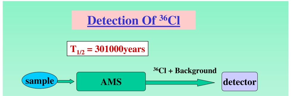
Accelerator based Mass Spectrometry (AMS) : ultra-sensitive means of counting individual atoms of long half life.
