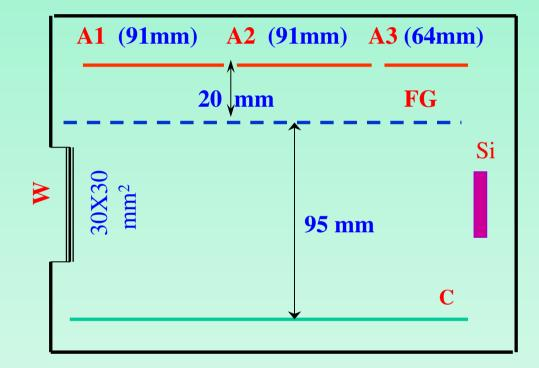
$V_{anode} = +150 V$   $V_{grid} = +63 V$   $V_{cathode} = -150 V$ Gas : P10 ( 52 torr flow mode) Window : Mylar (3.5 $\mu$ m) Si -Detector : 300 $\mu$ m
