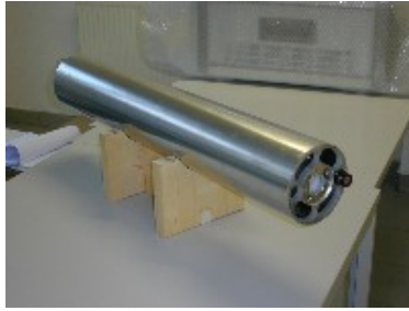
Fig. 2 Reaction chamber with cowling cover installed
