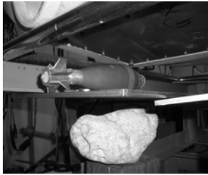
FIG. 3. The active grenade was measured in variety of geometries, here is shown above a rock. Results of the measurement, target in – target out under the same experimental conditions.
