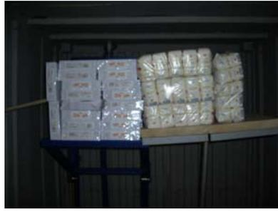
FIG. 4. Paper and flour targets in the container (tagged neutron beam traversed from right to left).
