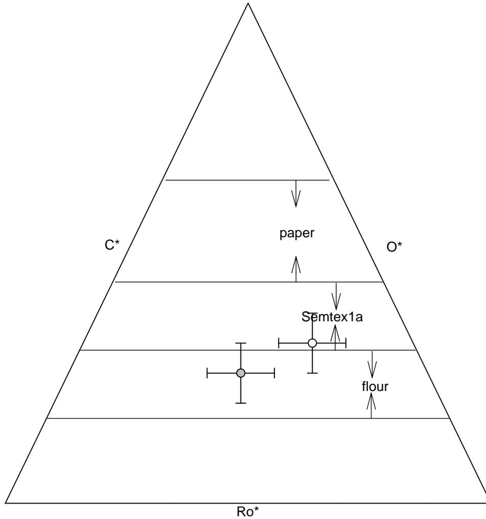
FIG. 6. Triangle diagram, flour (gray) and paper (white, paper misinterpreted as explosive).
