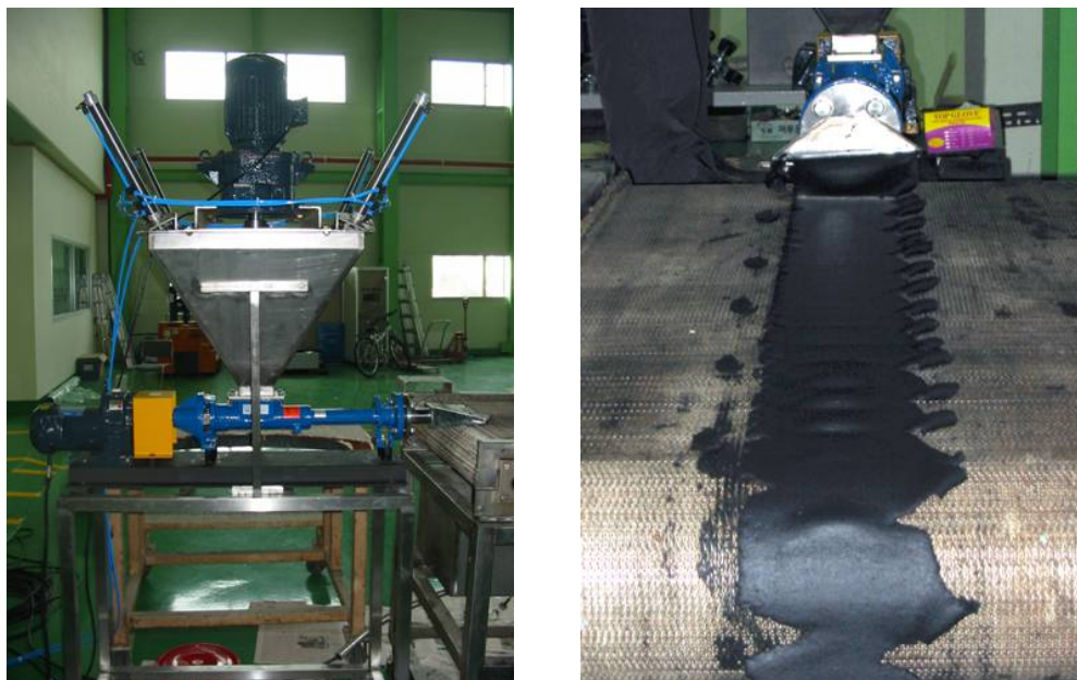
FIG. 2. Injection of sludge on the conveyor through nozzle
