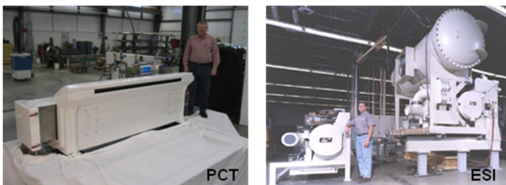
FIG. 3. Low-energy electron beam accelerators manufactured by PCT Engineered Systems, LLC (voltage: 70 to 125 keV and web widths: 914 to 1,727 mm) and Energy Sciences, Inc., ESI (web widths: 508 to 1,676 mm, speed capability: 335 m/min and thickness: 0.03 mm).
