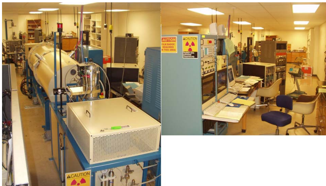
FIG 2. Photographs of the Hope College Ion Beam Analysis Laboratory. The 1.7MV tandem pelletron and alphasource ion source are visible on the left, while the control console and acquisition electronics are visible on the right. Note the absence of shielding walls due to the extra lead shielded installed during construction of the accelerator vessel.
