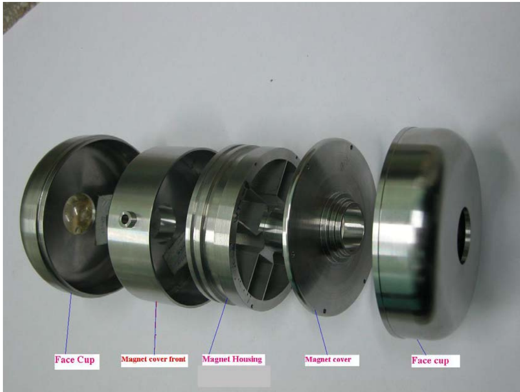
Fig-4 : Exploded view of the drift tubes
