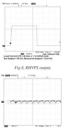
Fig. 9, Output voltage ripple.
