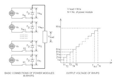
Fig. 1, Basic Scheme for PSM Based Accelerator Power Supply.
