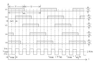
Fig. 2. Output Voltage with PSM and PWM for 5 SPMs.
