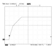
Fig. 10, Variable ramp start-up
