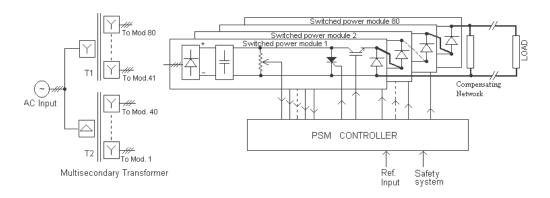
Fig. 3, Solid state high voltage power supply using PSM.
