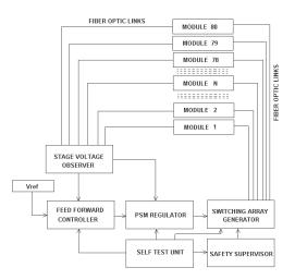
Fig. 4, Control System for Accelerator Power Supply.
