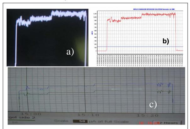
Figure 2.- a) Instantaneous and continuous exposure-rate monitoring, as displated on PC screen, from inside cyclotron's vault data during target irradiation. b) LabView plot display for collected data from LSMAM through SMARR network. c) Time dependent, both beam-on-target and stripper, intensities as a function of irradiation time as seen on IBA's INTOUCH screen.
