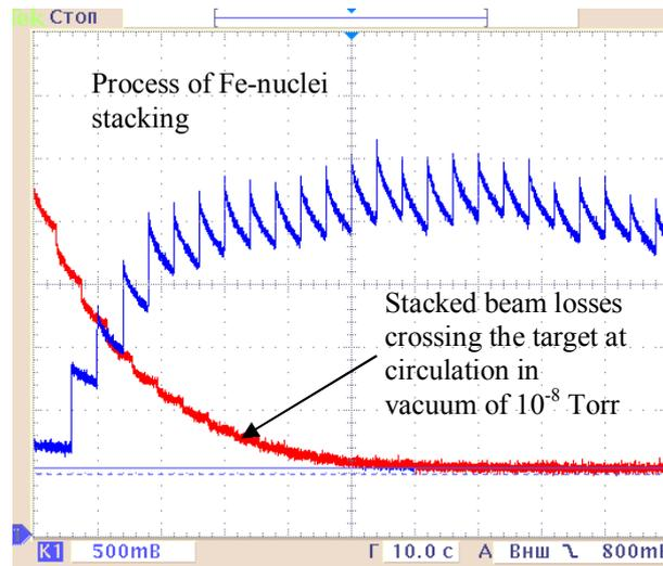
FIG. 7. Stacking of Fe<sup>26+</sup>-nuclei in the U-10 ring.
