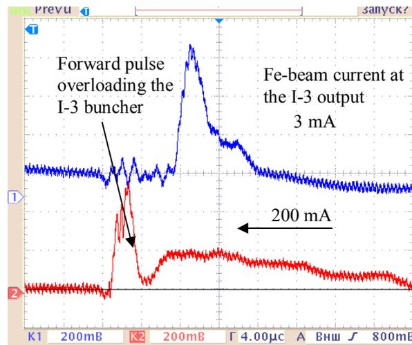
FIG. 6. Current signals of total Fe-beam at the LIS extraction gap outlet and  $\text{Fe}^{16+}$ -beam of 64 MeV at the I-3 linac output.
