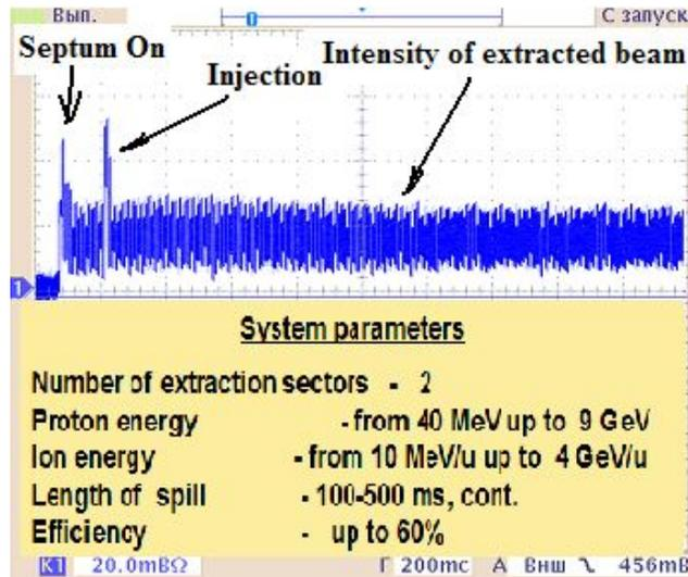
FIG. 3. Extraction carbon beam accelerated in the UK ring up to the energy of 200 MeV/u at repetition rate of 0.25 Hz using U10 ring as stretcher.
