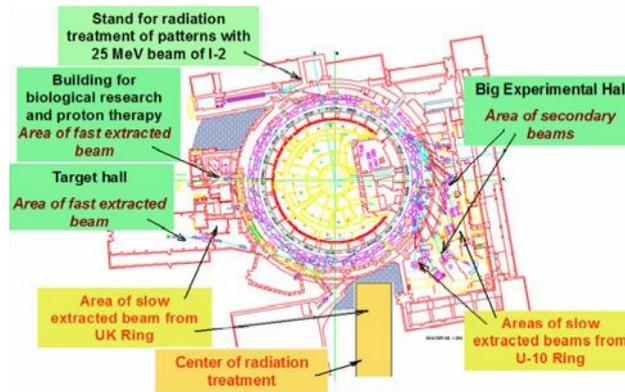
FIG. 1. Experimental area of ITEP-TWAC facility, green - in operation, yellow - in projecting.
