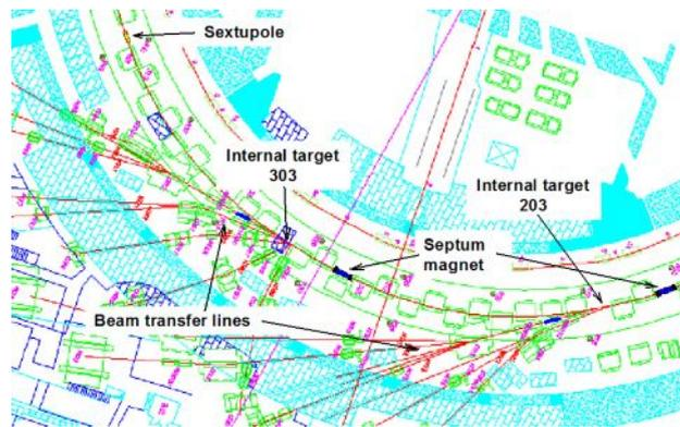
FIG. 2. Slow extraction system of U-10 ring.
