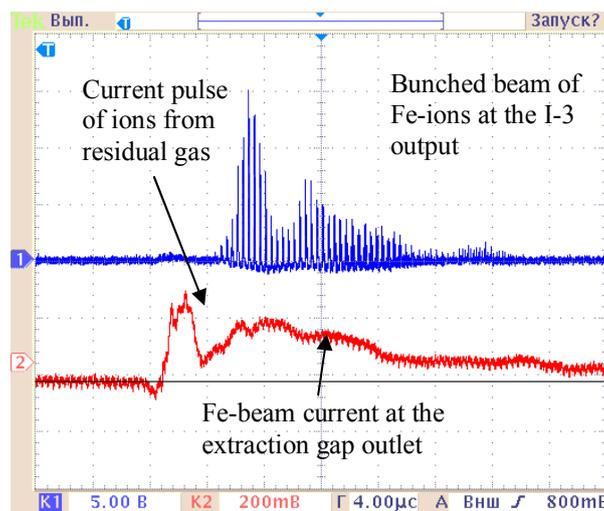
FIG. 4. Signals of Fe-ion beam generated in LIS.
