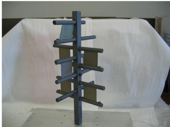
*FIG. 1. Sample holder for the CVD coater at PBMR (Pty) Ltd. Substrates of commercial polycrystalline silicon carbide wafers are mounted in grooves between the horizontal rods.*
