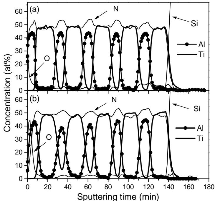
FIG. 2. XPS depth profiles of  $(\text{AlN/TiN})_{x5}/\text{Si}$ : (a) as-deposited sample; (b) sample implanted with argon to  $4 \times 10^{16}$  ions/cm<sup>2</sup>.
