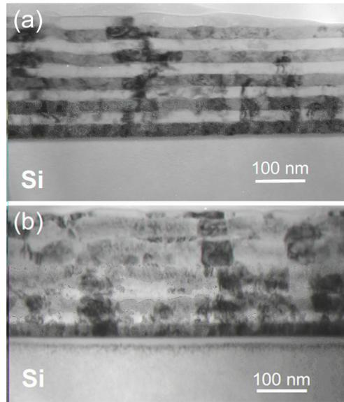
FIG. 6. Bright field cross-sectional TEM images of: (a) as-deposited  $(Al/Ti)_x5/Si$ ; (b)  $(Al/Ti)_x5/Si$  implanted with argon to  $4 \times 10^{16}$  ions/cm<sup>2</sup>.
