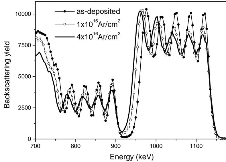
FIG. 3. Experimental RBS spectra from an as-deposited (Al/Ti)<sub>x</sub>5/Si sample, and samples implanted to  $1 \times 10^{16}$  ions/cm<sup>2</sup> and  $4 \times 10^{16}$  ions/cm<sup>2</sup>.
