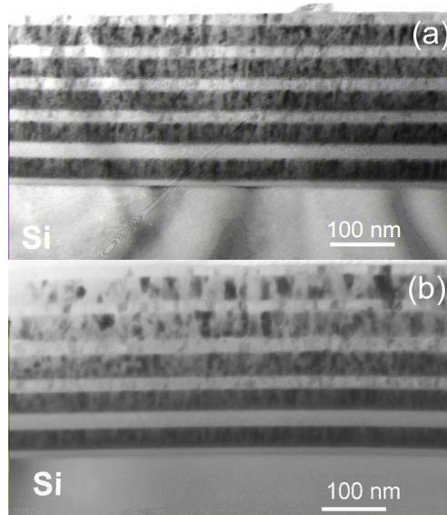
FIG. 5. Bright field cross-sectional TEM images of: (a) as-deposited (AlN/TiN)<sub>x5</sub>/Si; (b) (AlN/TiN)<sub>x5</sub>/Si implanted with argon to  $4 \times 10^{16}$  ions/cm<sup>2</sup>.
