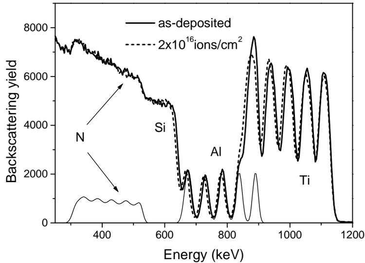
FIG. 1. Experimental RBS spectra from an as-deposited  $(\text{AlN/TiN})_{x5}/\text{Si}$  sample, and a sample implanted to  $2 \times 10^{16}$  ions/cm<sup>2</sup>.
