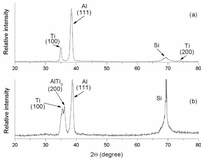
FIG. 4. XRD analysis of (Al/Ti)<sub>x</sub>5/Si samples: (a) as-deposited, and (b) sample implanted with argon to  $4 \times 10^{16}$  ions/cm<sup>2</sup>.
