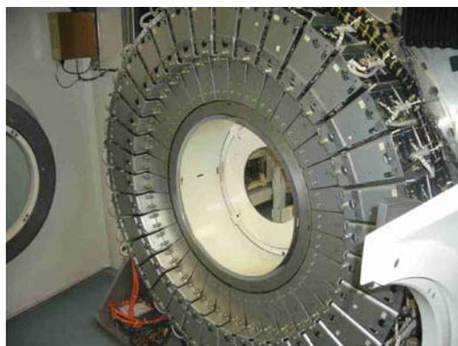
FIG. 2. The ECAD 'EXACT3D' PET camera consisting of 48 rings of BGO detector elements.
