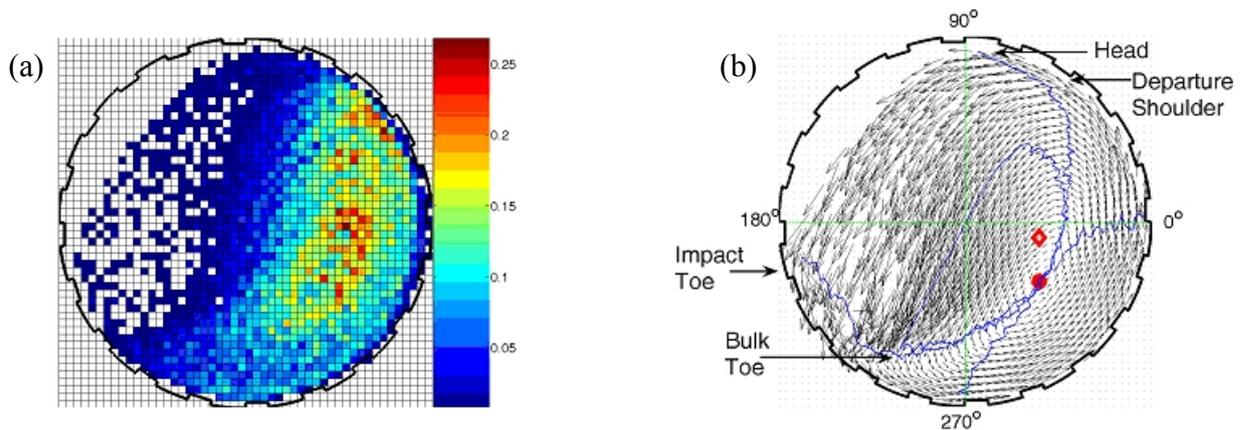
FIG. 5. (a) Percentage occupancy of a 2 mm rock particle for the mill rotating at 75% of critical speed. (b) Distribution of average velocity of the 2 mm rock particle. The three flow equilibrium surfaces (blue lines, see text) allow a number of charge features to be identified.
