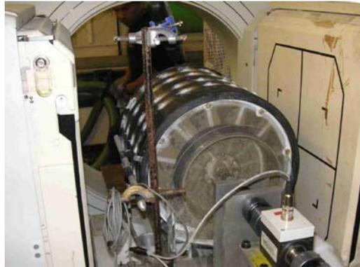
*FIG. 3. The tumbling mill positioned between the two detector heads of the Forte PET camera at the Positron Imaging Centre.*
