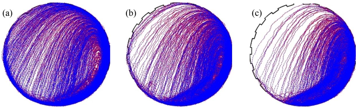
FIG. 4. Front view trajectory fields measured via PEPT for a 2 mm rock particle in a mill charged with a 15% dry load, rotating at (a) 95%, (b) 85% and (c) 75% of critical speed.
