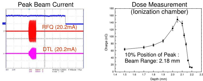
FIG. 3. Beam currents measured at the end of the RFQ and DTL (left), and beam energy measured at the end of DTL-1(right).
