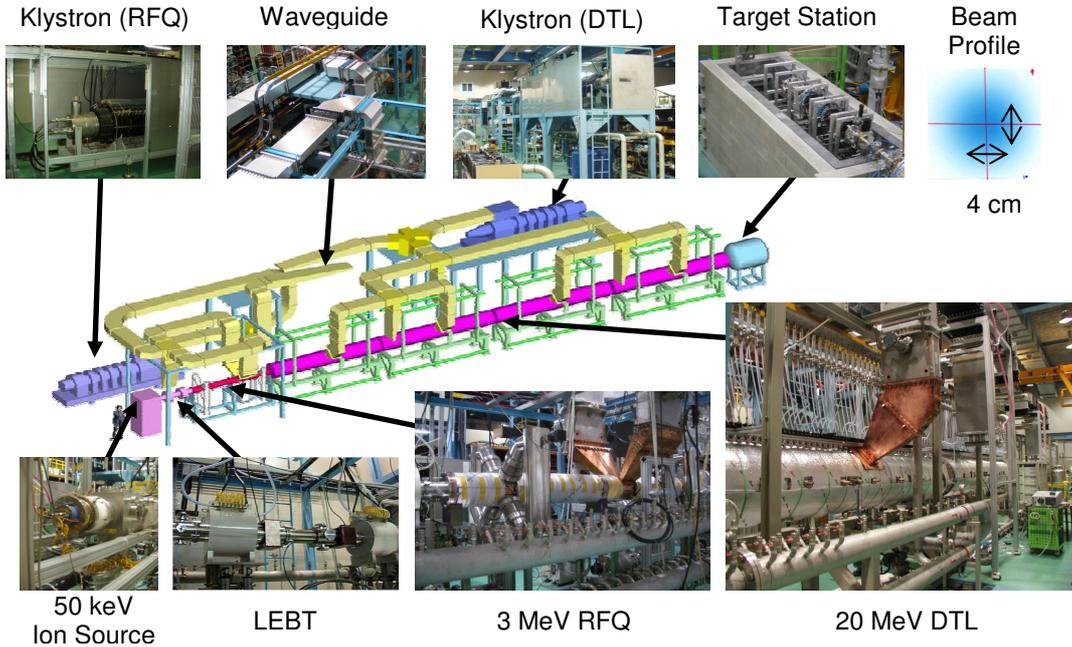
FIG. 2. The PEFP 20 MeV proton accelerator installed at KAERI.
