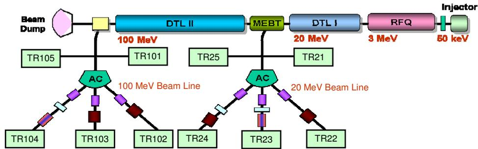
FIG. 1. Schematics of the PEFP 100 MeV linac and beamline facilities.
