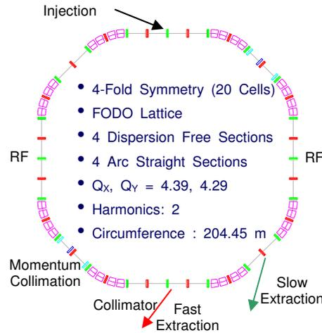
FIG. 7. Conceptual design of the proposed RCS.
