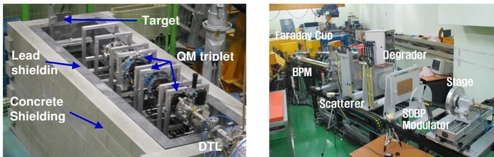
FIG. 6. The 20 MeV beam facility installed at the PEFP 20 MeV accelerator (left) and the 45 MeV proton beam facility at KIRAMS (right).
