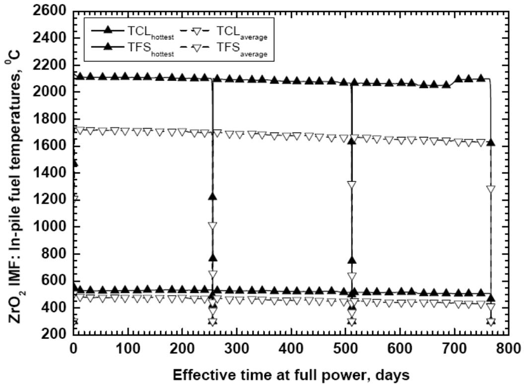
Fig. 1a. In-pile evolution of the fuel centreline (TCL) and the fuel surface (TFS) temperatures in  $ZrO_2$  based IMF.
