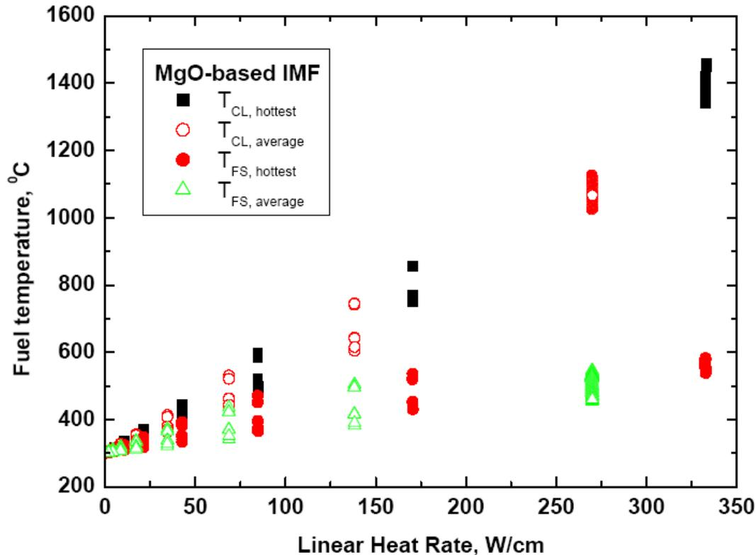
Fig. 2. Centre-line temperature vs Linear Heat Rate in MgO-base IMF.
