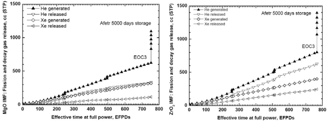
Fig. 4. Fission and decay gas generation and release in inert matrix fuels
