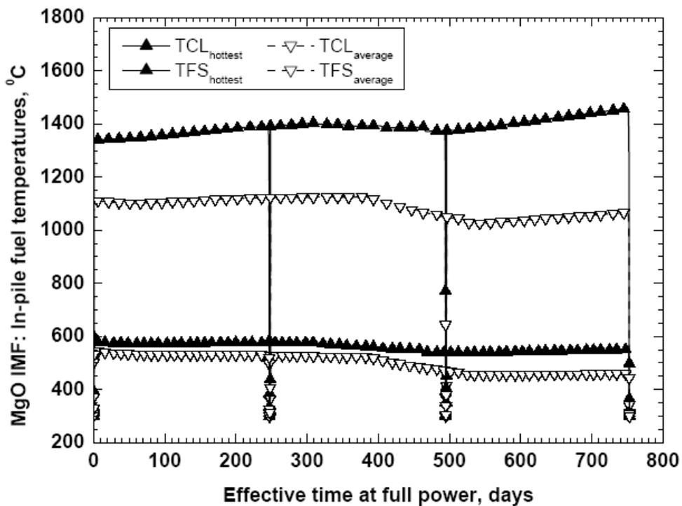
Fig. 1b. In-pile evolution of the fuel centreline (TCL) and the fuel surface (TFS) temperatures in  $MgO$  based IMF.
