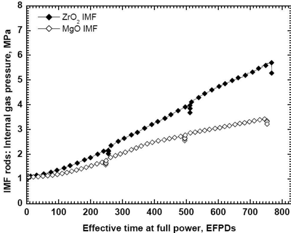
Fig. 6. Inner rod pressure evolution.
