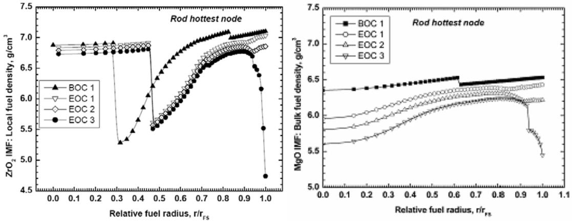
Fig. 3. Radial density profiles and their evolution with irradiation in IMF rods
