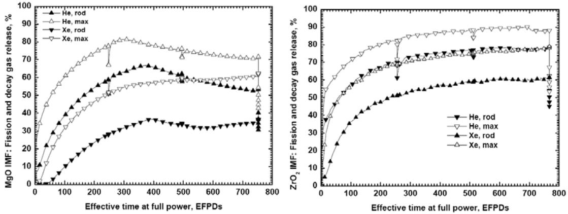
Fig. 5. Fraction of the released fission and decay gases during the operational period.
