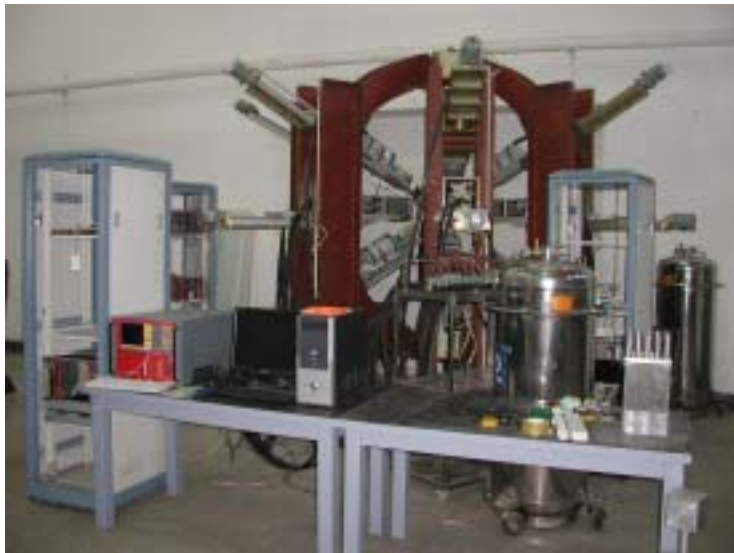
Fig.3 HPGe detectors array in CIAE
