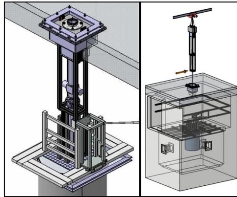
FIG. 5. Vertical beam line inserted into the reactor (left) and retracted to the upper level (right).
