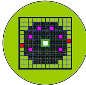
FIG. 1. Cross section of a sub-critical core configuration (SC1, 84 FA), including safety rods (pink), control rods (red) and accelerator insertion channel (central zone).
