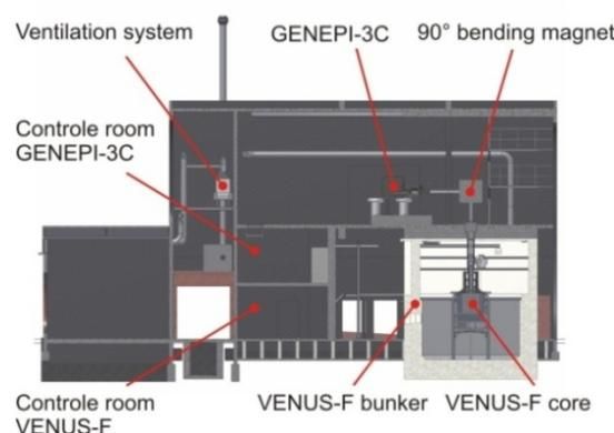
FIG. 2. Side view of the modified VENUS facility
