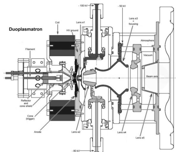
FIG. 4. Duoplasmatron source, extraction and focusing electrodes. High voltages are expressed with respect to the HV ground labelled on the figure.
