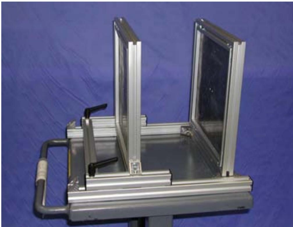
*Figure 4. As-built two-plate collimator.*
