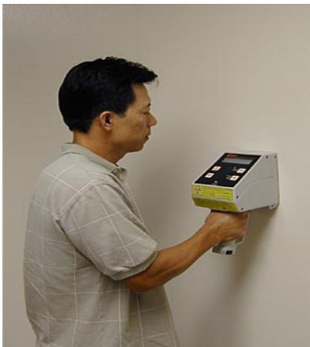
In 1995 in Georgia applicants of the given project had been developed, tested and introduced into customs department of the country portable neutron search detector explosive
