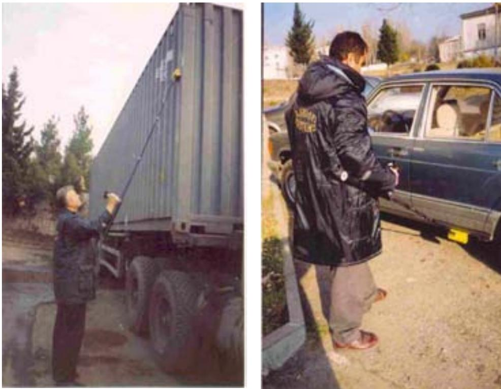
A working surface of a sensor control of the device made 6,0x10,0 cm, and the weight did not exceed 350 g. Application of the telescopic handle of the device provided radiating safety of the operator.
