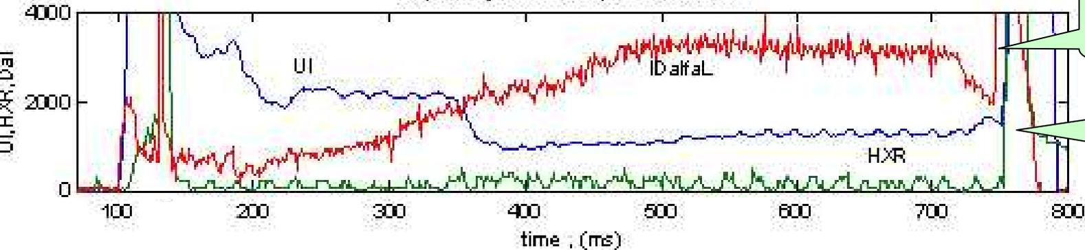
Standard hard x-ray burst are observed 5ms AFTER the energy quench during runaway interaction with the “wall”
