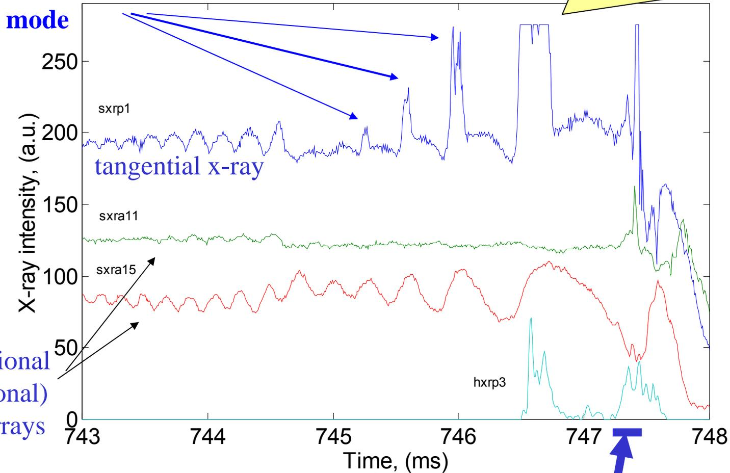
Standard x-ray burst during energy quench is observed with all x-ray arrays
