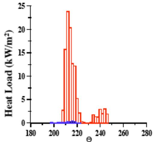
Fig. 1 Poloidal distribution of the heat load in the standard operation. Red histogram corresponds to banana particle loss and blue one shows locally trapped  $\alpha$  loss [2].
