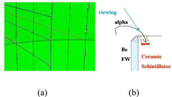
Fig. 3 (a) The area viewed by the camera at the upper port 11. Extra holes on the slit of the first wall panels will be used for installation of various lost alpha probes.
