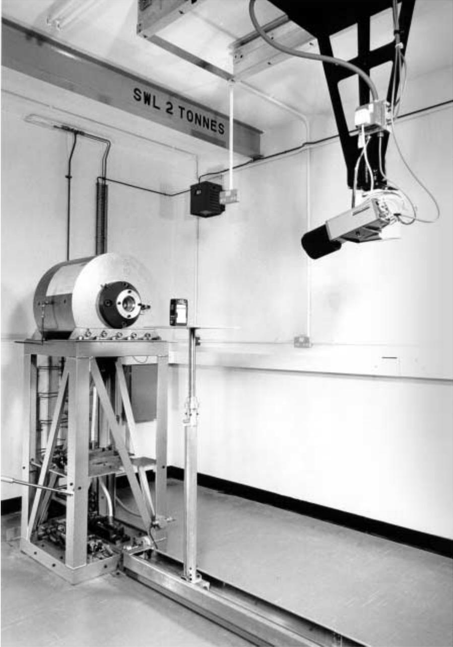
*FIG. 17. Example of a collimated gamma irradiation facility.*
