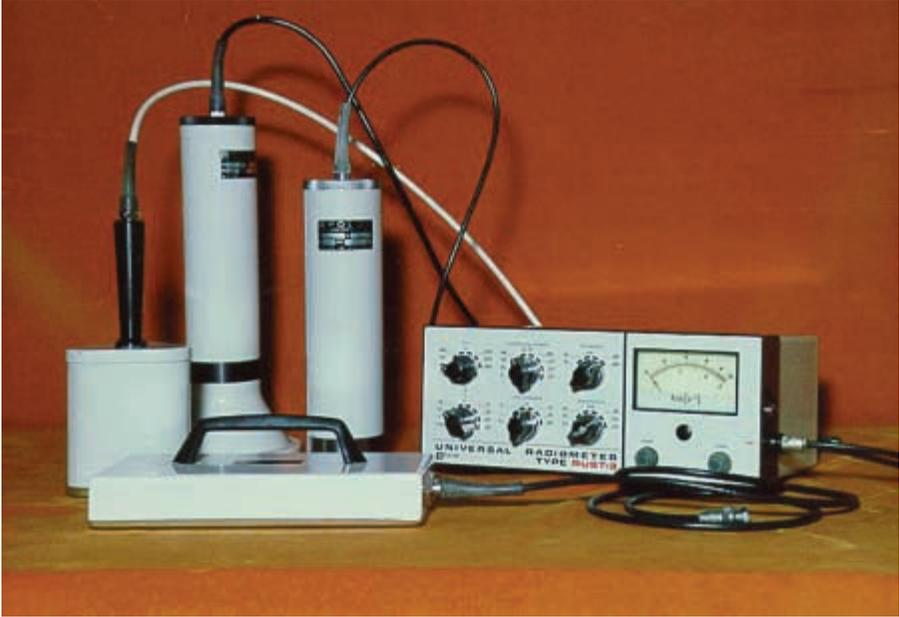
*FIG. 33. Surface contamination meter with various detectors.*
