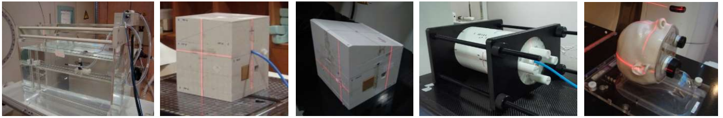
Fig. 1. The phantoms used in DAs: Water, polystyrene (cube and oblique options), CIRS head and neck phantom and RTSafe pseudo-patient head phantom
