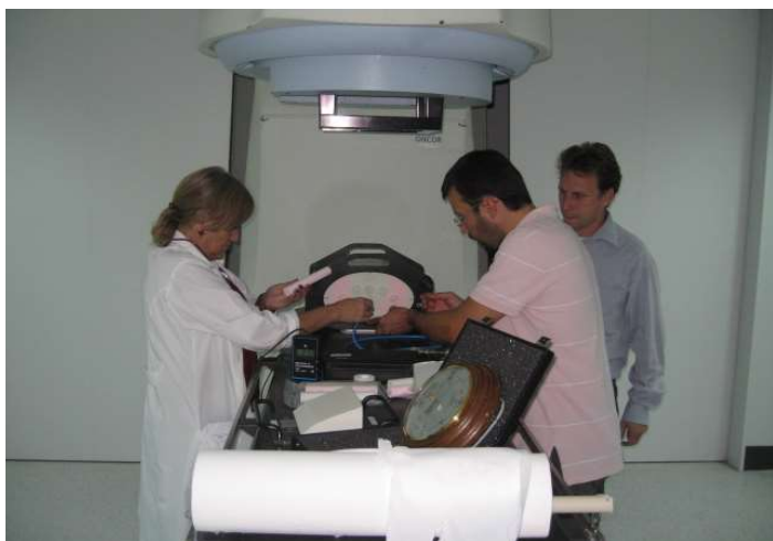
Fig. 1. Medical physicists positioning the CIRS thorax phantom during the “end-to-end” TPS dosimetry audit.
