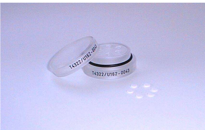
Fig. 1. TLD discs and the irradiation holder.
