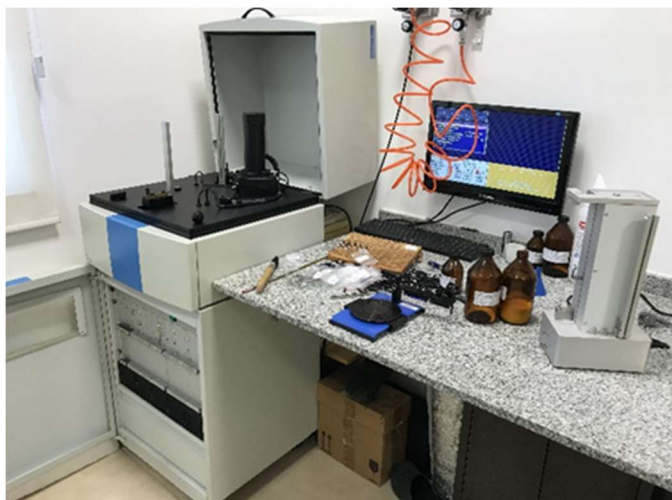
Fig. 1. The TLD system used for dosimetry audits in Argentina.
