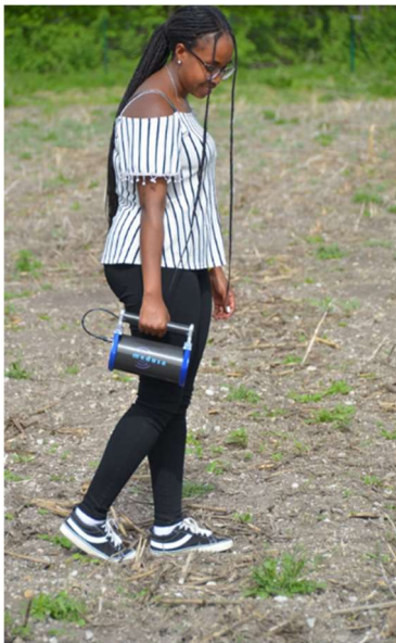
FIG.2. Gamma Ray Spectrometry field measurement in Petzenkirchen, Austria.
