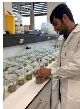
Photo 3. Gas sampling with syringe and transferring to exetainer.
