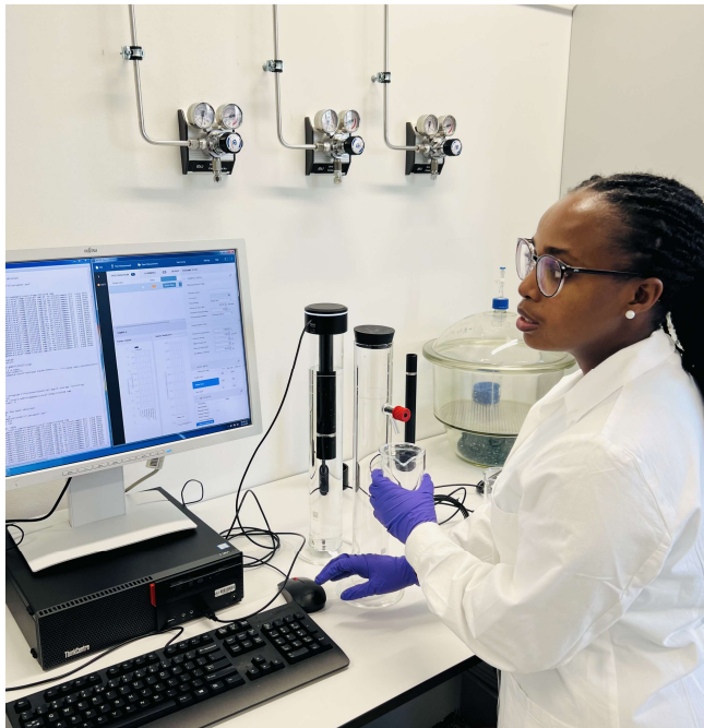
Photo 1 (above). Particle size distribution analysis with the integral suspension pressure method (ISP).
