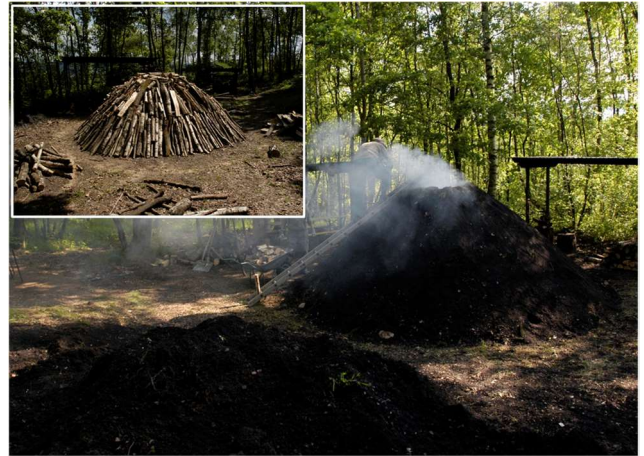
Fig. 6. A typical kiln as it was probably operated for many centuries in the Siegerländer Hauberg and in a very similar way also in the Amazon (© Institut für Pflanzenökologie)
