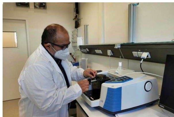
Figure 1. MIR spectroscopy measurement of soil samples
