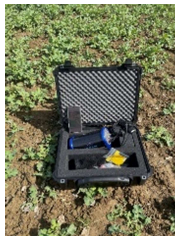
Figure 1. Gamma-ray sensor model MS 350 in Petzenkirchen, Austria.
