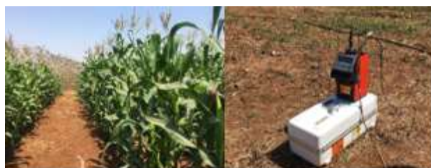
Figure 1. Experimental field with maize, and Neutron probe for soil moisture monitoring
