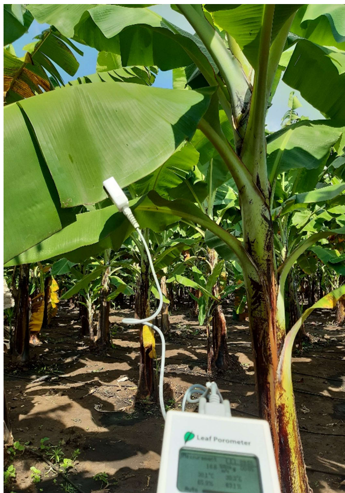
Figure 1. Stomatal conductance measurement of a banana leaf with a porometer (Decagon SC-1).
