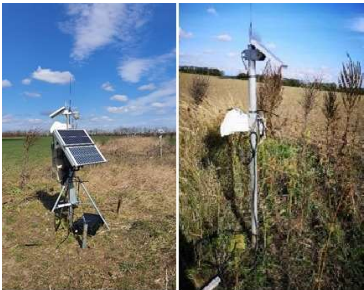
Figure 1. Cosmic ray neutron sensor and drill & drop capacitance probe installed in Rutzendorf, Austria.
