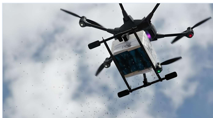
A drone that was designed under the IAEA coordinated research project and tested in pilot projects for aerial releases of sterile mosquitoes (Photo: Moscamed Brasil).
