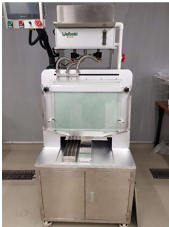
The automatic mosquito pupae sex sorter for Aedes mosquitoes.
