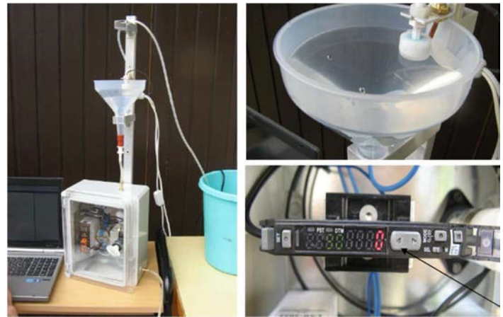
The automated mosquito larval counter. The left panel shows a general view of the larval counter, the top right a detailed view of the larvae dispenser and the bottom right the digital display of the larvae counts.
