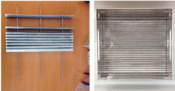
New filter device allowing larvae / pupae separation. Left, details of V shaped filter units. Right, overview.
