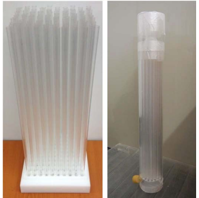
Various systems developed to measure mosquito flight ability. Top, aspirator device used to impose an aspiration stress exposure to mosquitoes; bottom left, 40 cm high flight organ device used to test the quality of adults emerging from pupae; bottom right, flight organ device used to test the quality directly of adults.
