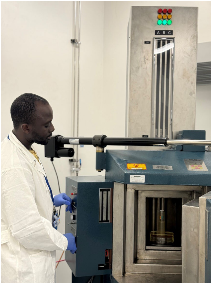
Mr Bénéwendé Aristide Kabore setting up the model 812 irradiator to expose the pupae.
